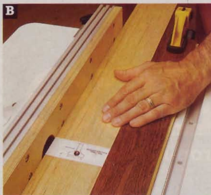
Put the bit through the side panel's start hole, and turn on the router. Move the panel to the stop hole, switch off the router, and remove the panel.
