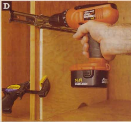
D To easily and accurately position the drawer slides, clamp an 1 1/4"-wide plywood spacer to the carcass.
