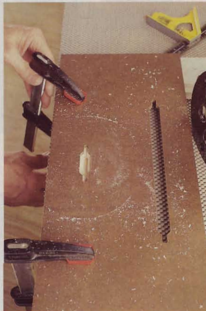
4 Remove the template After finishing the cut, turn the router off and back it completely out of the cut. If you're going to hang the piece from two fasteners, mark the other slot and repeat the process.
