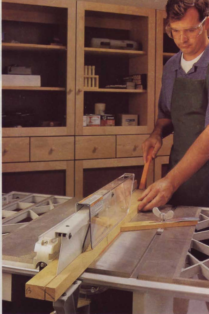
This is the way to play defense against tablesaw kickback. Stand at the outside edge of the board, use a proper pushstick and featherboard, and keep your splitter and anti-kickback pawls in place.
