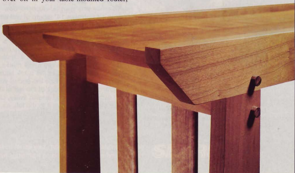
To avoid chipping, extend the straight-edge past the leg's end. Begin routing at the wider bottom portion, and move toward the narrower top.
