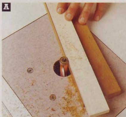
To avoid chipping, extend the straight-edge past the leg's end. Begin routing at the wider bottom portion, and move toward the narrower top.
