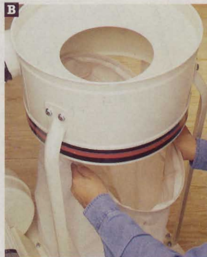
Rather than a traditional bag clamp, the Jet DC-1100 has a spring-steel hoop stitched into the bag's mouth for effortless bag removal and reinstallation.
