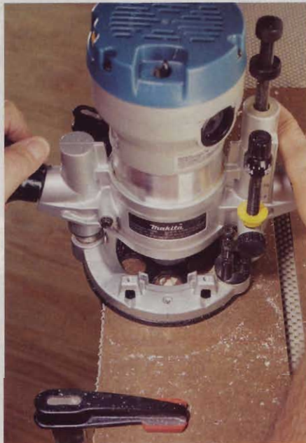
3 Rout the slot With the guide bushing at the bottom of the slot (as the workpiece will hang) and the router on, plunge the bit into the workpiece. Guide it to the other end, backing the bit out frequently to clear dust.
