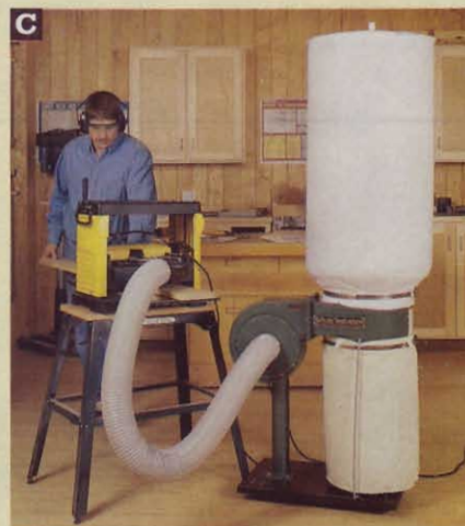
The optimized bag set for the Grizzly G8027 performed better—even with the storage bag full—than the factory bags did when empty.
