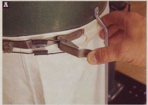
The release lever on the Grizzly G8027's bag clamp bent easily when closing it. Since our test, a Grizzly spokesman told us they would improve the clamps.
