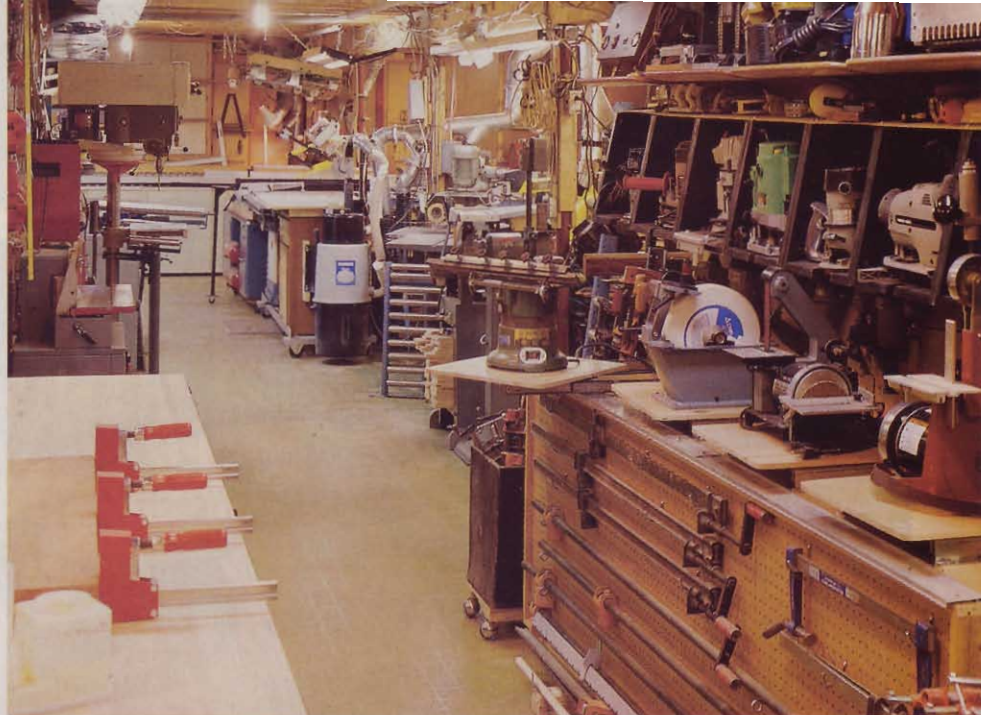
Even in a shop this big, every inch of space counts. These slide-out, rotating platforms allow benchtop tools to be pulled out when in use and tucked away when not needed.
