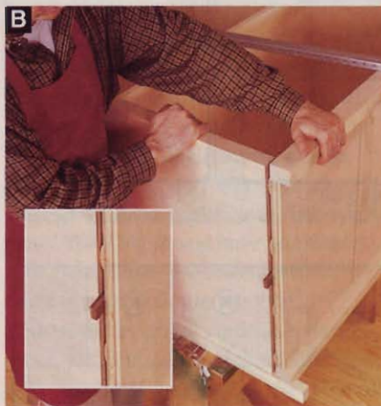
B When popping the top in place, a short block of wood, inset photo, helps to lever the sides apart.
