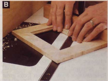
Rout the corner tab recesses, making multiple passes until the frame's corners ride against the fence.
