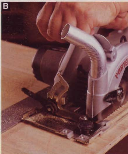
B This dust-deflecting tube on the Porter-Cable circular saw rotates about 270° to redirect dust away from the operator.
