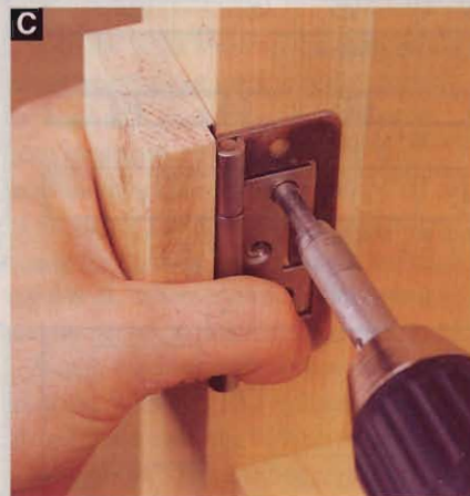
C The hinge knuckles protrude ⅛" beyond the legs. A simple scrapwood guide ensures accurate positioning.
