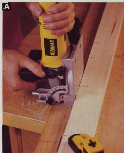
Clamping a straightedge to the back (D) creates a fence for positioning the biscuit joiner when cutting the biscuit slots along its bottom and right side.
