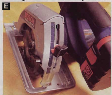
E Clear markings and good location make Bosch's depth scale the best in the test. The door on top of the blade guard opens to accept a dust-collection hose.
