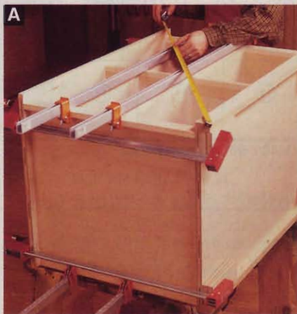
A When assembling the carcass's drawer recesses, measure the diagonals. Equal dimensions indicate a square assembly.
