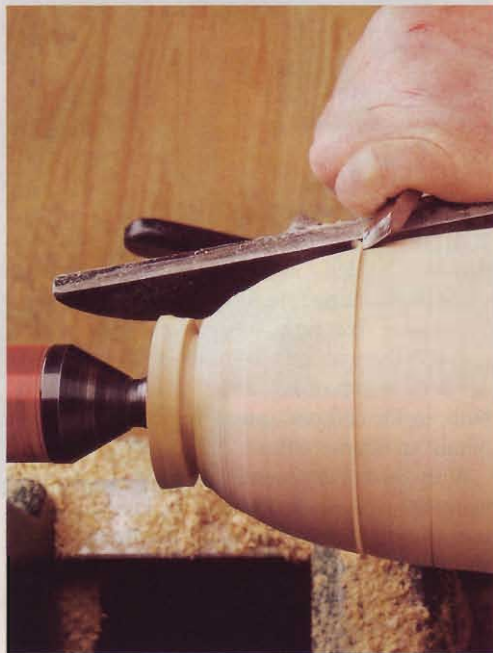
TOOLS: Bowl gouge, roundnose scraper. TOOL REST: Above center. SPEED: 800-1,200 rpm.
