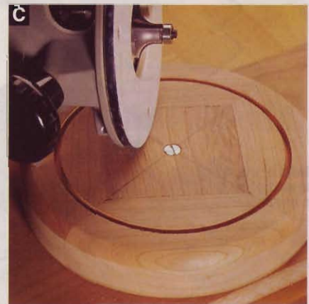
Mount a cove and bead bit in your router, and set it so that it rounds over the edge without cutting a shoulder.
