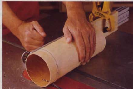
Move the tube over the saw blade, then rotate it against the auxiliary fence and stop for an even 360° cut.
