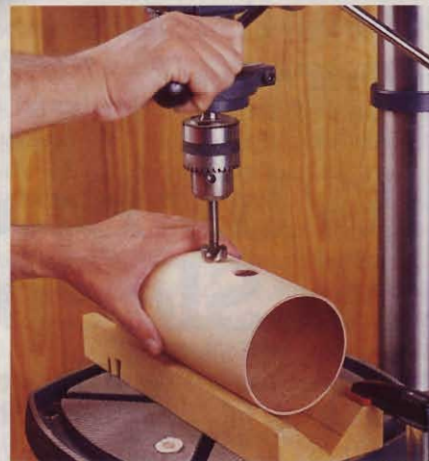
Use your drill press and a Forstner bit when making holes in Hollowood, easing the bit slowly into the wood to avoid tear-out.
