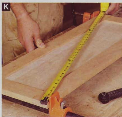
K Before the glue sets, measure across the diagonals of each door. Equal measurements mean the corners are square.
