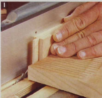
I A feather board adds a lot to your accuracy when you're cutting grooves on the edges of the door rails and stiles.
