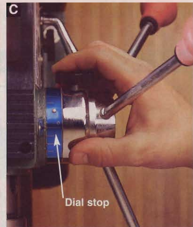
The stop nut of a three-nut system (Photo A) sets the drilling depth, the jam nut locks the stop nut in place, and the quill-lock nut fixes the quill's upward travel. Delta's stop system (Photo B) employs a quick-set stop nut and separate ratcheting-lever quill lock. In our tests, the models with dial stops on the quill-feed hub (Photo C) were easy to use but unreliable over the long haul.
