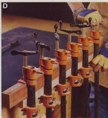
A caul of scrap wood ensures even clamp pressure on the laminate adhered to the wood edging.
