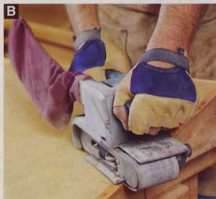
B A belt sander removes the excess from the wood edging, making it flush with the medium-density fiberboard (MDF).
