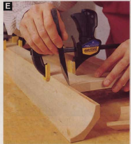
Want to know how pros get nearly invisible miters? Just use a sharp knife to transfer the cove molding cutline from the top assembly.
