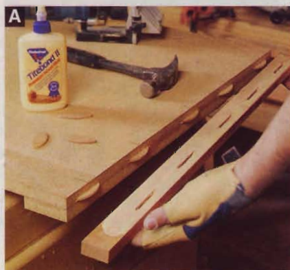
A Shimming up the biscuit joiner to cut the underlayment raises the slots \frac{1}{32} ". This, in turn, raises the edging, allowing you to flush-sand it with the underlayment.
