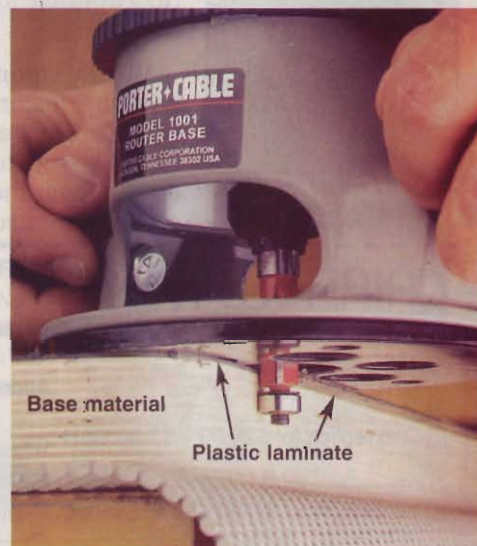
Keep the bearing in light contact with the base material when routing. Too much pressure can mar the workpiece.
