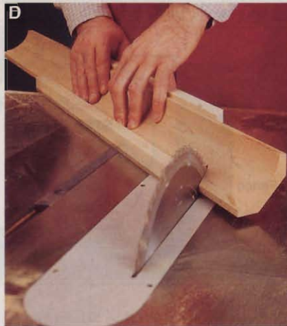
The jig cradles the cove molding, preventing it from rocking while you make the miter cuts. Screw the jig to your table saw's miter gauge.
