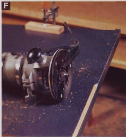
F To expose the cherry in the edging, cut the reveal with a 45° chamfer bit chucked into a handheld router.
