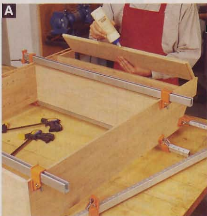
A To fasten part C, apply glue to the rabbets and also along the upper edge of part C. Clamp against the lower shelf.
