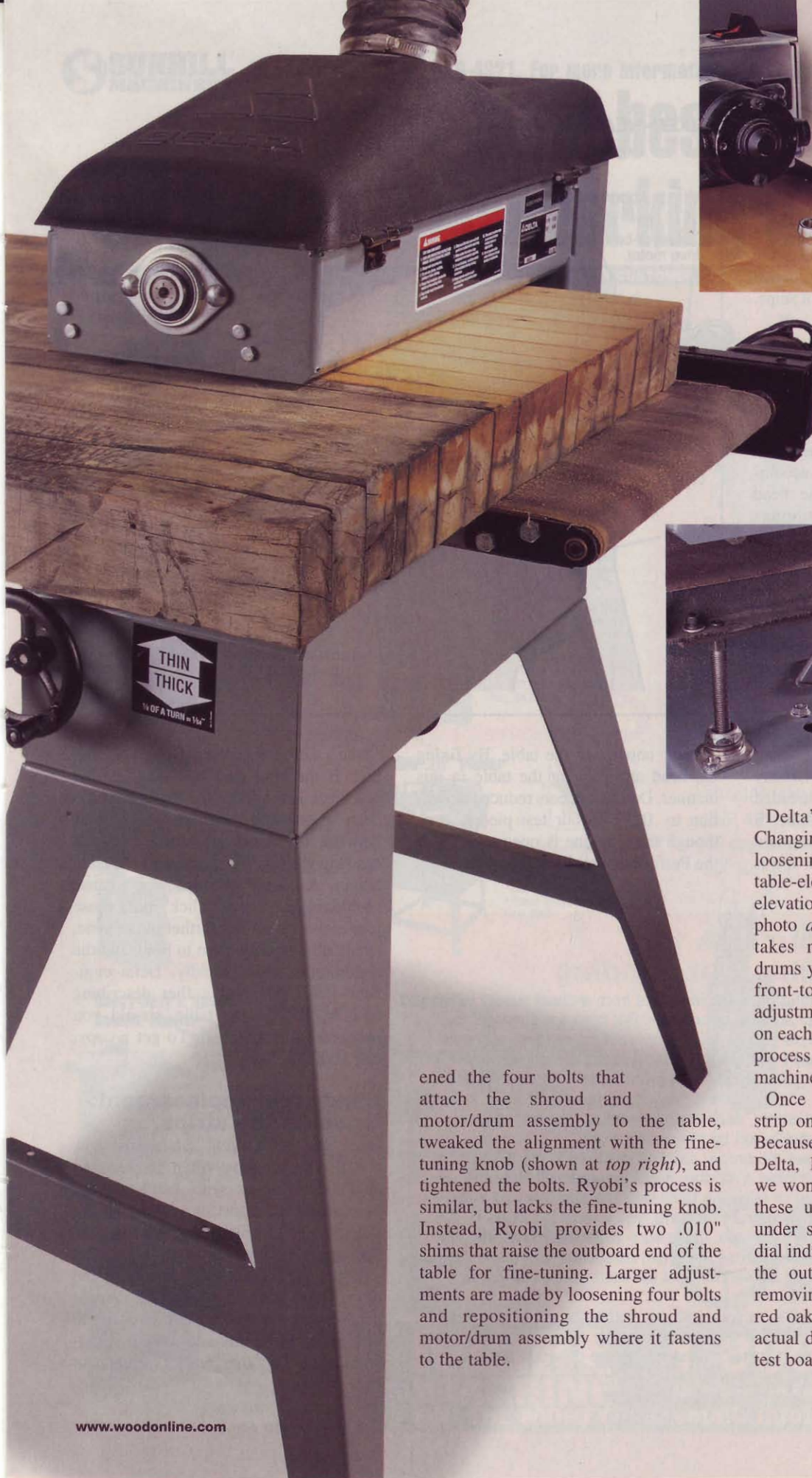
The fine-tune adjustment knob on the Performax 16-32 PLUS, above, allowed us to dial-in precise head-to-table alignment.
