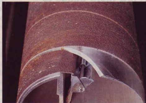
LEFT: Performax's "TUF Tool" activates the tough-to-get-to spring clip on the inboard end of the drum to prevent finger-pinching while loading abrasive. RIGHT: The cutout on Delta's drum means you don't have to blindly feel for the take-up clip. However, it tended to pinch our fingers against the sharp edge as we released the clip.
