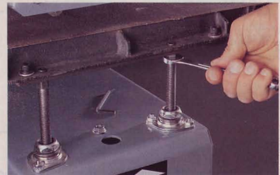
To make Delta's table, below, parallel to its drum, turn the outboard elevation screws an equal number of turns, then lock them in place with setscrews.
