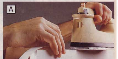
A Apply the front banding edge last. That way, the joint between the front and bottom banding isn't visible from the front.
