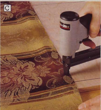
Stop your staples 2" from the end of the ½" plywood cushion panel when tacking the fabric in place.
