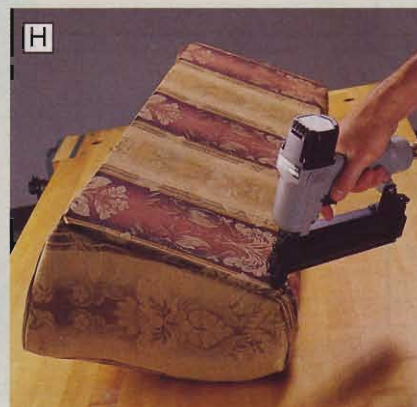
H Brads hold the upholstered back panel to the upholstered cushion panel. The brad heads disappear below the fabric.
