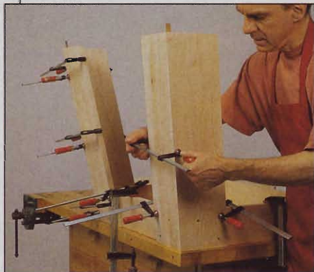
Clamping the legs (D) to the frame (A/B/C) holds them at the proper angle while you finish clamping their length.
