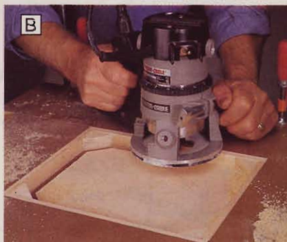
B With the guide bearing of the pattern bit riding on the spacer strips and triangles, cut out the opening.
