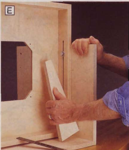
E Working from the rear, square the table to the base, and position the braces.
