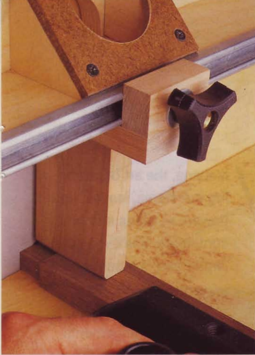
Slide the hold-down block into the fence channel, and center it whenever you need to keep a narrow piece in place.
