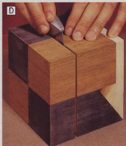
Carefully slice through the last \frac{1}{32} " by cutting down the center of the saw kerf with a utility knife.
