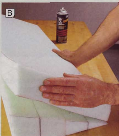
Align and adhere the front piece of the seat back to the glued-up rear pieces.
