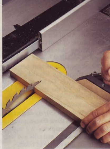
You can use the sliding aluminum fence faces of the Delta 36-475 and DeWalt DW746X (shown) as a crosscut stop without trapping the workpiece.
