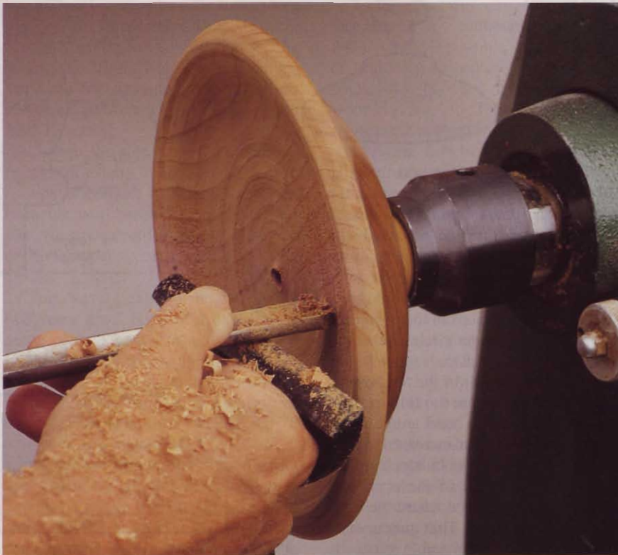
Remount the bowl on the screw chuck to turn the inside. Take light cuts with a sharp gouge to prevent knocking the workpiece off the chuck.
