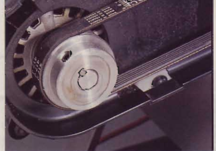
The Ridgid TS2424's machined steel pulleys and flat, ribbed drive belt made it one of the smoothest operators in our test.
