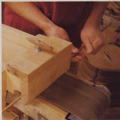
To make his own dowels, Jim invented a simple jig that mounts to his stationary belt sander. Pressure from the adjustable wooden platen holds the wood against the belt as he turns it with his fingers.
