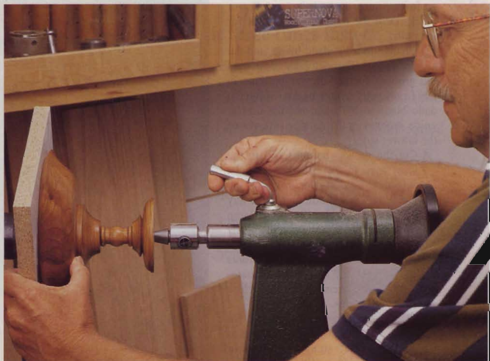
Glue the bowl, stem, and base together, and clamp them to complete the project. For a clamp, you can't beat the lathe.
