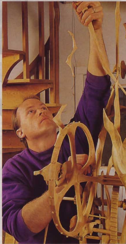
Much like decorating a Christmas tree, Jim hangs sculpted bits of wood to a clock in progress to properly balance it.
