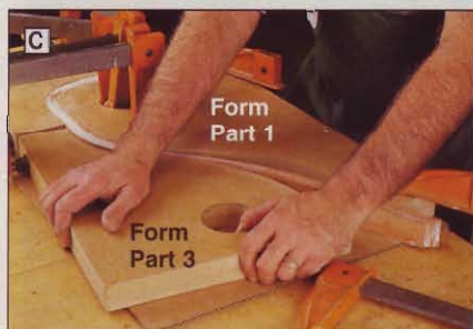
Use arm force to bend the laminations and draw form part 3 into position so you can clamp it to form part 1.
