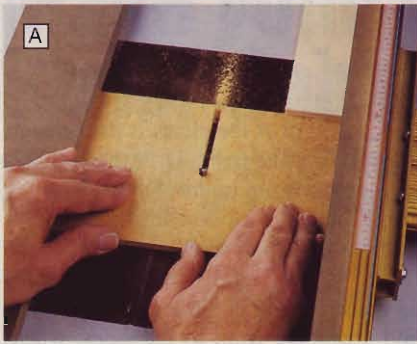
A Center the bit between two fences that capture the dividers. A stopblock controls the length of the slot.
