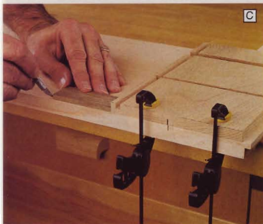
Use a craft or utility knife to mark the location of the top of the next dado in the carcass side.
