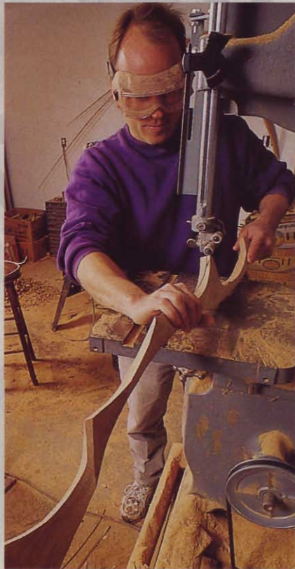
At his bandsaw, Jim freehands stock through the blade to rough-shape a new pendulum for a clock.
