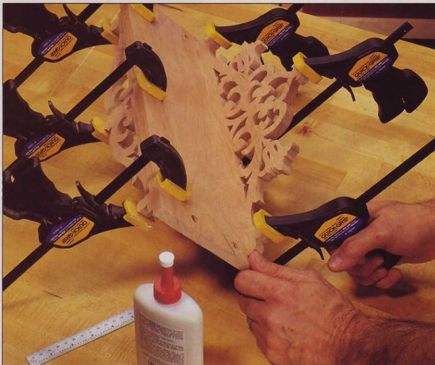
Space the top trim \frac{1}{4} " from the back edge of the top, and position the top apron \frac{1}{2} " from the front edge of the top.
