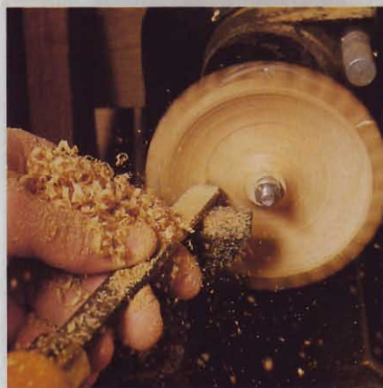
Shaping the gear wheels' faces adds to the sculptural effect of the clocks.
