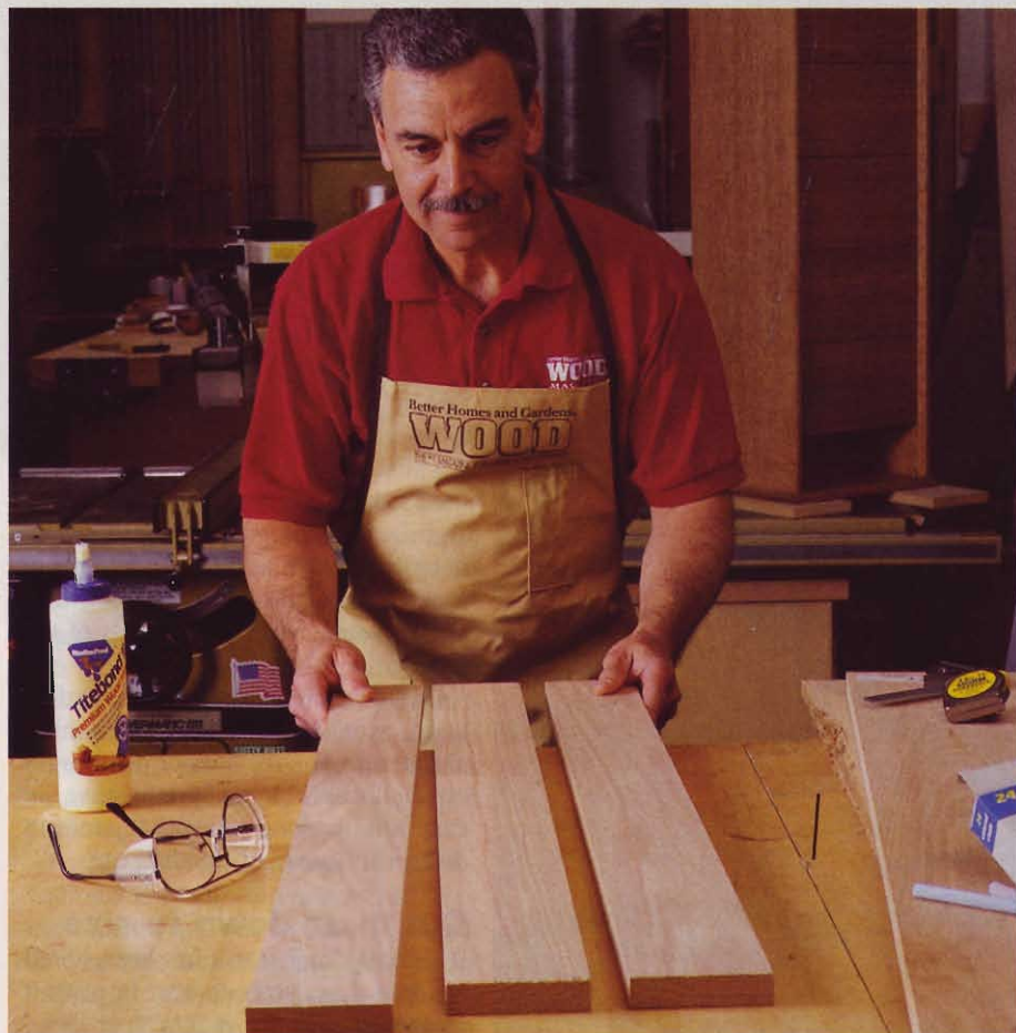
After cutting your stock to size, lay the boards on your workbench and begin looking for the perfect match, as WOOD magazine's contributing craftsman Jim Heavey does here.
