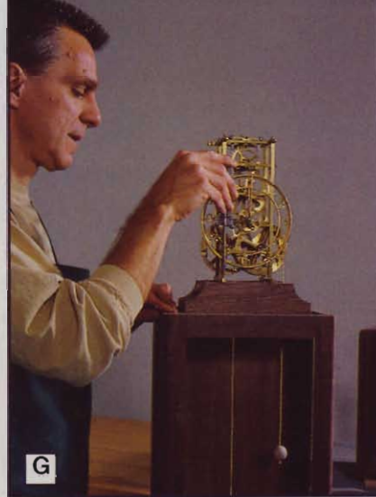
The removable upper case makes mounting and adjusting the movement easy.
