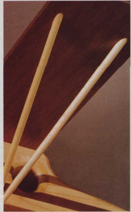
Sand the ends of the wing struts at an angle so they match the wing underside.
