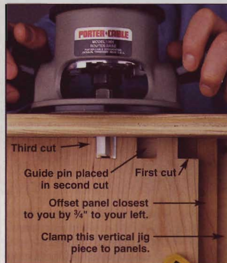
Work from your left to right when cutting the pins and matching holes across the ends of two clamped panels.
