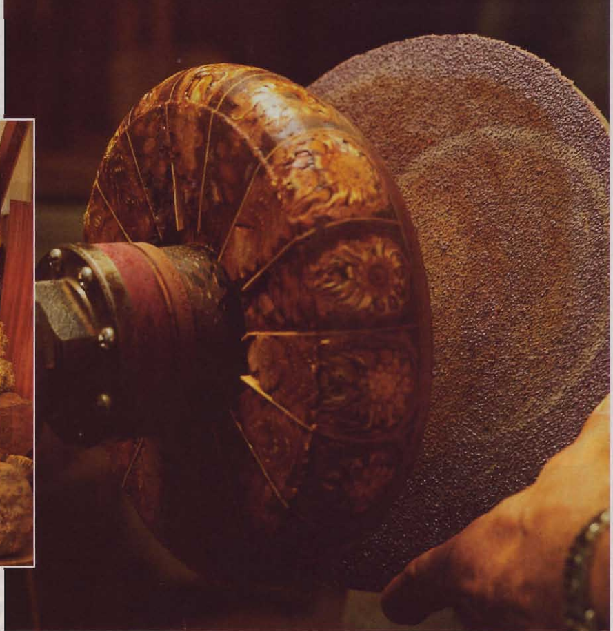
Can you guess what this bowl's made of? Pine cones joined with epoxy! Galen uses a sanding disc fastened to a metal plate to perfectly flatten its bottom.
