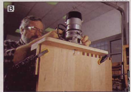
Use the jig to rout the notches in the ends of the back panel.
