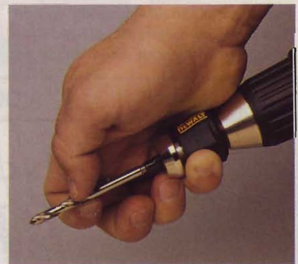
One-handed bit removal on most connectors, such as DeWalt's Rapid Load, is possible, but uncomfortable. The hand-stretching motion required may be difficult for those with limited dexterity.
