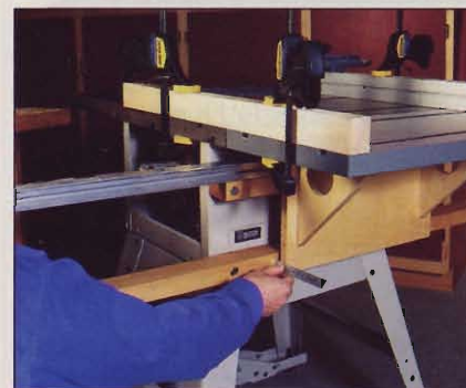
Clamp the sliding table flush with the saw top, and measure for the thickness of the wear blocks and their spacers.
