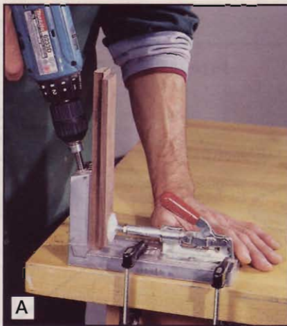
A Use a pocket-hole jig to drill the inside faces of the rabbeted rails.
