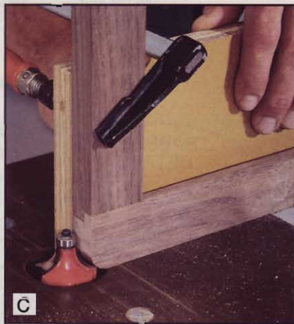
C To prevent tear-out on the trailing faces of the stiles, use an auxiliary fence attached to the miter gauge.
