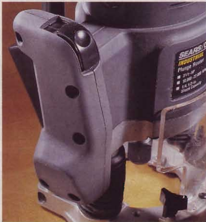
Lock the Craftsman 27511's plunge depth by pulling the handle-mounted trigger. To release the mechanism, simply push the button on top of the handle.
