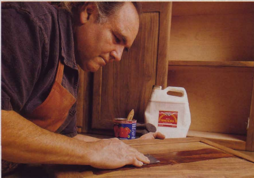
Going beyond label instructions, Victor applies a penetrating, tung-oil sealer with 220-grit wet-dry paper. The top coats of an oil-urethane mix he'll wipe on, then buff with steel wool.
