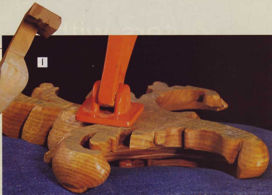
To support a workpiece on an uneven carved face, press it into a sandbag. This one is made from one leg of an old pair of jeans.
