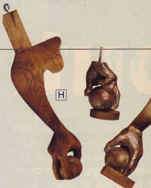
Keith used a life-casting of a hand holding a baseball (center) to mock up a table leg (right) prior to carving a prototype leg (left).
