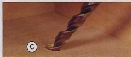
Angle the \frac{5}{16} " hole in the box top so you can pass the carriage bolt through it.
