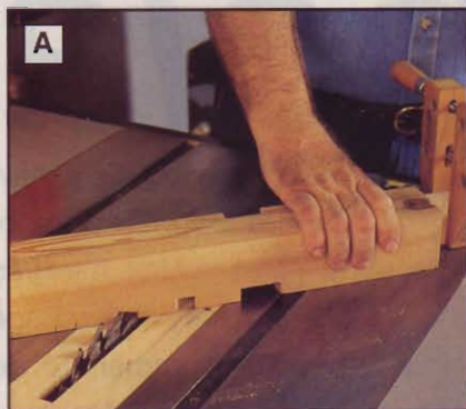
Align the marked dadoes with your dado blade. Use a clamp as a stop on the miter-gauge extension for consistently placed cuts.
