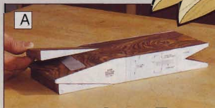
A Tape the sawn-off sides back onto the blank to provide flat surfaces for pattern attachment and sawing.
