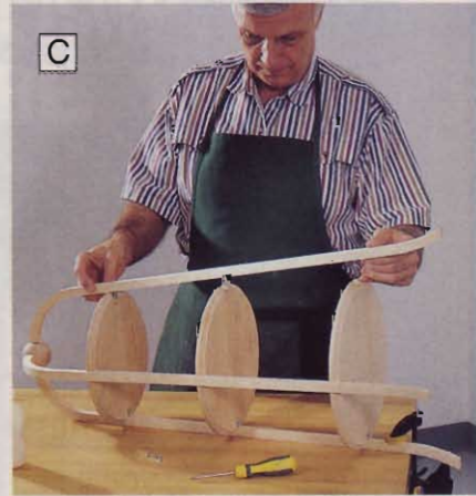
C After gluing the leg to the ball, seat it in the notches in the trays.
