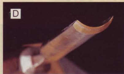
Honing the edge brings it to final sharpness. The line of reflected light is now too narrow to see with the unaided eye, and the tool is sharp.
