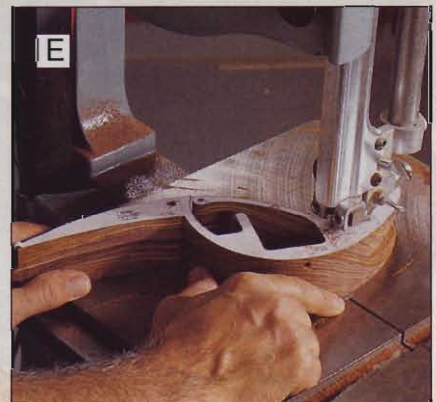
E Make the final cut to free the lid as a smooth continuation of the curve that comes down the top of the tail.
