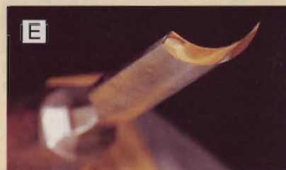
Polishing smooths the bevel for easier cutting and to leave a burnished surface, free of scratches, in the cut.
