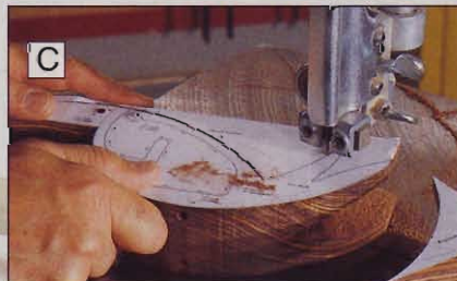
C To saw a sharp corner, cut into it from both directions. Carefully stop each cut at the pattern line.
