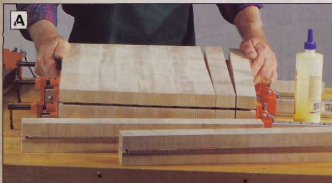
Spread an even coat of glue on all mating surfaces, then glue and clamp the top strips together, keeping the ends flush.
