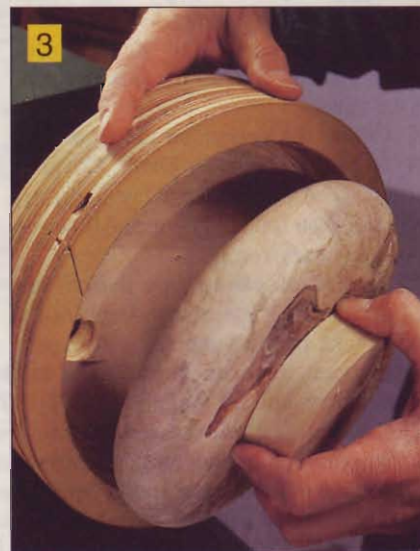
3 Insert the turning into a shop-made jam chuck for parting off the waste block and completing the back of the flask.
