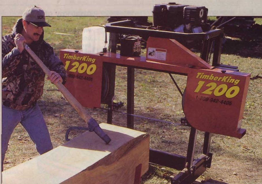
Manually loading logs and turning cants was part of the experience with the TimberKing 1200 and the other two lesser-priced bandsaw mills.
