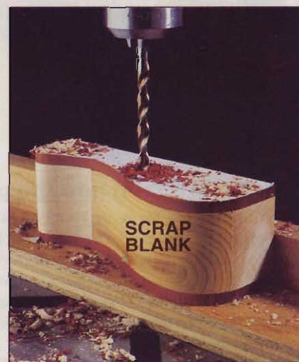
The scrap blank prevents the side stock from tearing out when you drill the \frac{1}{4} " hole for the brass rod.
