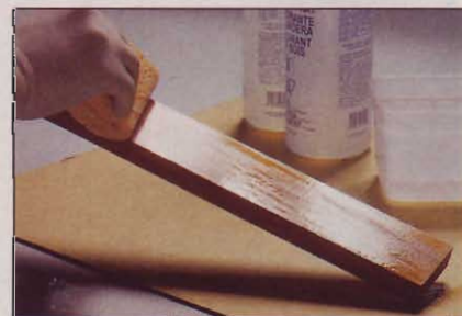
Apply the bleach as evenly as possible, and keep the surface wet as you work.
