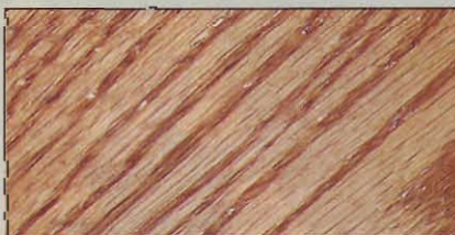
Oil/varnish blends bleed back out of the pores of such woods as red oak. You need to wipe away these tiny puddles before they dry.
