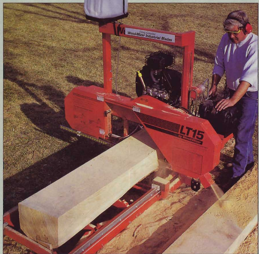
With the Wood-Mizer LT15, as with all bandsaw mills, you must first square the log into a cant before you can saw boards.
