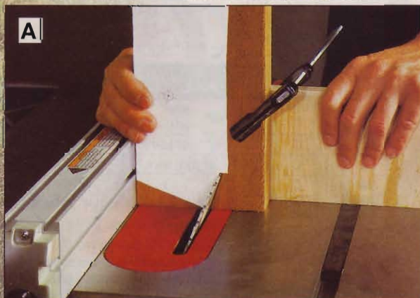
With the pattern adhered to the leg blanks, cut the notched ends first. Note support fence and clamp used.
