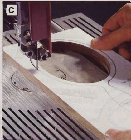
Photo C Bandsaw the mirror to shape after routing the rabbet in the opening.
