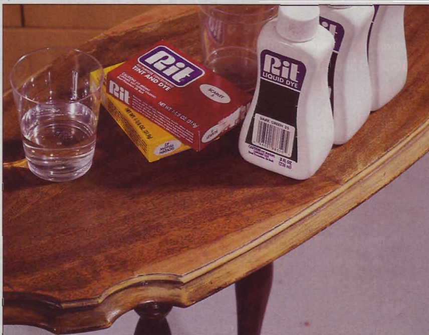
You can color wood with either liquid or powdered dyes. Mix powdered dyes according to package instructions.
