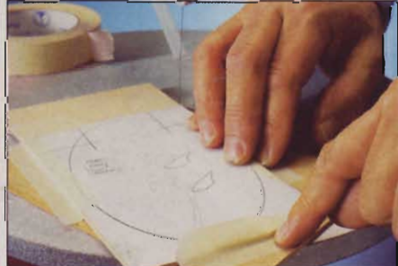
Firmly press the tape into position to prevent the background panel and inlay stock from shifting.
