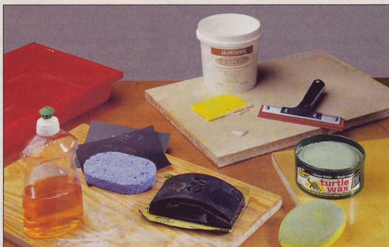
Paste wood filler, top center, makes a smooth foundation for the finish. Wet-sand with a simple solution of liquid detergent and water, left, using a rubber sanding block, bottom center. Polish with an automotive wax, bottom right.
