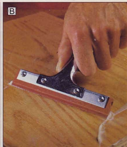
Paste wood filler, top center, makes a smooth foundation for the finish. Wet-sand with a simple solution of liquid detergent and water, left, using a rubber sanding block, bottom center. Polish with an automotive wax, bottom right.
