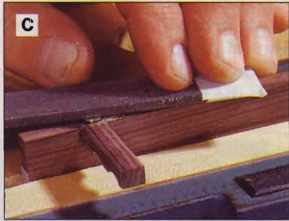
C Tape on the end of the file protects the lid when filing the screws flush.
