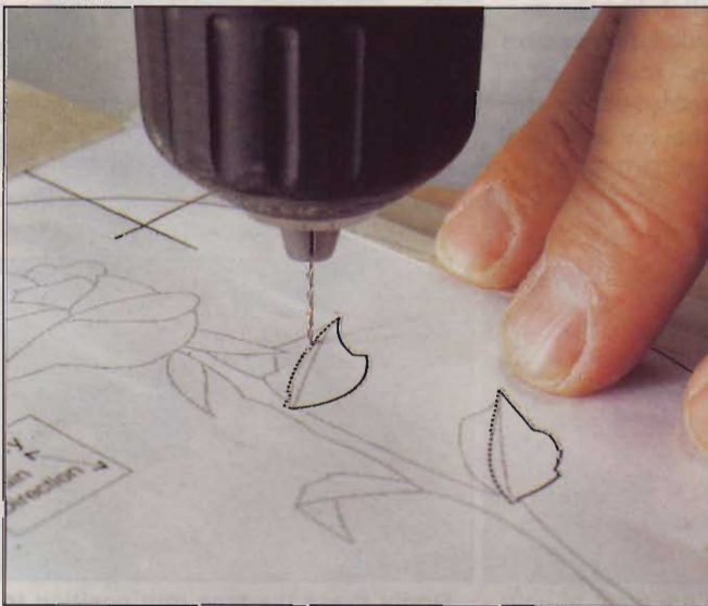
Drill straight down into the dashed areas on the plates to make start holes for your scrollsaw blade.
