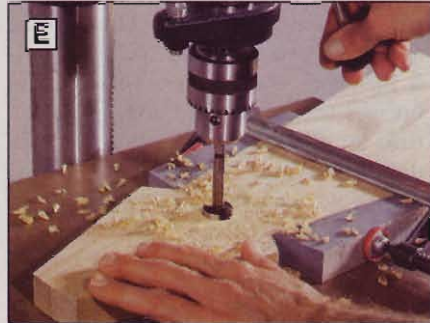
To make the half-round notches for the foot ring, clamp legs back-to-back and drill a 1" hole right on the centerline.
