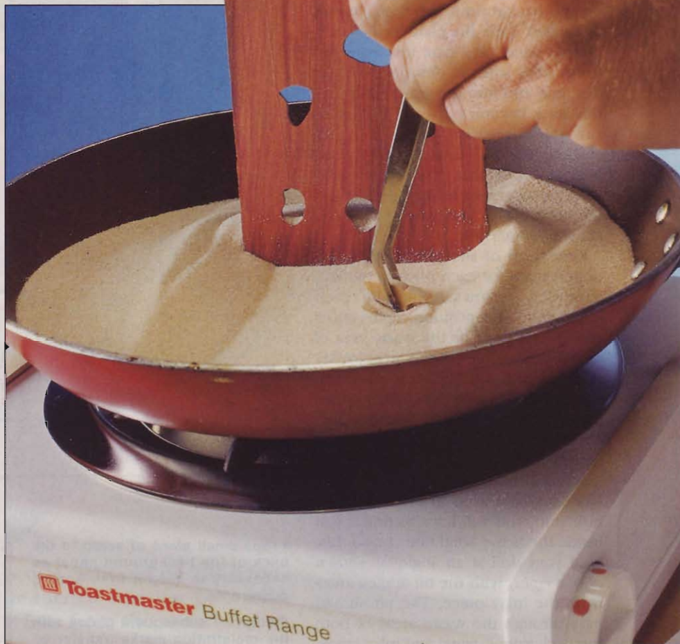
We used a scrap of wood to scrape away the top layer of sand and expose our work-piece to the hotter sand below.
