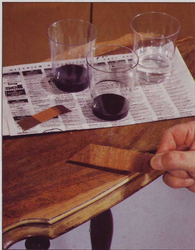
Green dye, applied to the pointed end of the test strip, took away some of the redness in the mahogany veneer, resulting in a close color match. Brown dye proved to be too dark.
