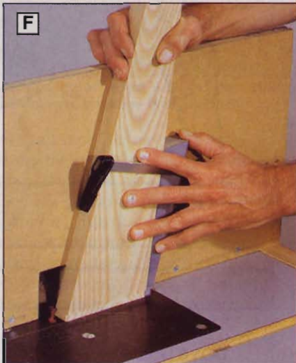
Make test cuts in scrap, then rout the dovetail "tenon" on the top end of each leg. A tall fence and follower block help.
