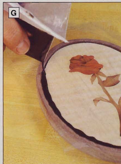
G Borrowing a technique from cake-decorating, squeeze dyed epoxy from a bag into the gap between the back insert and the mirror frame.
