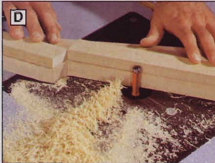
Use tape-adhered guide blocks and a flush-trim bit to rout the first leg to final shape. Then use it as your template.
