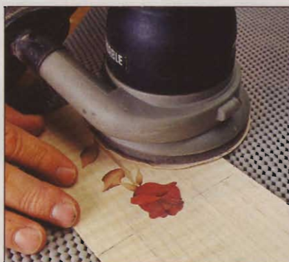
A random-orbit sander and 150-grit disk remove the registration marks and flatten and smooth the workpiece.
