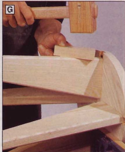
Two of the legs will have to be tapped in toward the center to make clearance for the foot ring, which installs from the top.
