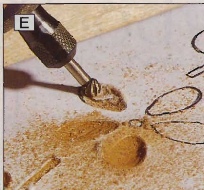
E Carve the floral design about ⅛" deep at the lowest point. You can cut right through the paper pattern.
