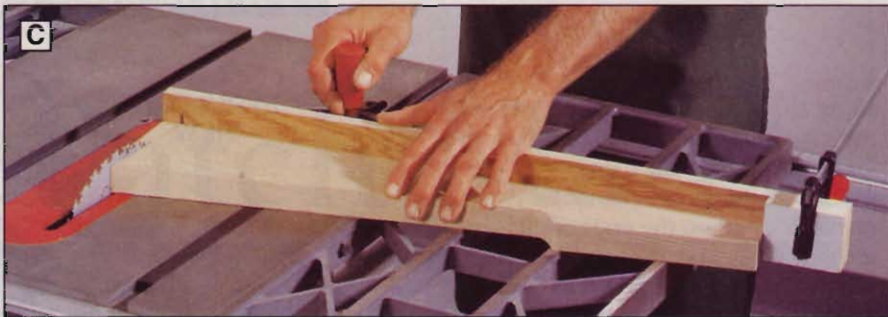
With your miter gauge set at a 6^\circ angle, trim the top of each leg. Then reset the miter gauge to 6^\circ the other direction, reset the stopblock, and cut the bottom ends.
