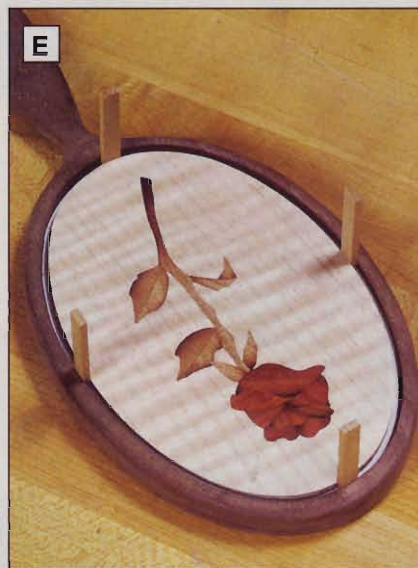
E You can center the back insert in the mirror frame by eye, but four spacers will do the job more accurately. Cardboard or scrapwood will suffice.
