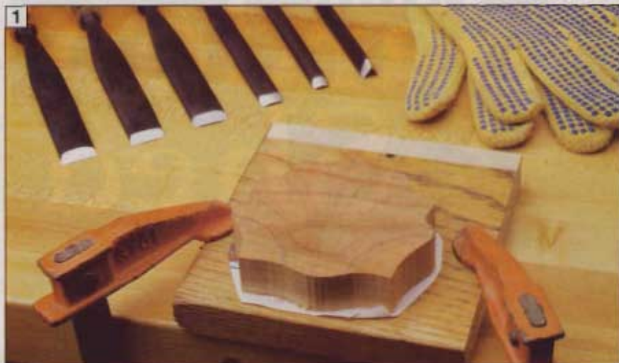
1 Glue the blank to a piece of scrapwood with a paper joint so you can hold it easily for carving. Tools shown are, from left, nos. 3, 4, and 5 gouges (all 20 mm wide), 13 mm no. 6 gouge, 10mm no. 8 gouge, and 10 mm V-tool. The gloves incorporate Kevlar fiber to minimize the chance of cuts.
