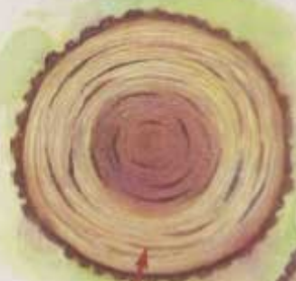
Wind shake causes the wood to separate parallel to the trunk.
