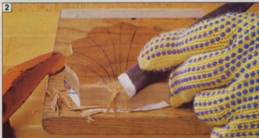
2 After roughing out the curvature with a gouge, you can smooth the contour by carving with the inside of a gouge, such as the 20 mm no. 3 shown. (The wing end of the shell is shown here.)
