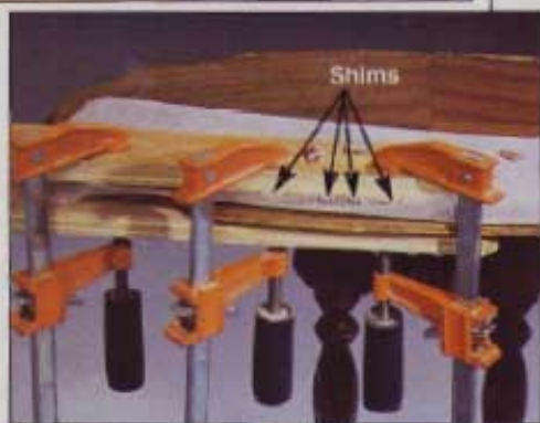
Spread glue between the layers with thin cardboard or plastic. We scraped out the old glue and stuff with the tools on top of the table.
