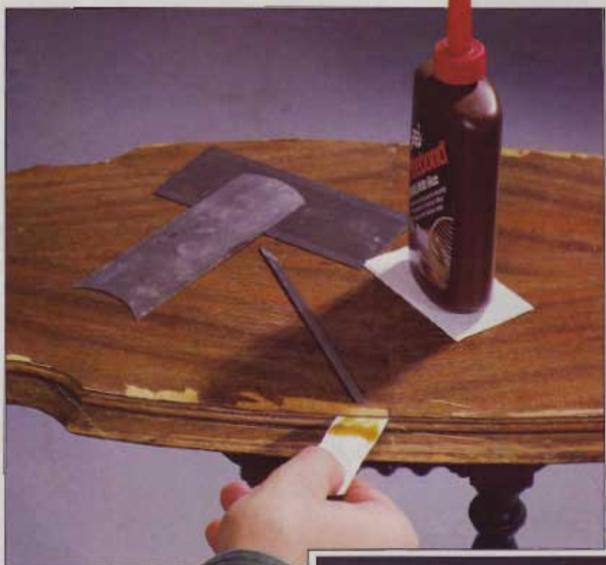
Spread glue between the layers with thin cardboard or plastic. We scraped out the old glue and stuff with the tools on top of the table.
