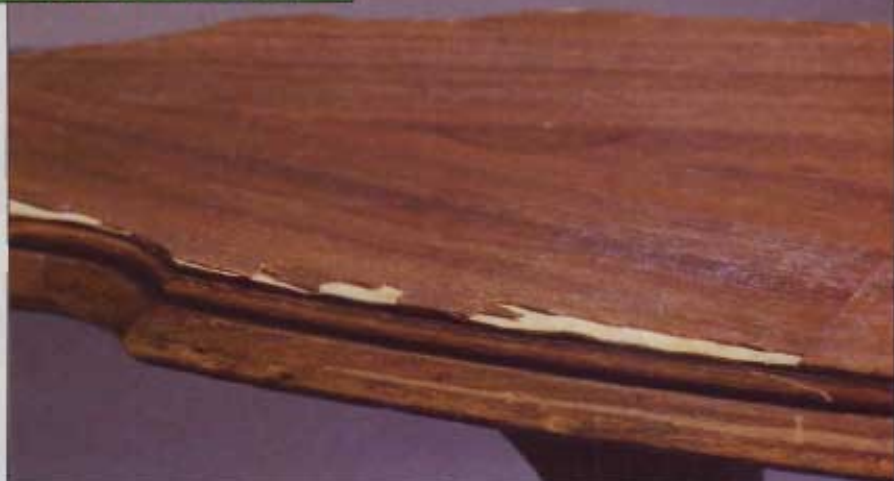
Chipped veneer is only part of the damage to this table edge. The layer between the tabletop and the finish veneer has come unglued, too.
