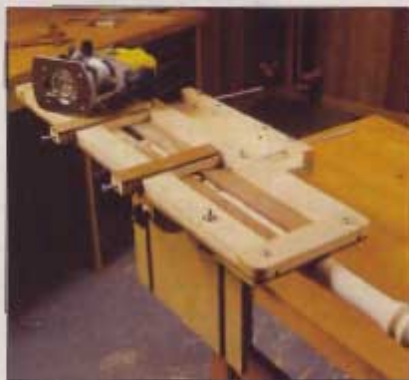
Creating mortises in workpieces goes quickly and precisely with this jig setup.
