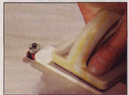
A secured zero-clearance table overlay and pad-style pushblock facilitate routing round-overs on the side panels.
