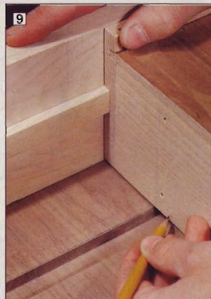
During assembly, turn the tabletop and base upside down and mark the stop locations on the back of the drawer.
