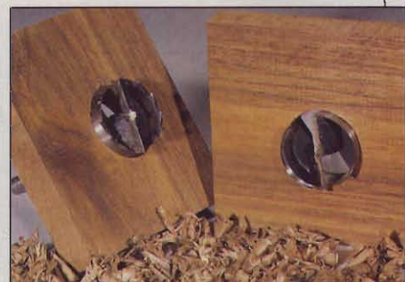
A Forstner bit (right, with the smooth rim) or a multispur bit (left, with the toothed rim) bores a large hole easily.
