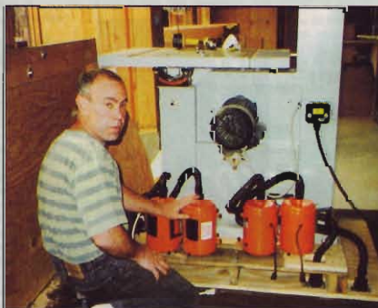
Chuck Pyle displays the four reverse vacuums used to levitate the Laguna Tools' LT24 bandsaw for cutting through timbers.
