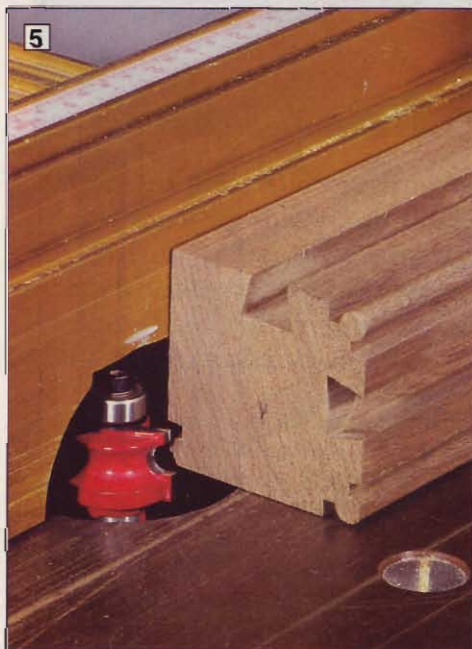
5 Two passes with a \frac{1}{4} " beading bit will cut the detail on the table legs. Check the settings on scrap first.
