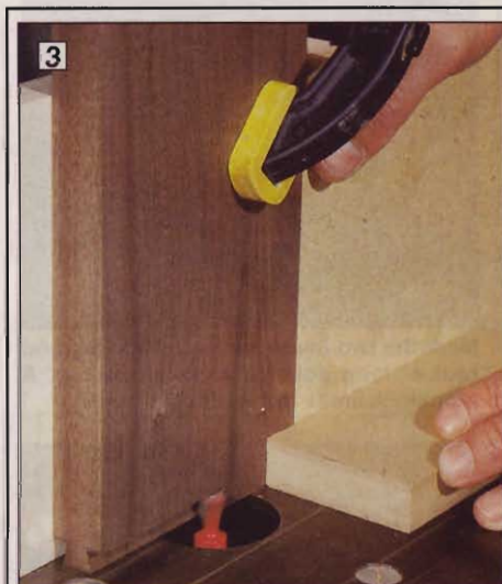
3 Stand the dovetailed rails on end to rout the tenons. Use a tall fence and push blocks for safety and control.
