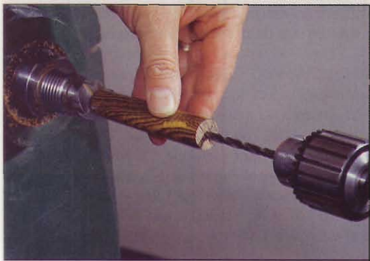
Align the point of the drill on the center mark in the turning. Start with a small drill, and work up to \frac{1}{2} " in steps.
