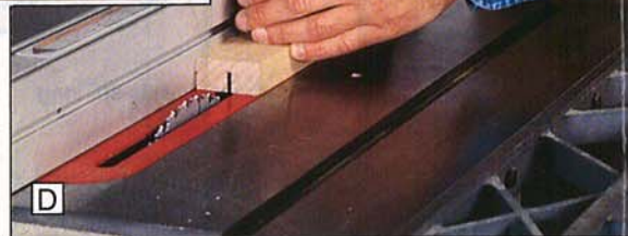
Insert the dowel end into the guide block and align the layout mark with the saw kerf (inset). Cut the kerf; then switch dowel ends and repeat.
