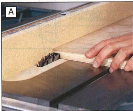
A wood auxiliary fence allows you to use the full width of the 3/4" dado blade to cut rabbets in the plywood carcass panels.
