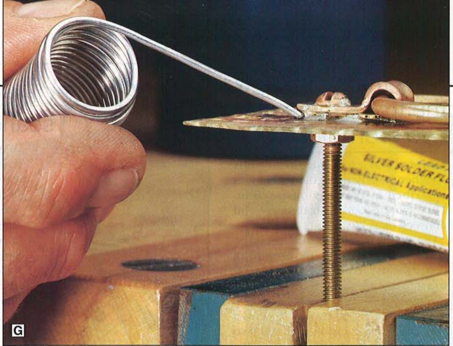
G Touch some silver solder to the fluxed and heated joints to secure them.
