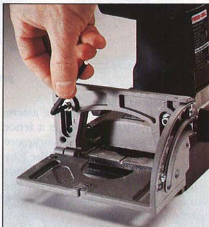
The fences on the Porter-Cable 556 (shown) and Skil require you to use an allen wrench to lock them in place.
