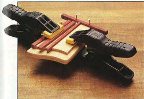
Scrapwood spacers (the dark pieces) help position the front and back dividers when gluing the end assemblies.
