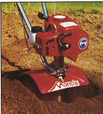
Mantis tines spin at 240 RPM
