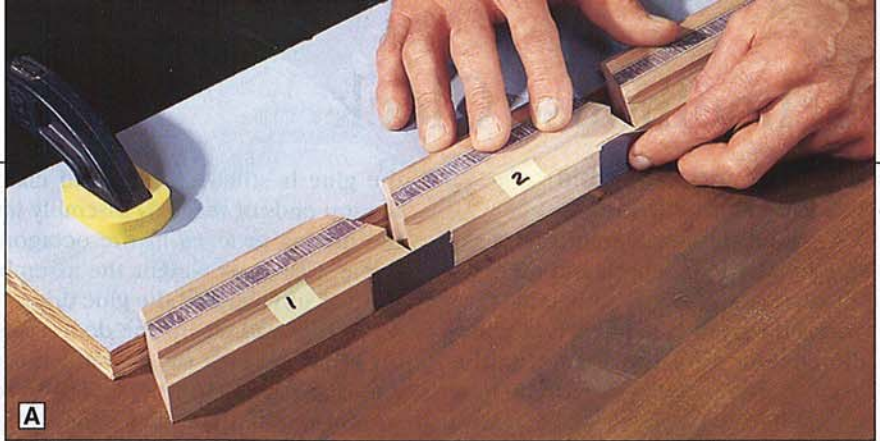
A Working on a flat surface and against a straightedge, tape the outside edges of the miter-cut octagonal frame pieces together.
