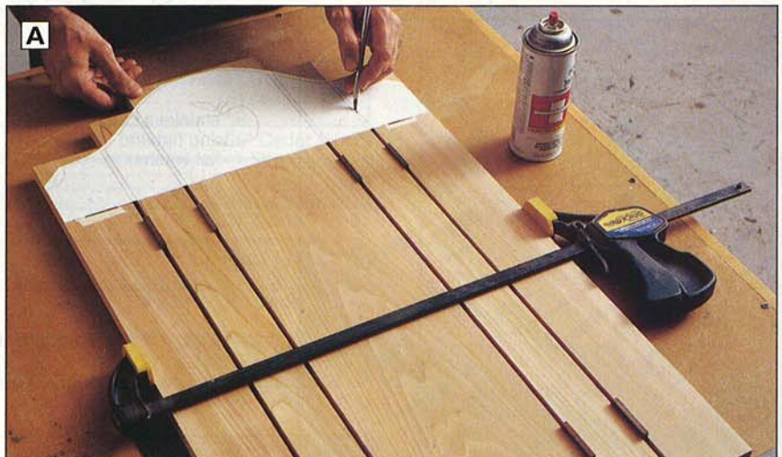
Clamp the backrest splats and spacers together, adhere the pattern, and cut the paper pattern from between the boards.
