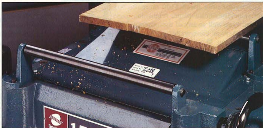
Stock return rollers on top of the planer make it easier to move long or heavy stock back for the next cut.
