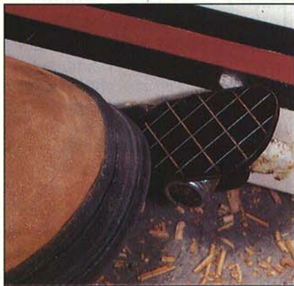
A foot-operated lever quickly and easily locks the wheels on the Jet JWP15-CSW's built-in mobile base.
