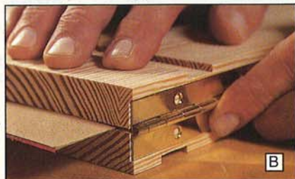
Use a tablet-back spacer to separate the seat halves and allow proper clearance.
