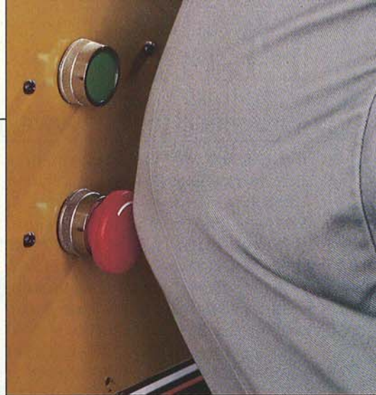
Powermatic's off switch is located within easy reach of the operator's knee, so we didn't have to reach across the planer to power it down.
