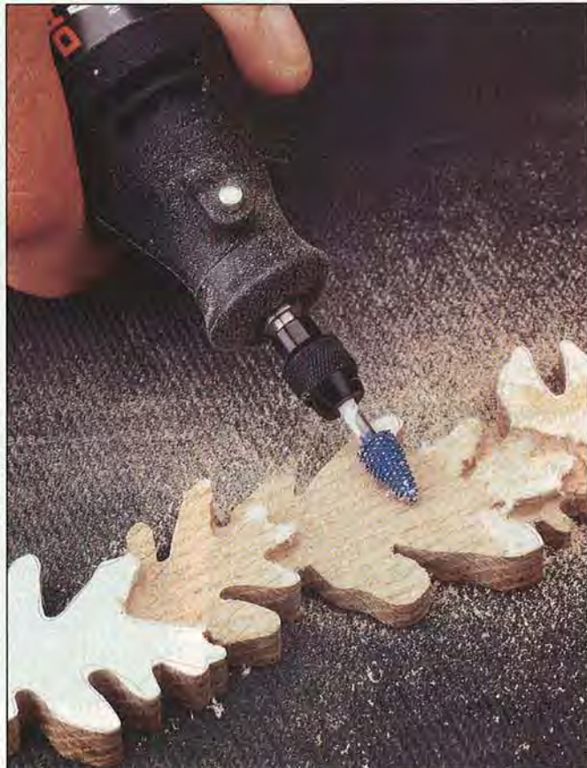
An aggressive carbide cutter, such as this Typhoon taper bit, makes quick work of tapering the leaf surfaces.
