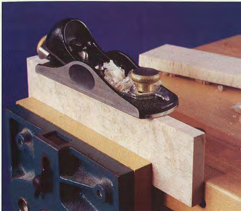
A hand plane (here, a block plane) with a low-angle iron makes clean cuts in figured stock. Adjust the iron and plane mouth for a whisker-thin shaving.
