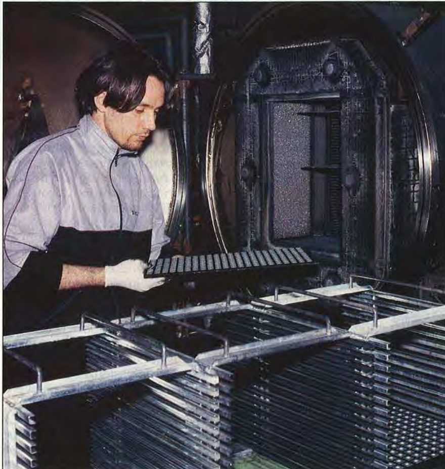
Trays of carbide tips go into an oven that fuses the powder together.
