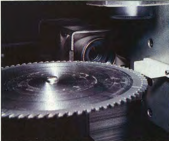
Electric eyes make 13 checks on the alignment and brazing integrity of each tooth in just a second or two.
