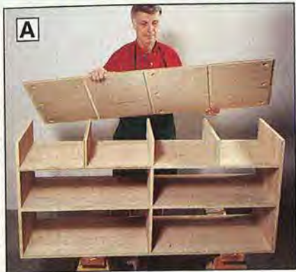
When assembling the plywood carcass, glue and screw the plywood carcass top in place last.
