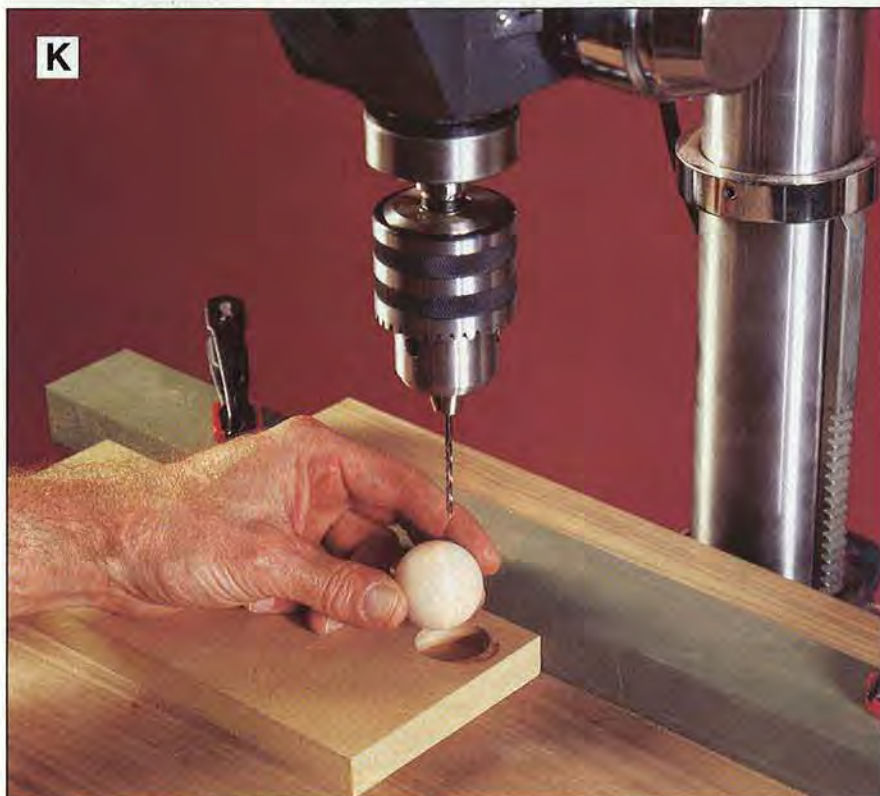
K A hole in a piece of scrapwood holds the ball for accurate drilling.
