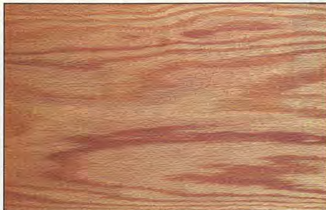
Use an untinted, natural oil slurry to achieve an even coloration in the filled wood grain, as on this piece of oak.
