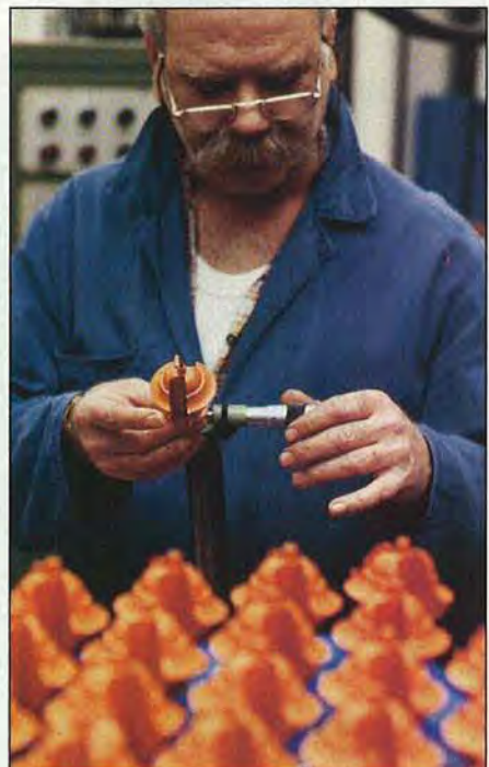
A micrometer helps this worker accurately check the diameter of ground shanks.
