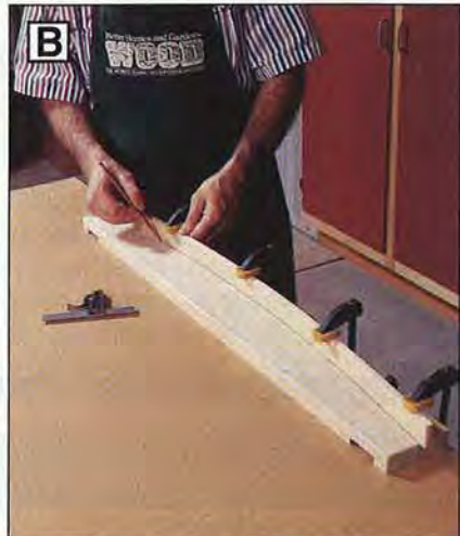
Clamp the top trim piece in place, and use it as a fairing strip to mark the curved cutline on the top piece.
