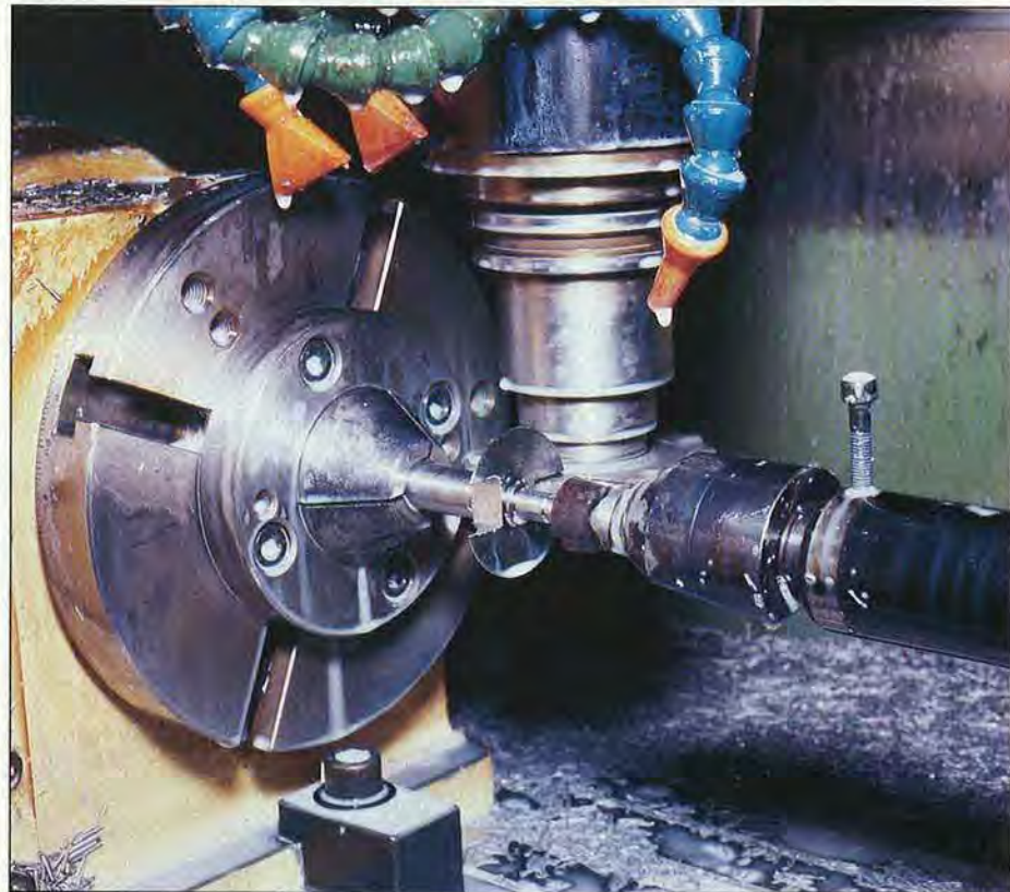
A milling machine cuts the two slots that will later accommodate the carbide tips.
