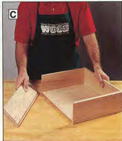
Dry-clamp each drawer together first to check the fit. Then, glue and clamp the parts, adding one side piece last.
