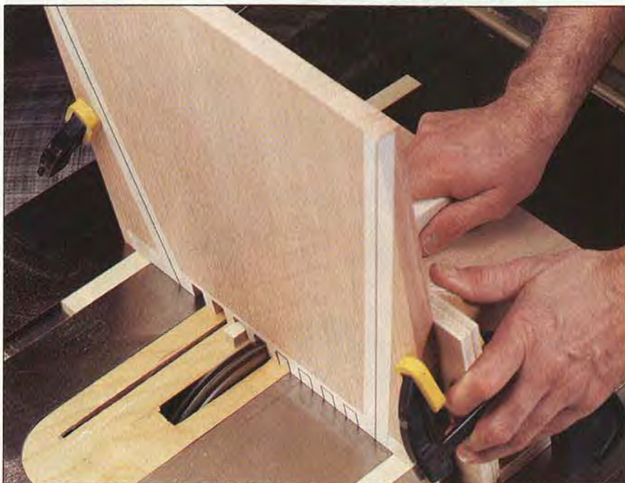
Clamp the workpiece to the jig, and press down at the back for stability while sawing.
