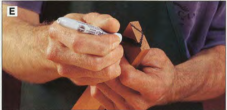
E Mark one end of the stock before resawing the laminations. After restacking the laminations in order, darken the mark if necessary to maintain orientation during gluing.
