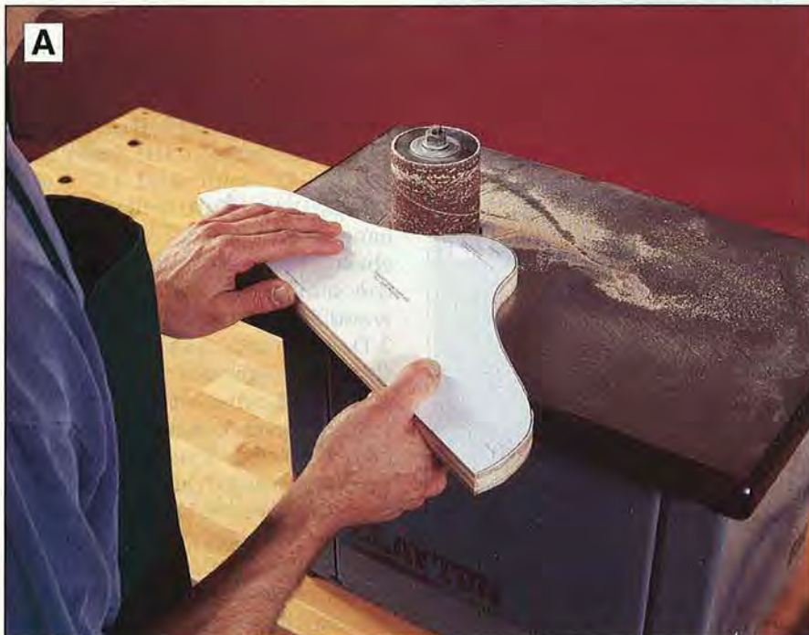
A Sand the edge of the template smooth and true. The router bit's guide bearing will ride against the curved surface.
