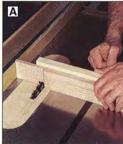
Use a tablesaw fitted with a dado blade to cut a shoulder on each half-lap so the stile fits snugly into the mating joints.
