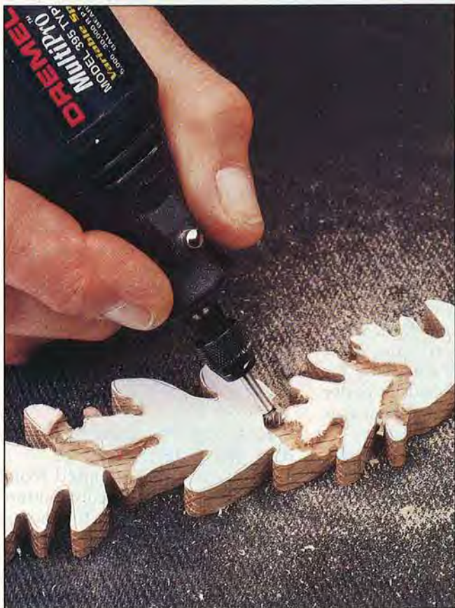
Outline the overlapping leaves with a spherical cutter. Don't worry if you stray slightly from the pattern line.
