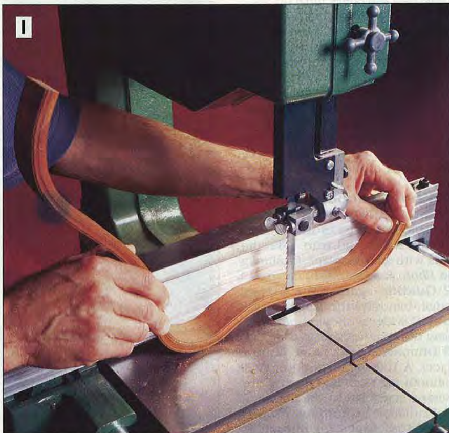
Guiding against the planed edge, bandsaw the laminated blank to width. Allow a little extra width, then plane or sand to finished width.
