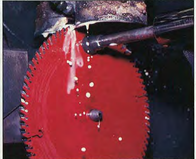
Dual diamond wheels side-grind the carbide teeth. Other wheels grind the teeth faces and tops.
