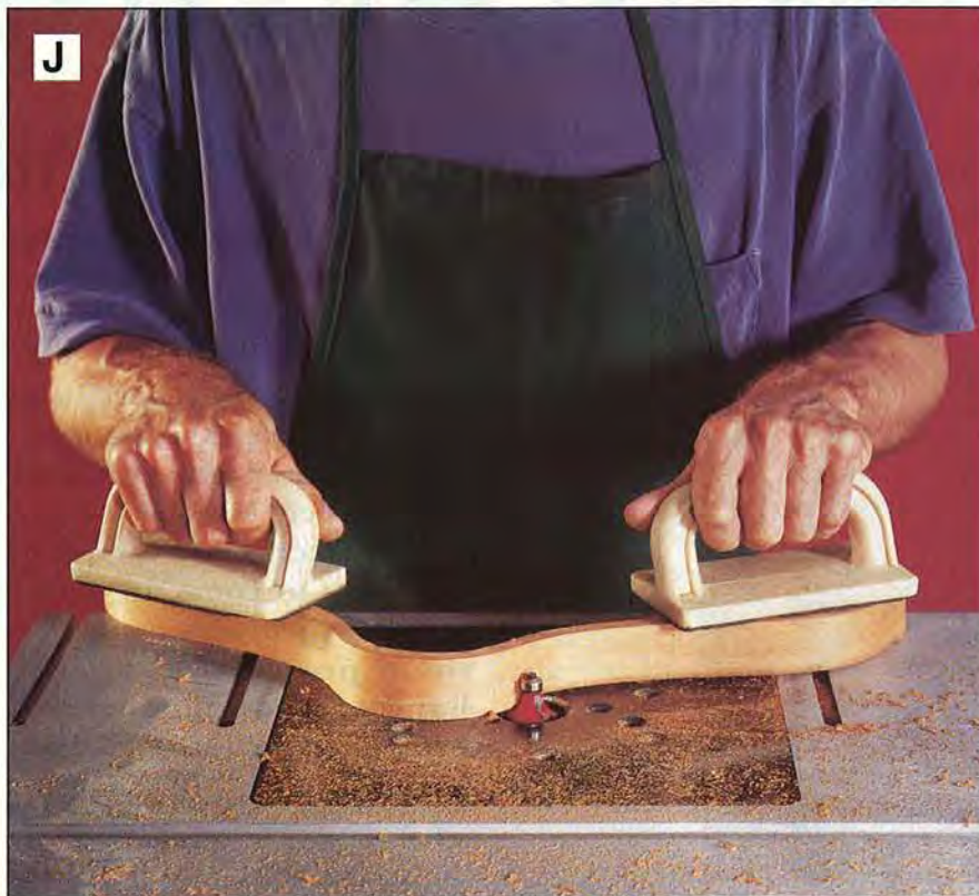
J Pad-style pushblocks help safely rout round-overs on the top edges of the hanger. Rout before cutting off the ends.
