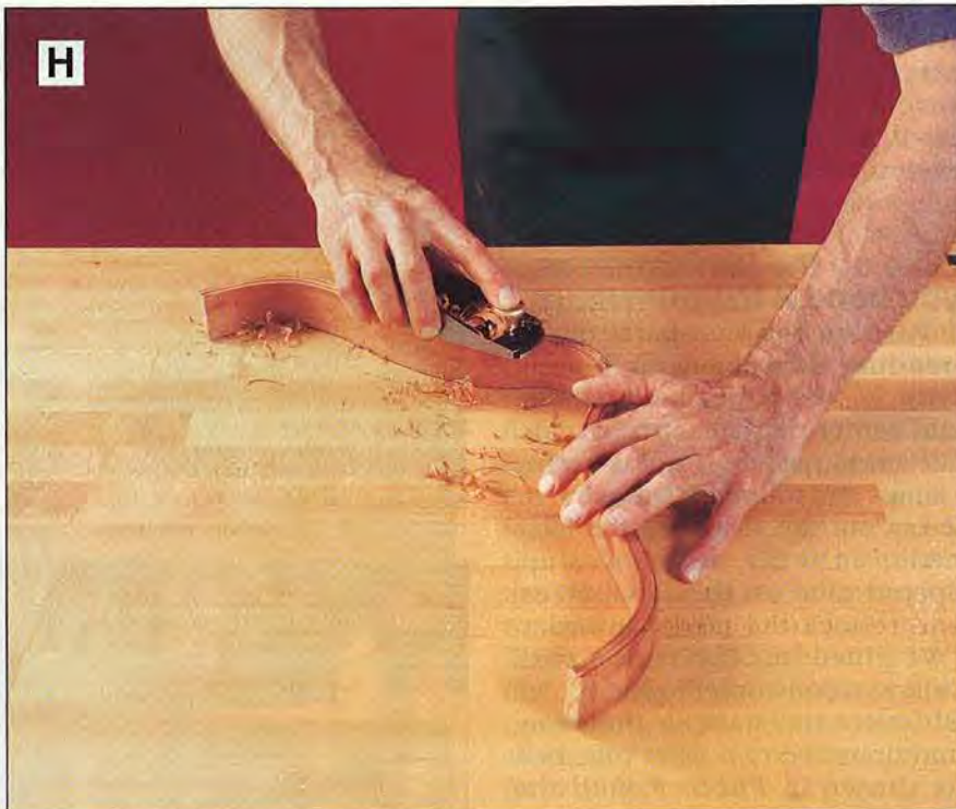
Plane one edge of the lamination smooth and straight after removing it from the form.
