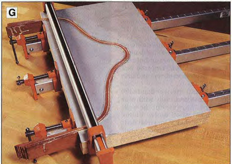
G Secure the form sections with bar clamps while the glue dries. The clamp across the bottom draws the lamination tight at the ends.
