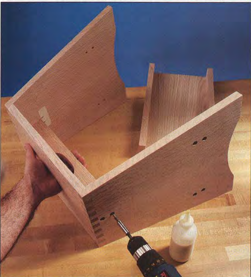
Screw the crossbar (C) into place to clamp the joints at the correct angle.
