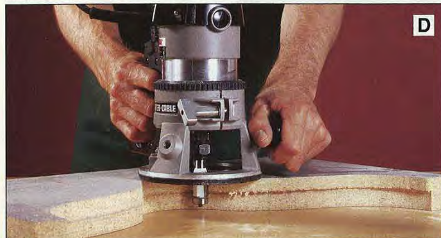
D After separating the form sections, trim the sawn part of the edge with a flush-trimming bit. Guide against the routed part of the edge.
