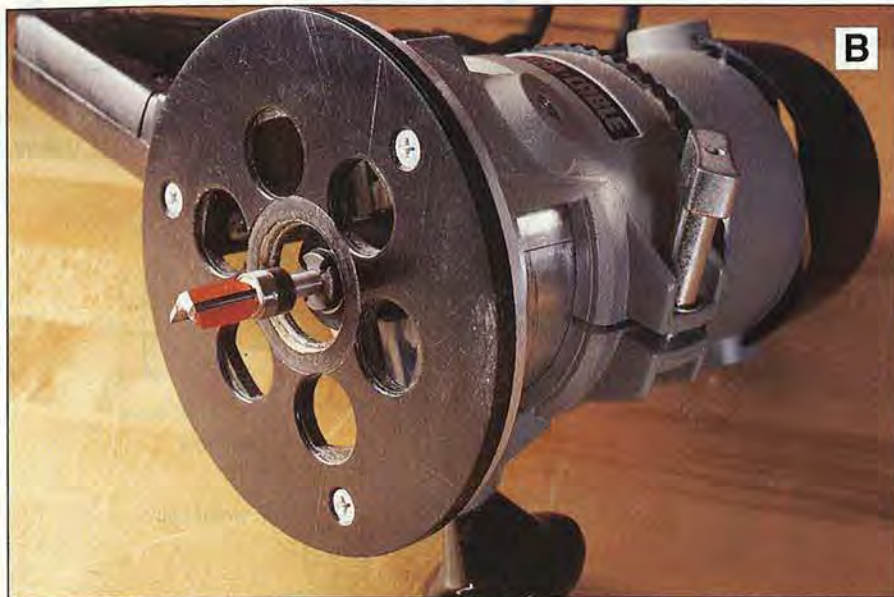
B The pattern bit's guide bearing sits atop the cutter. When cutting the lamination form with this bit, make shallow passes.
