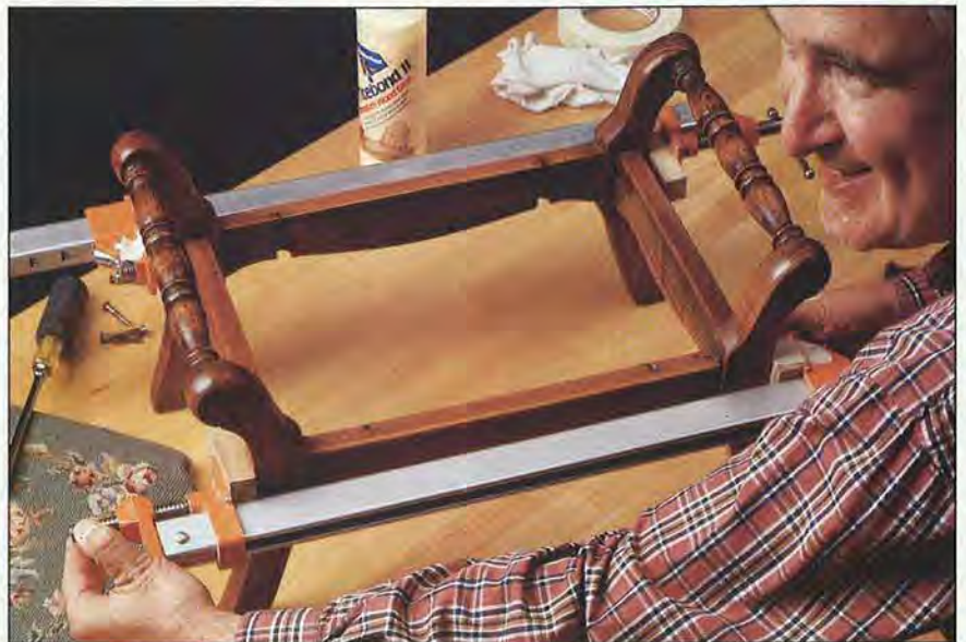
Gluing loose joints was all it took to put this needlepoint footstool back in service.
