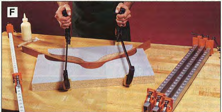
F Pull the form sections together with quick-acting clamps. Keep sides flush as you force the lamination into the curves.
