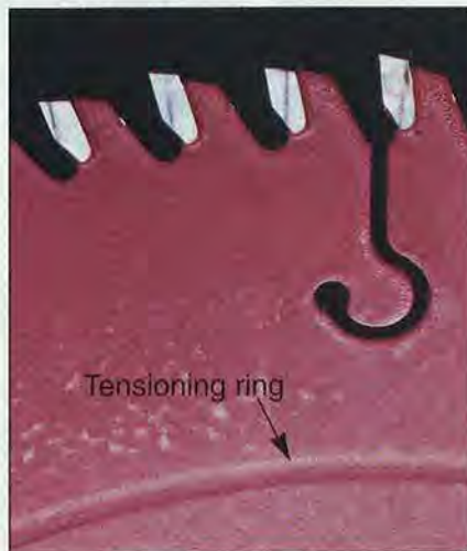
A machine automatically tensions each blade by pressing a ring into both sides.
