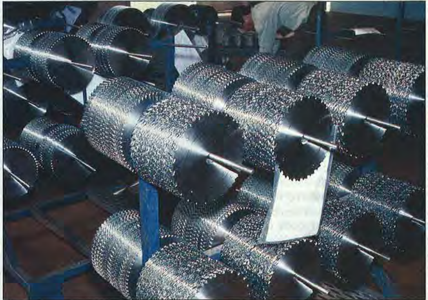
Thousands of saw blade blanks sit ready at a Freud plant, awaiting carbide teeth.
