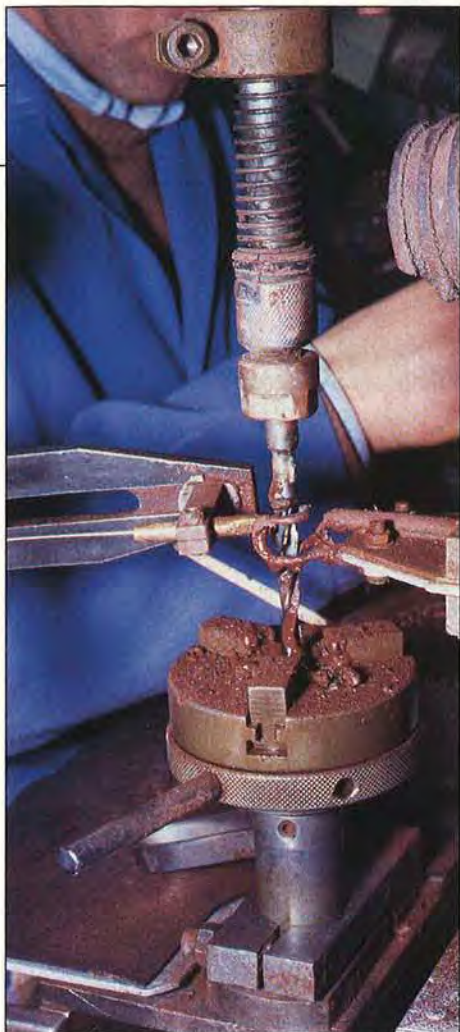
An induction brazer emits an electrical field to heat a bit without touching it.
