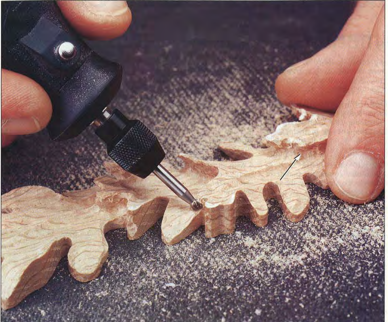
Shape the leaves' fronts with the ball cutters, raising a central vein. Undercut the edges (at arrow, for example) with a smaller ball.
