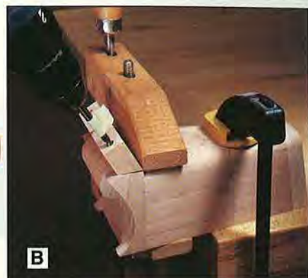
B Use the bottom of the windshield blank as an alignment guide to drill a pair of mating holes into the hood assembly.
