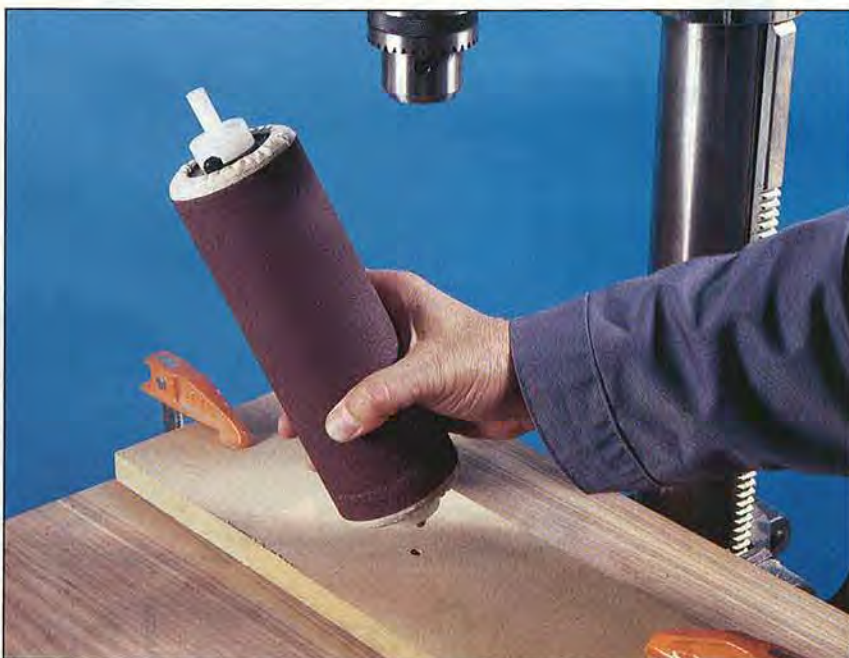
A pin on the bottom of the drum fits into a hole for support while sanding.
