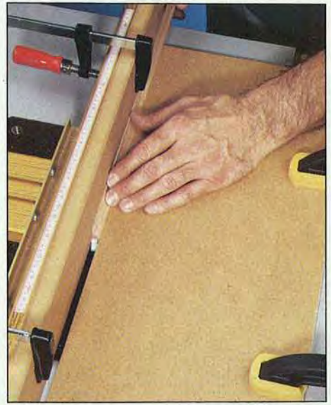
The guide board extends past the router bit to prevent chatter and keep the workpiece in contact with the fence.
