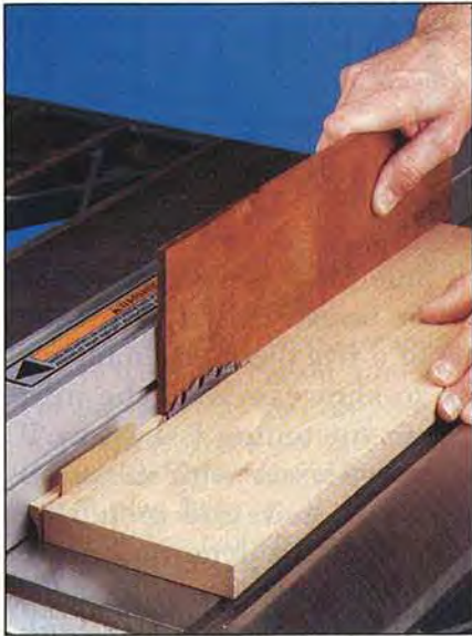
A tall, narrow pushstick keeps your fingers far away from the blade when ripping thin molding from the blank.
