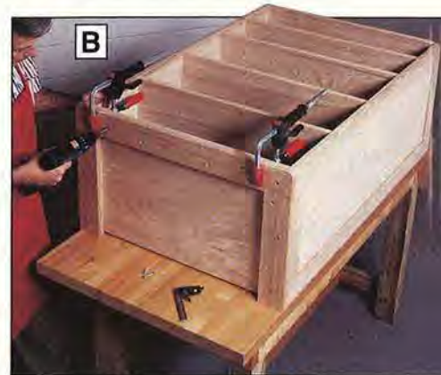
With the back edges flush and an equal overhang along each side, screw the base to the bottom of the carcass.
