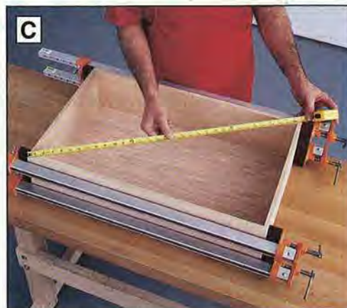
Measure diagonally from outside corner to outside corner. When the measurements are identical, the drawer is square.
