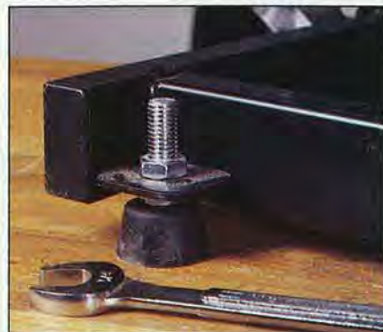
Leveling pads on the Delta and HTC (universal only) bases require that you bend down and use a wrench for adjustments.
