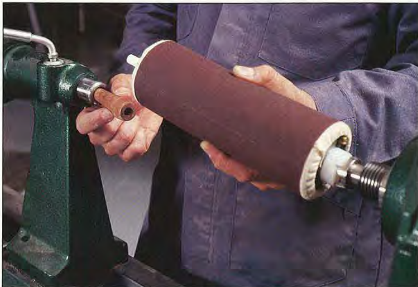
For lathe-mounting the drum, we turned a wooden bearing to fit into the tailstock
