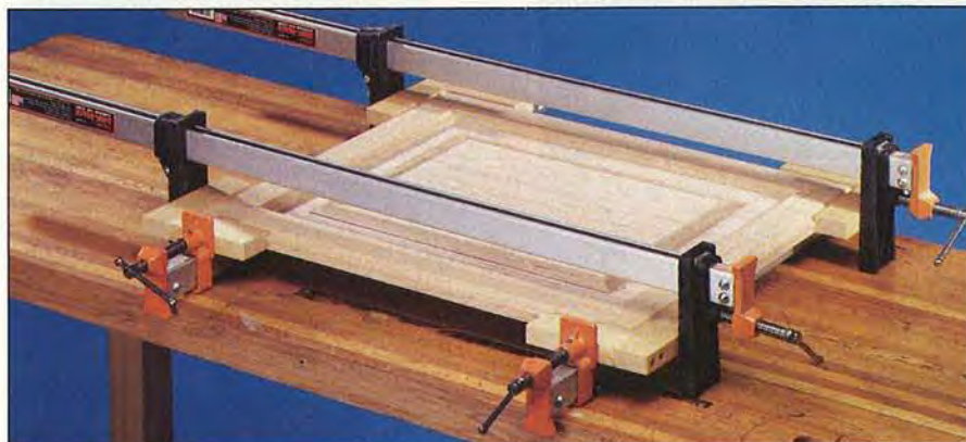
You'll find the clamping process less clumsy if you use a pair of bar or pipe clamps with extended-reach jaws.
