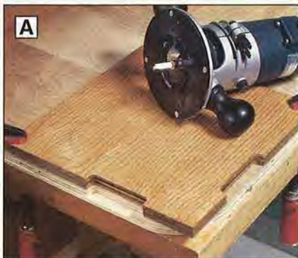
A Clamp the template in place, and rout the recesses. Reposition and rout until all eight recesses have been formed.
