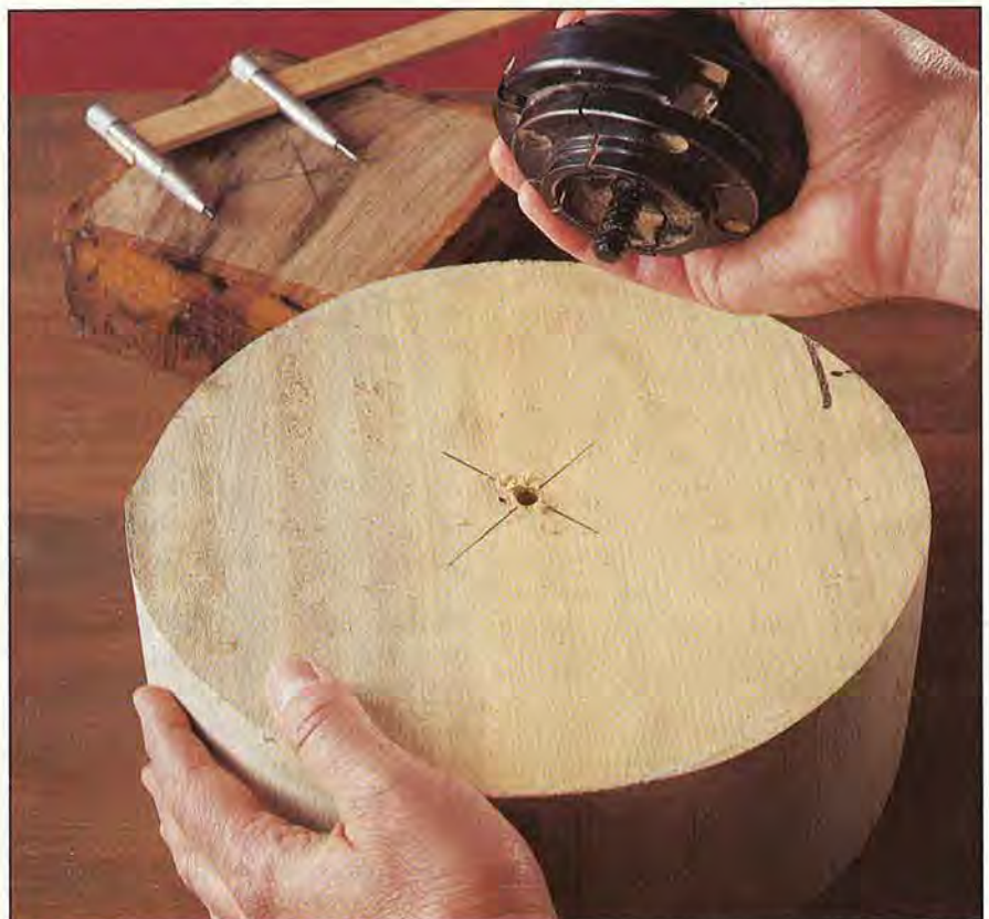
A screw center holds the bandsawn blank for turning. We'll bandsaw a blank for a small bowl from the smaller block.
