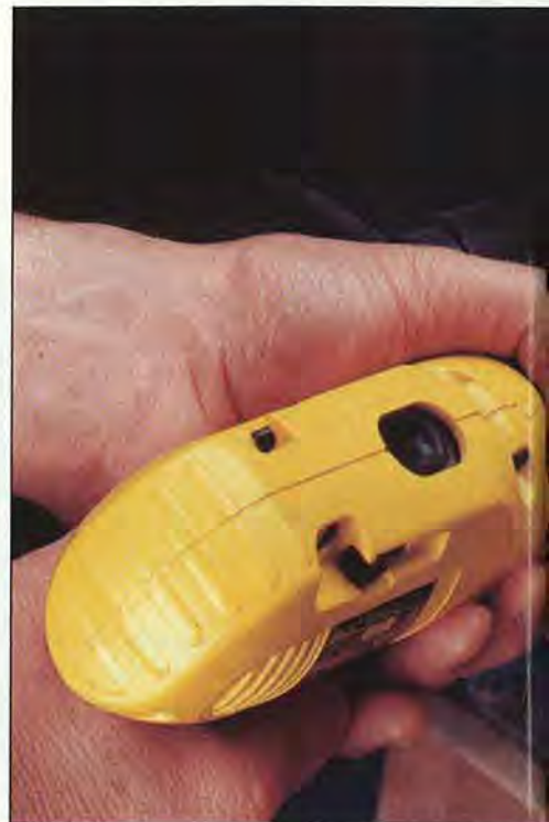
Power-sanding with a resilient foam pad smooths the bowl's curve.
