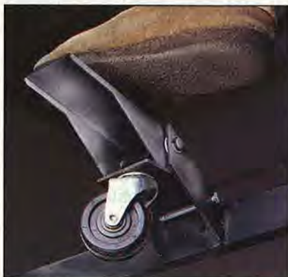
By pressing down or lifting up on a foot pedal you can quickly convert some bases from mobile to stationary.
