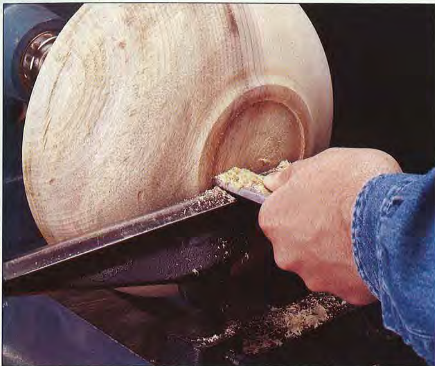
Lay your skew chisel flat on the tool rest to form a dovetail mortise for the bowl chuck. For turning on a wasteblock, form a flat gluing face here.
