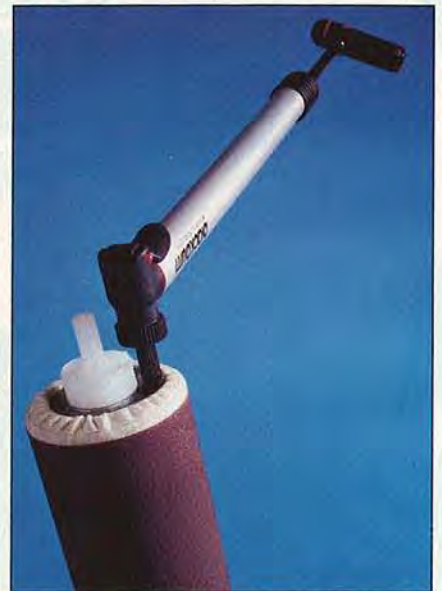
A hand bicycle pump will inflate the drum sufficiently in just a few strokes.
