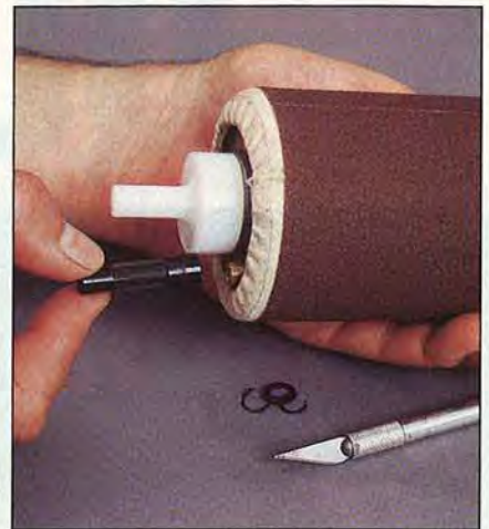
Screw on an extension to make the valve stem more accessible.
