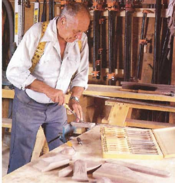
"To build Victorian furniture, you have to learn to carve," advises Charlie as he cuts into a walnut scroll piece intended to replicate original trim on a bed's headboard. "It can also be fun."
