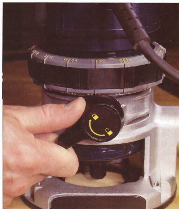
The Ryobi routers have innovative and easy-on-the-fingers cam locks for securing the motor housing to the base.
