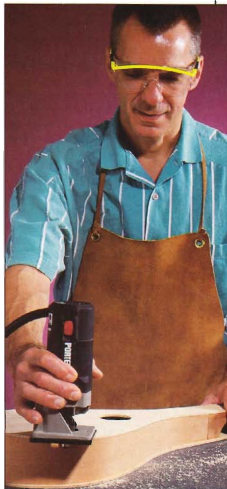
Jan uses the laminate trimmer to trim the sound board on his small guitar.
