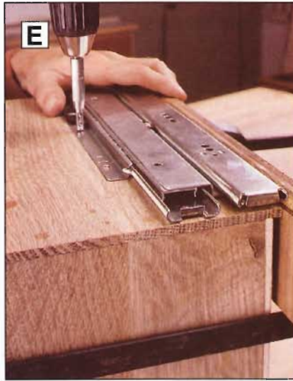
E We used a rabbeted piece of plywood to position the bottom edge of the slide \frac{1}{8} " below the bottom edge of the drawer.
