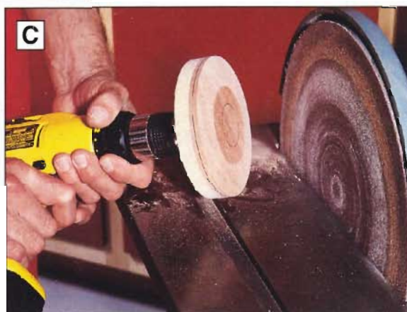
Form the beveled surface on the cap (E) by spinning the piece against a disc sander ( above ). The reference circle and edge line show the limits of the bevel ( right ).
