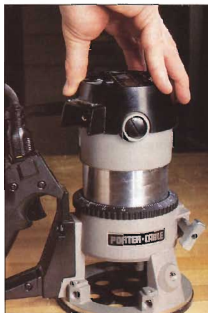
A fast and simple twist of the motor housing raises or lowers a Porter-Cable router to the correct cutting depth.
