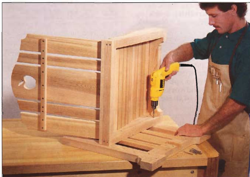
Drill the mounting holes and drive the screws to secure the front seat support to the front upright.
