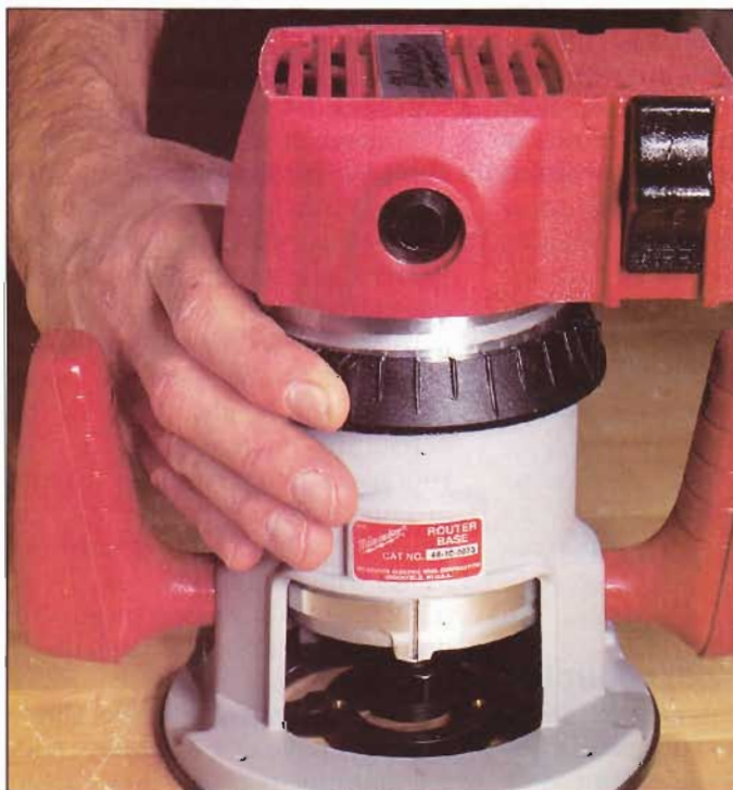
We found depth-adjustment rings, like the one shown here on a Milwaukee router, difficult and time-consuming to adjust.
