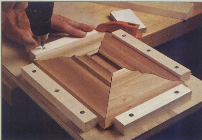
Attach four cleats at right angles to each other to hold the lid pieces in position on a plywood clamping platform.
