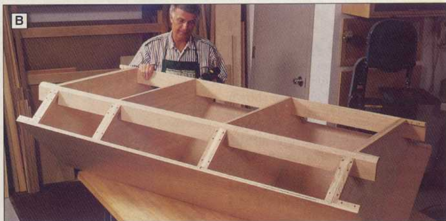
Secure the notched supports to the previously installed shelves by driving wood screws through the previously drilled cleats.
