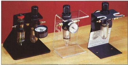
The regulators for the Foredom 350K (left), SCM 400XS (middle), and Paragrave come with filters and moisture traps installed, a requirement for prolonging bearing life.
