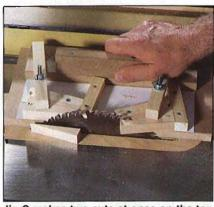
Jig C makes two cuts at once on the top staves. Blanks must seat firmly against the alignment blocks for accuracy.
