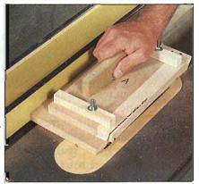
With the bevel angle established by the 11.25° blade tilt, Jig A rips one edge of the tapered, beveled staves.
