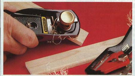
A block plane works great for corner chamfering, passably well for rounding over. For fine work, set the plane iron for a shallow cut and narrow the plane's mouth, if it's adjustable. You also could use a spokeshave, right.
