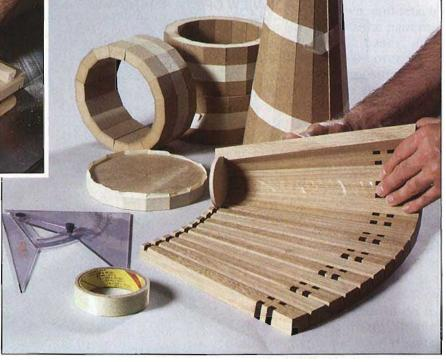
Held together with tape, the staves roll into a tapered cylinder like the one shown standing at the back. The adjustable triangle, left, helped set the blade tilt. Test staves form the two cylinders and the disc.
