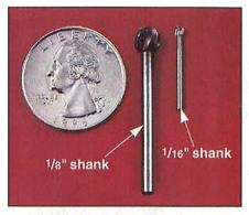
The 1/8"-diameter shank carbide bit typically used with motorized rotary tools (shown above and in the micro diegrinders below) dwarfs the 1/16"-diameter shaping wood and glass come in most of the same profiles as the carbide bits. More susceptible to heat damage, these bits cost \$3 to \$4 each. They're best suited for finish work because they cut less aggressively, and more smoothly, than carbide bits.
