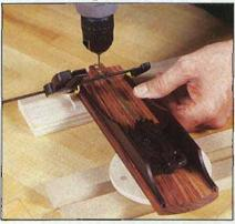
5 Remove the clock movement from the body. Finish-sand all the pieces and add the finish. Reattach the movement to the body. Then, screw the pendulum bob/spacer to the end of the pendulum. Attach the clock hands and install the battery. Set the time and hang in place.
