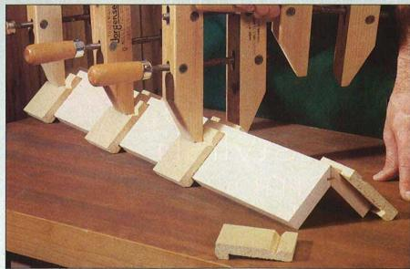
For a tight joint when joining the splined and mitered leg halves together, we used our handscrew clamps and shop-built clamping blocks.
