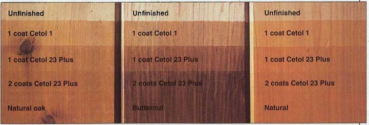
Although after application Cetol 23 has a clear appearance, it actually has a light pigmentation. As shown on these three sample boards, the tinted finishes still let the wood show through.
