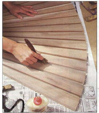
After laying out the staves in fan fashion, the drum maker applies glue to the mating edges with a brush.
