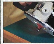
Trim the laminate and shape the edge banding at the same time. Rout counterclockwise around the top.
