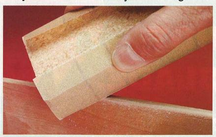
You can chamfer or round over a sharp corner with just a few strokes of a sanding block. Removing sharp edges gives your project a finished look and feel.
