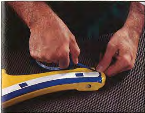
Tape around the pattern outline. Don't overlap the edge of the pattern while masking—you'll be removing it later.
