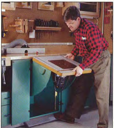
Editor Larry Clayton demonstrates the space-saving, flip-up storage of the router table beneath the workbench.
