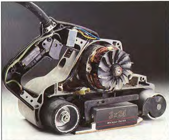
Mounting the motor transversely, as in the Porter-Cable 360VS (left), creates a high profile, although the handle remains near the center of gravity. An in-line motor design, used in the Ryobi BE-321 (right), creates a low-slung, compact design with good balance.
