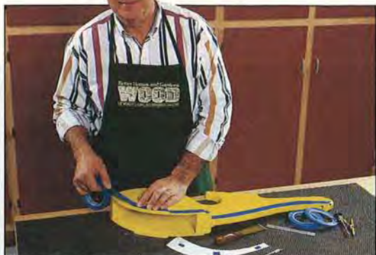
A strip of \frac{3}{4} "-wide masking tape establishes the reference line parallel to the edge of the frame. We used Scotch #471 tape for masking.
