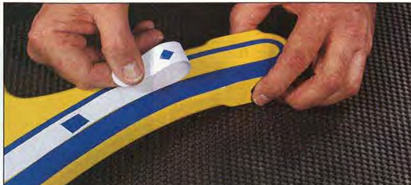
Place tape over the diamond cutouts in the pattern to affix it to the frame. The pattern serves as a guide for taping an outline of the stripe, so it cannot be taped down along the edge.
