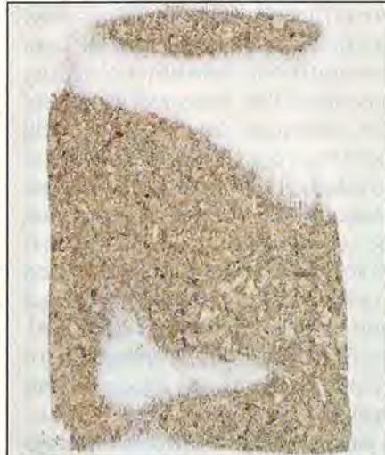
A flat platen created an even pattern (left) when sanding polyester-coated particleboard. Uneven marks (right) show the platen had ridges and low spots.
