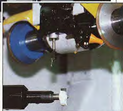
Above: State-of-the-art 5-axis CNC grinding centers put accurate and complex cutting edges on Jesada bits.
