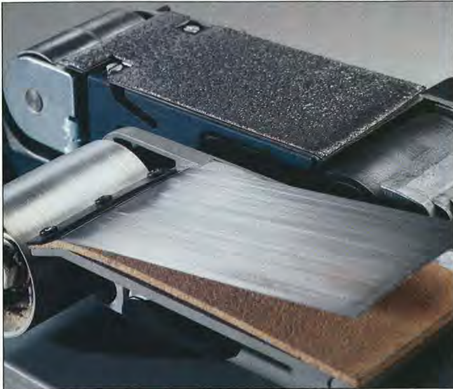
Cloth-backed graphite slip plates (top) conform perfectly to the platen. Tempered steel slip plates (bottom) don't lie flat against the platen along the bend line, a problem compounded when the cork pad compresses under the mounting screws.
