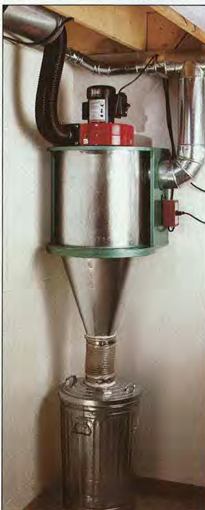
In a corner or against a wall, this highly efficient cyclone dust collector requires minimal space with easy access to the waste can.
