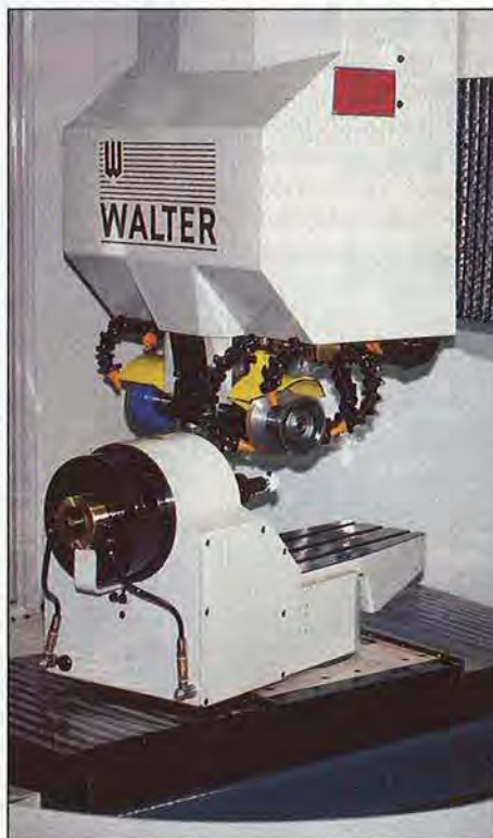
Above: State-of-the-art 5-axis CNC grinding centers put accurate and complex cutting edges on Jesada bits.
