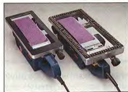
Sanding frames come with a phenolic base (left) or ride on hundreds of small brushes (right). We found that the latter glided more smoothly on flat workpieces.
