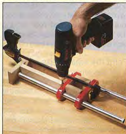
Place the short spacers between the fork blocks when assembling the fork. Push the tubes in until they contact the stop.
