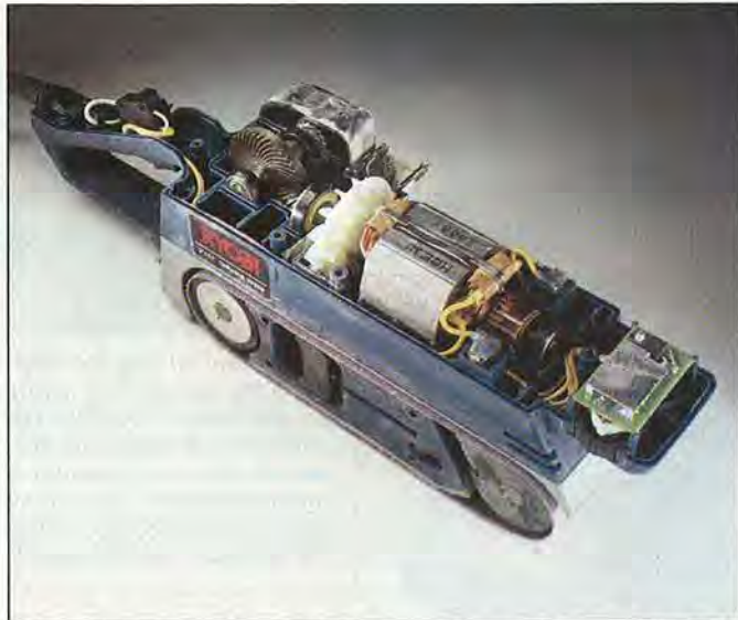
Mounting the motor transversely, as in the Porter-Cable 360VS (left), creates a high profile, although the handle remains near the center of gravity. An in-line motor design, used in the Ryobi BE-321 (right), creates a low-slung, compact design with good balance.
