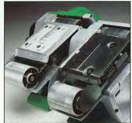
Cast-aluminum platens (left) proved flatter and more rugged than platens stamped from steel (right). Stamping and machining for mounting screws also warps the steel.
