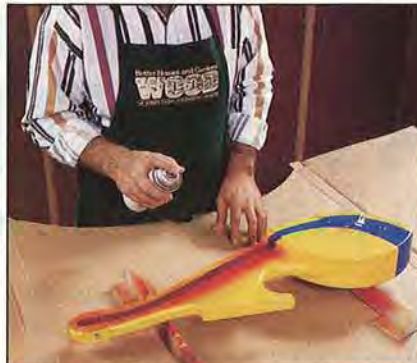
With the stripe masked off, paint the entire frame red. Removing the tape will then reveal the yellow stripe.
