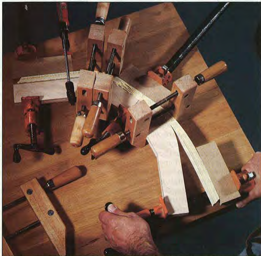
Dry-clamp the handlebar strips (F) to the form (G) before gluing. This allows you to work out your clamping scheme ahead of time.
