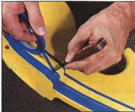
After removing the pattern, mask the stripe area. Tape must not overlap the guide strips, as they will be removed.
