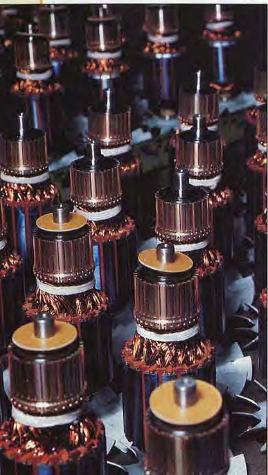
The armature assemblies of universal motors roll off Taiwanese assembly lines by the thousands every day.
