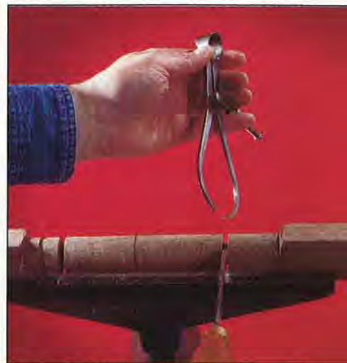
Set caliper to the desired diameter to gauge the parting-tool cuts.
