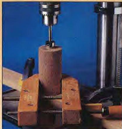
Hold the pepper mill blank with a hand-screw clamp as you bore the center hole. Line up the bit with the center mark on the tenon.
