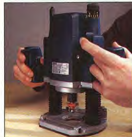
The Bosch 1613EVS has a convenient in-handle trigger switch and an easy-to-reach spring-actuated locking lever.
