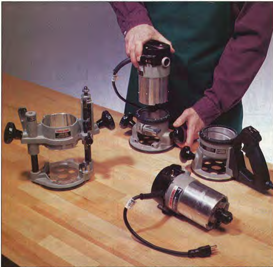
The same Porter-Cable motor fits into the three bases shown from left: plunge, two-knob, and D-handle.
