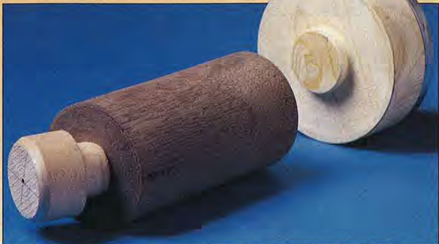
The bottom of the blank fits over the tenon on the jam chuck (right). The plug (left) fits into the bottom hole for mounting the bored blank.
