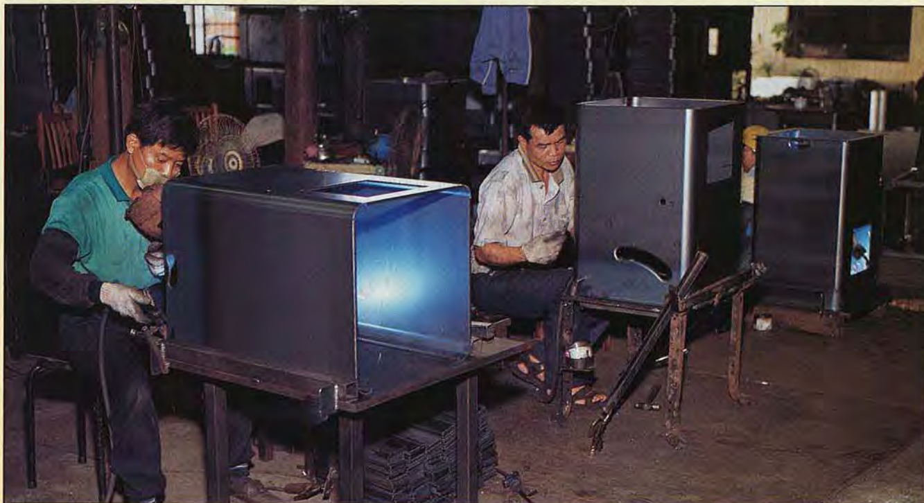
Manual labor costs are much lower in Taiwan than in the U.S. Here, workers weld together bases for Grizzly cabinet saws.
