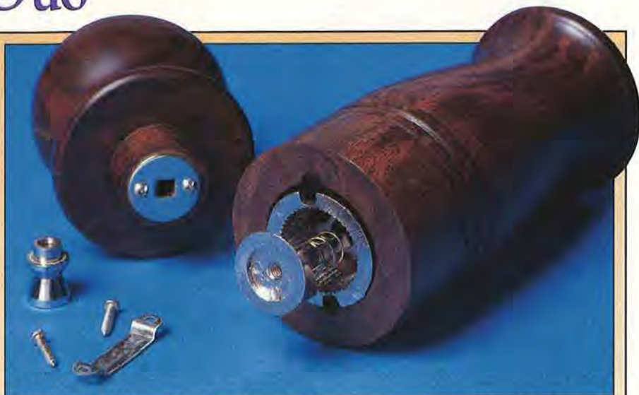
The drive plate shown on the bottom of the top's tenon engages the square mill shaft. Align the slots on the mill housing with the notches in the turned body.
