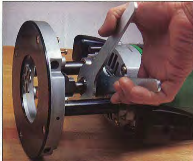
Two wrenches give you plenty of leverage to loosen a stubborn collet. No strain, no banged knuckles.
