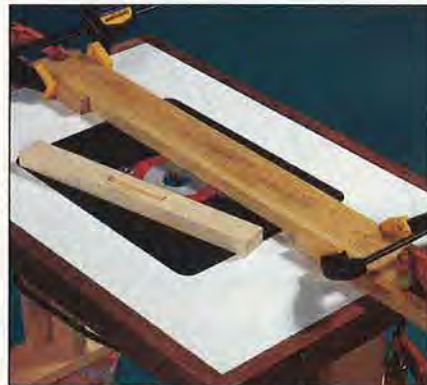
Use a pair of stops clamped to the fence when routing the 3"-long covers on both sides of the handle blank.
