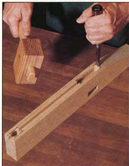
After removing most of the waste from the marked mortises with a Forstner bit, complete the mortises with a chisel.
