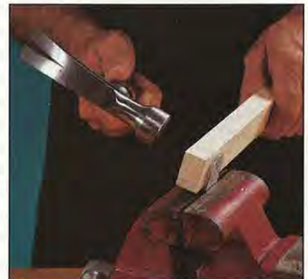
Use a scrapwood block to aim the force of hammer blows at the bending line.
