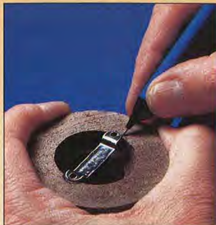
Draw or scribe around the ends of the retaining strap to mark the notch locations. Lay the strap in the hole upside down as shown to make this easier.
