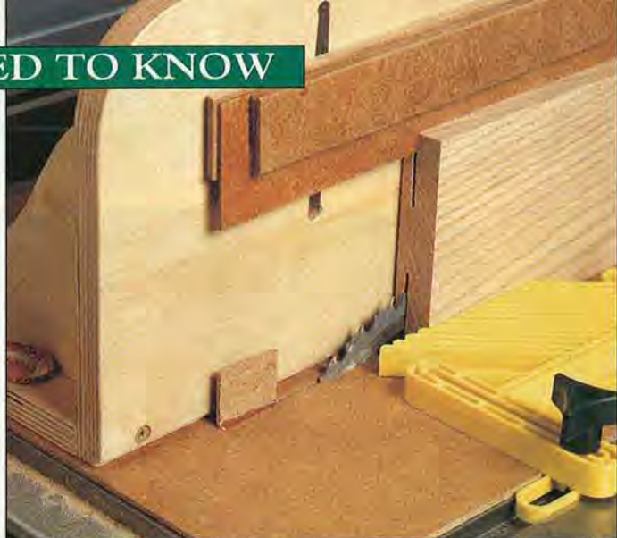
The splitter keeps the stock from binding against the blade, and the upper guide assembly helps hold the stock against the fence. Use a pushstick and feather board for safety.
