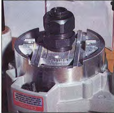
Lower-cost routers have lower-arbor bearings supported by plastic (left). On high-quality routers these bearings are supported by aluminum (right).
