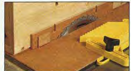
To set the fence, place spacers between it and the blade. Clamp the fence, then put the spacers behind the upper guide.
