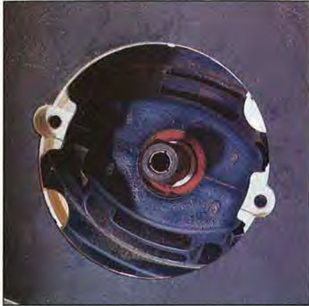
Lower-cost routers have lower-arbor bearings supported by plastic (left). On high-quality routers these bearings are supported by aluminum (right).
