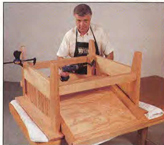
With the chair upside down, clamp the pivot blocks in place and secure them with screws.
