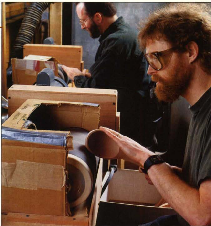
All of the cherry utensils get a final smoothing with 220-grit at one of two inflatable drum sanders. Ian Keal works in the background behind Jonathan. For a finish, the utensils receive a coat of high-grade mineral oil.
