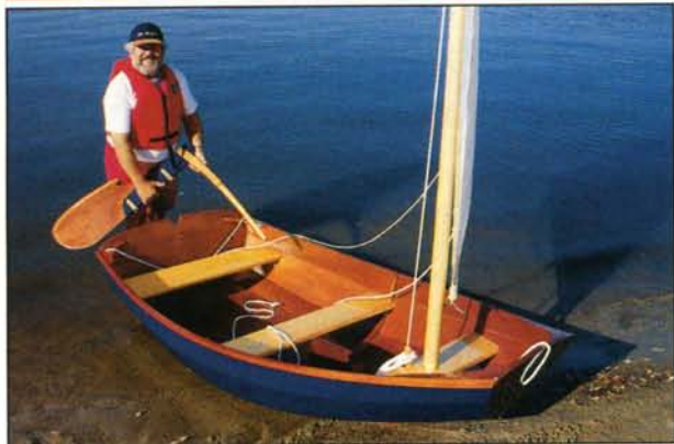
Jim Downing's lapstrake sailing pram kit from The Wooden-Boat Store took him 60 hours to build. "Small but stable, it handles like a dream," he says.
