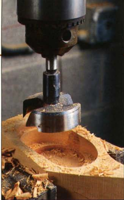
After sawing a ladle to shape, the bowl is roughly bored out at the drill press with overlapping bites of a Forstner bit.
