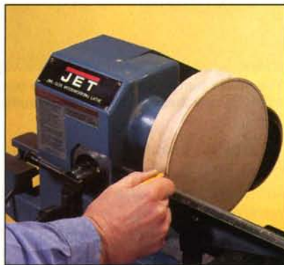
Draw pencil lines on the face and rim of the blank as guidelines for rounding over the clock's back edge.
