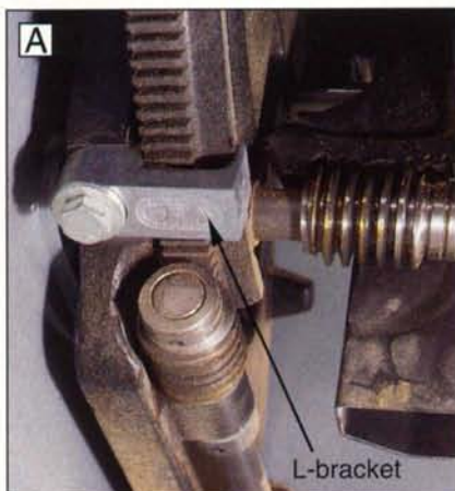
An L-bracket on the Delta prevents its yoke-style trunnion carriage from twisting when adjusted for 45° bevel cuts.
