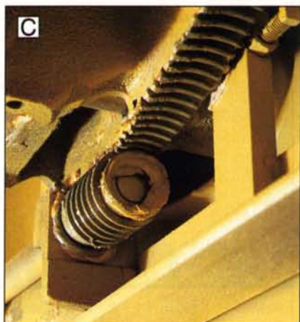
Only the Powermatic has concave-ground gear teeth for longer wear and smoother operation.
