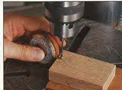
Support the post with scrapwood while you drill it to accept the chain hook.
