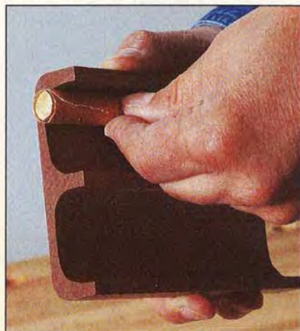
Sand the inside curves with sandpaper wrapped around a dowel.
