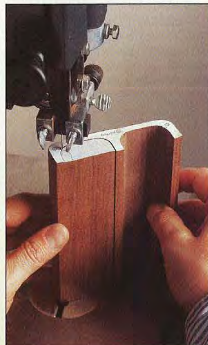
Stand the lid and bottom on end to saw the inside contours.
