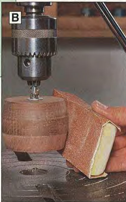
B Chuck the threaded end of the carriage bolt into your drill press, and sand the center boiler section smooth.
