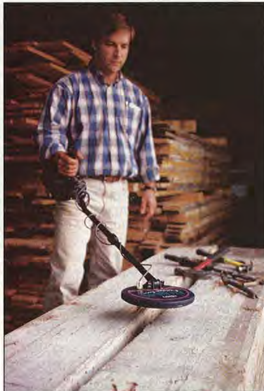
Before salvaged wood is sawn, workers must go over it thoroughly with a metal detector to find nails, bolts, and other objects that would damage an expensive blade during remilling.
