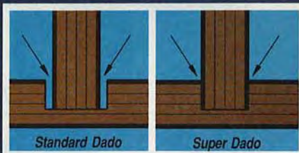
Exclusive 3/32" Chipper lets you perfectly adjust the width of the cut for today's undersized plywood.
