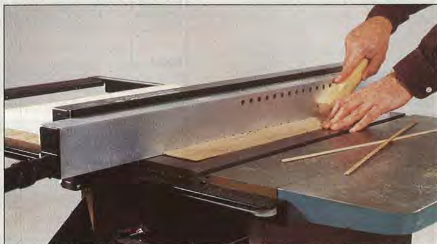
The Vac-U-Fence excels at helping you rip thin strips, among other things.
