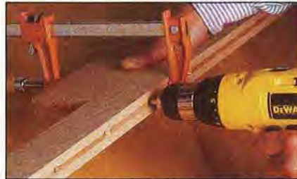
Mark the hole locations on the foot peg blanks by drilling through the holes in the leg blank.
