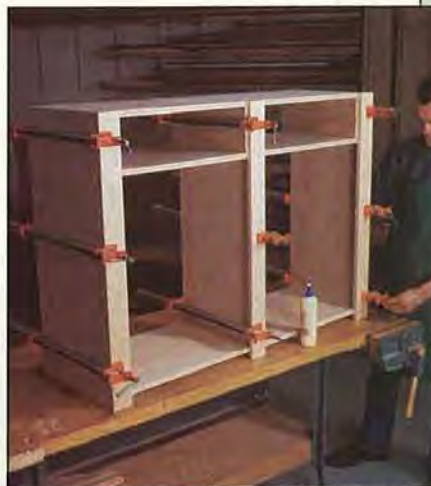
Glue and clamp the stiles to the carcase first. Then, measure the distance between the stiles and add the rails.
