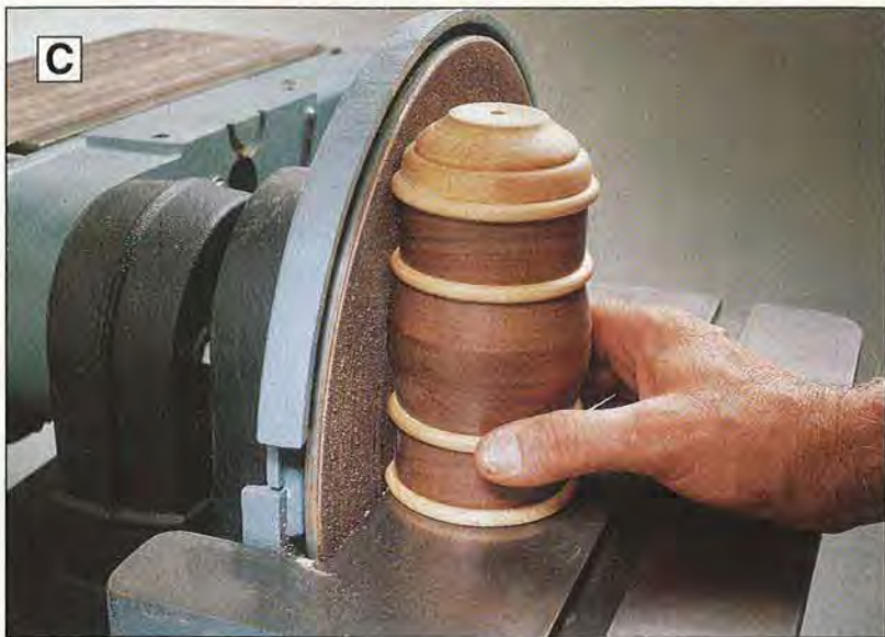
C Use a disc sander to sand a flat area on the bottom of the boiler for mounting the boiler to the chassis later.
