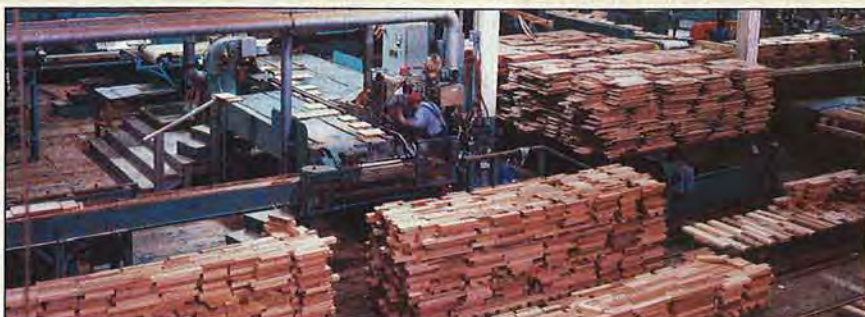
At Pacific Lumber Company's Scotia, California, plant, short redwood cutoffs from the sawmill that were once waste are finger-jointed into vertical-grain siding and other premium architectural products.
