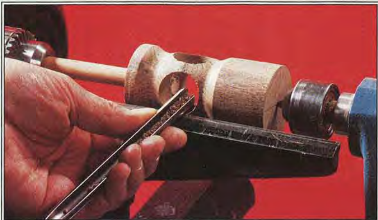
Run the lathe at 1100–1500 rpm when turning the bored-out center. Slower speed increases the risk of breakage.
