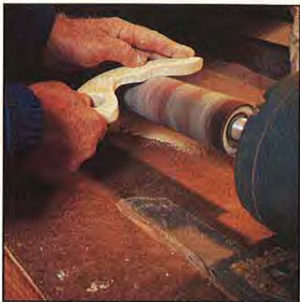
Wolf cuts each piece for a picture to rough shape on a bandsaw, then contours it with an inflatable drum sander.
