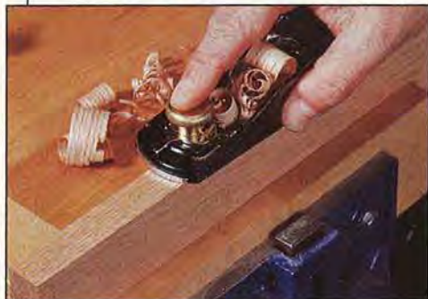
The compact block plane fits your hand comfortably, making it easy to use.
