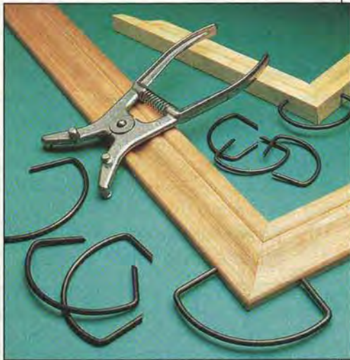
Spring clamps work simply and effectively. They leave small indentations in the frame edges that fill as easily as brad holes.
