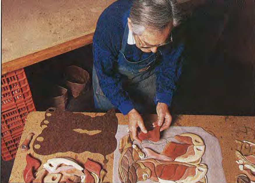
After the first pass by the sander with 40-grit, the assorted wooden pieces go back down on the pattern for a final inspection.
