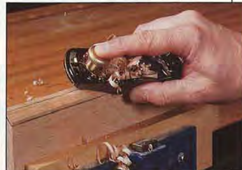
Angle the plane across the edge of the workpiece to form a bevel or chamfer.
