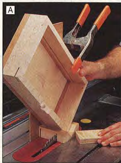
Use a spline-cutting jig to support and angle the box for cutting the 1/8" kerfs in the corners.
