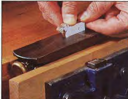
Clamp the block plane upside down in a vise to plane tiny or hard-to-hold pieces.
