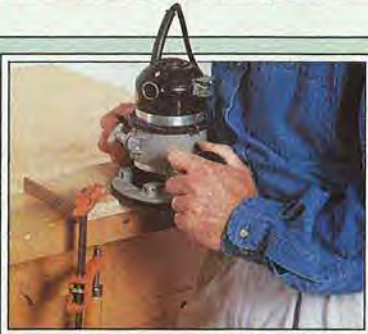
Edge-routing can mean shuffling clamps to keep them out of your way.
