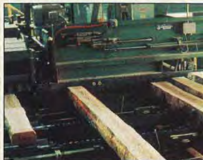
Computer-guided lasers (the orange lines) help determine the best position for maximum lumber recovery on the gang saw at Weyerhaeuser's Green Mountain, Washington, sawmill.
