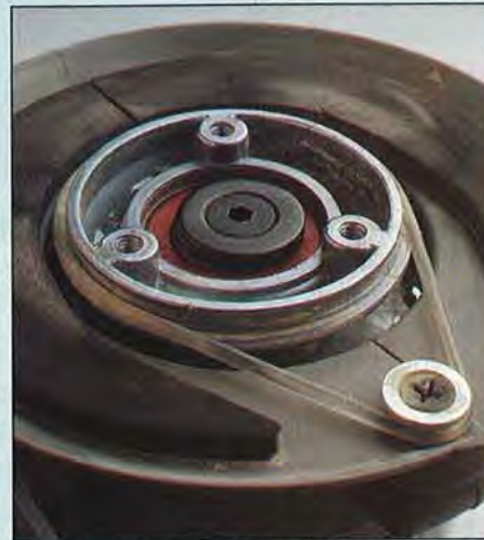
The Porter-Cable 333’s pad-brake mechanism has a rubber belt wrapped around the pad mount and idler pulley (sanding pad removed for clarity).
