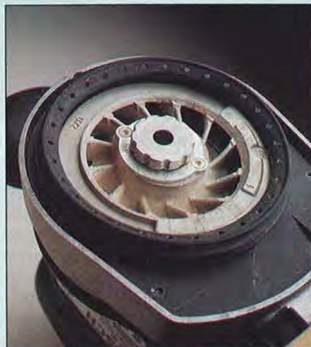
The pad brake on the Bosch 3725DVS consists of a rubber ring that contacts the underside of the sanding pad (pad removed for clarity).
