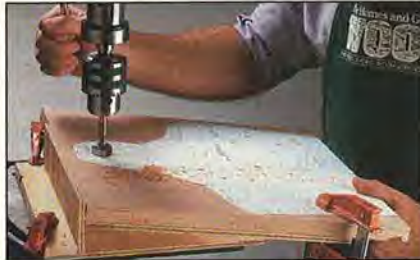
Using an angled support on your drill-press table to position the end-panel blank at 8^\circ , drill a 1" hole in each one.
