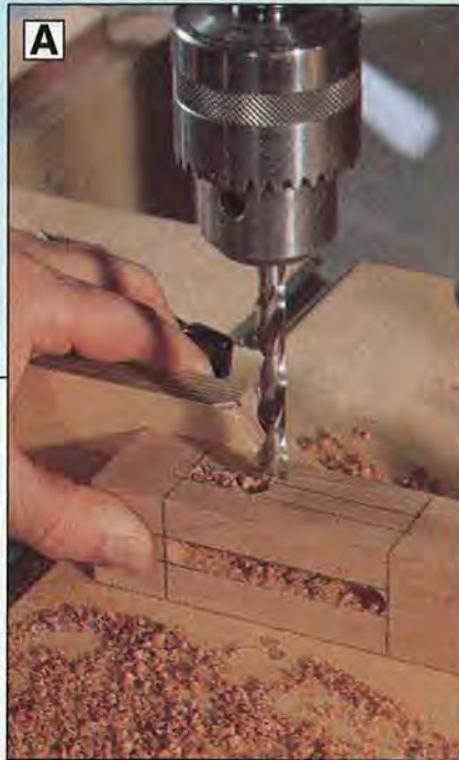
Mark the mortise locations carefully, and use a drill press with a fence for alignment to remove most of the stock.
