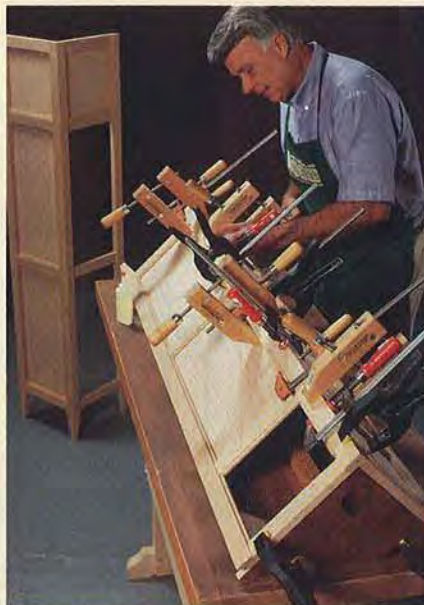
Using right-angled pieces at each end to keep it square, glue and clamp together two frames at a time.
