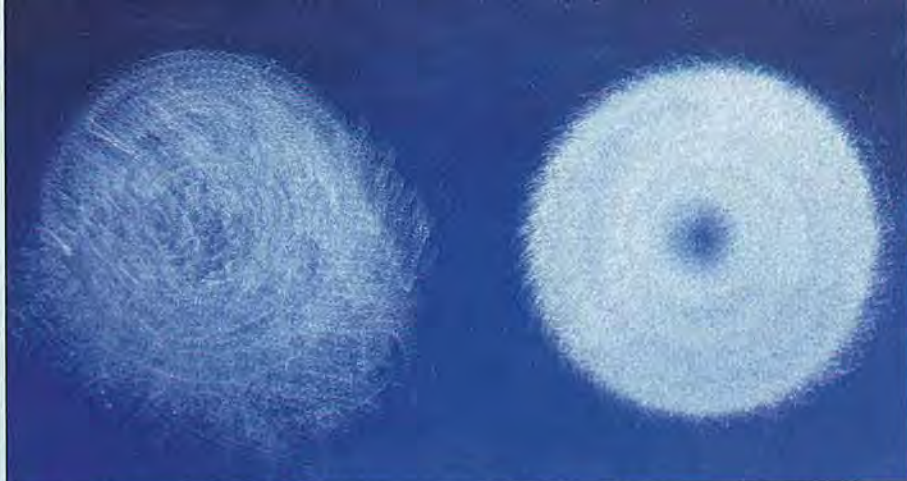
The Bosch 3725DVS left hard-to-detect scratches (right). Most low-cost models leave detectable scratches such as those produced by the Sears 27717 (left).
