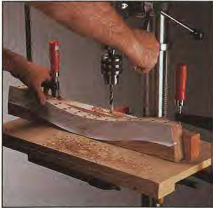
Mount a fence to your drill-press table for accurately centered holes in the bottom edge of the rails.
