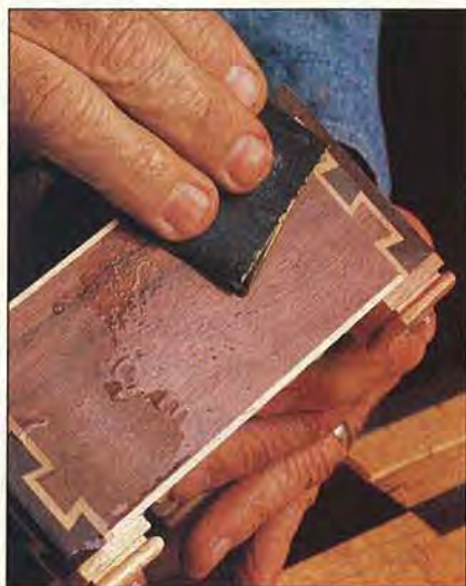
Wet-sanding with 400-grit wet-or-dry paper removes what Arliss calls "orange peel" from the first four coats of sprayed-on lacquer.
