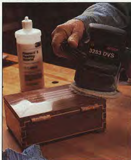
Buffing polishing compound with a random-orbit sander brings out the gloss on the multi-coat lacquer finish.
