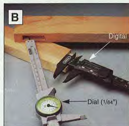
A rod for taking depth measurements is a handy feature. Some calipers will take step measurements between the end of the bar and the end of the sliding jaw.
