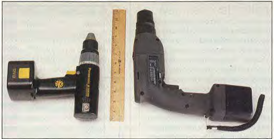
Drills of the same voltage can vary greatly in size. The Panasonic drills (left) were the most compact we tested.
