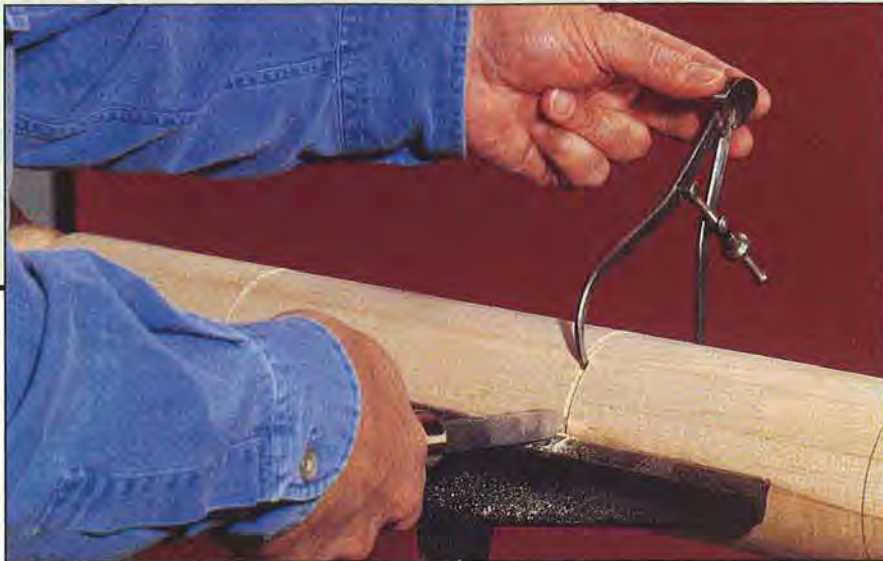
Accurate sizing cuts ensure that the turned legs will be uniform. Carefully set the caliper for each cut, and don't force it over the turning; wait until it falls freely.
