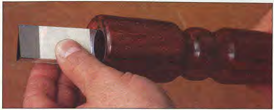
Slide the mirror assembly into the body. It should fit snugly to prevent turning. Slide the mirror assembly into the body. It should fit snugly to prevent turning.
