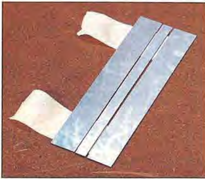
Tape holds the three mirrors in position to fold into a triangle.
