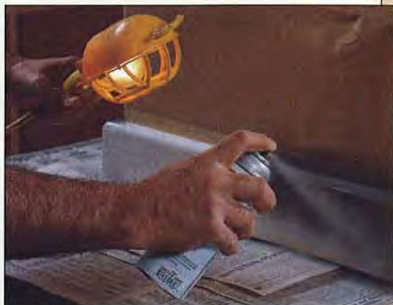
A can of spray paint in one hand and a bright light in the other is a perfect combination for even coats of paint.
