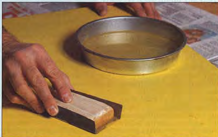
Keeping the project and sandpaper wet, use 600-grit wet/dry sandpaper to sand away imperfections or runs.
