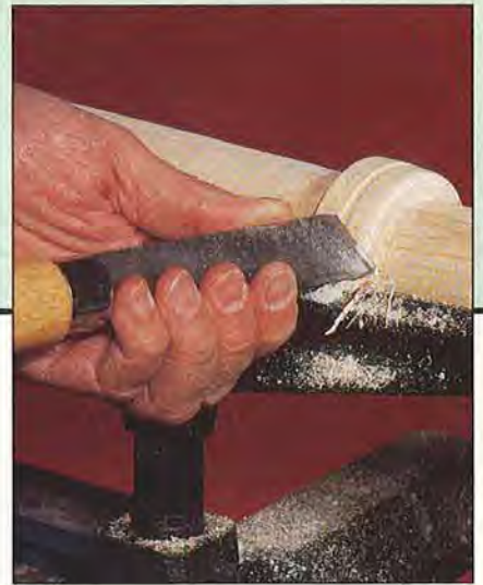
The groove in the middle of the lower bead is the sizing cut which establishes the finished diameter for the feature.
