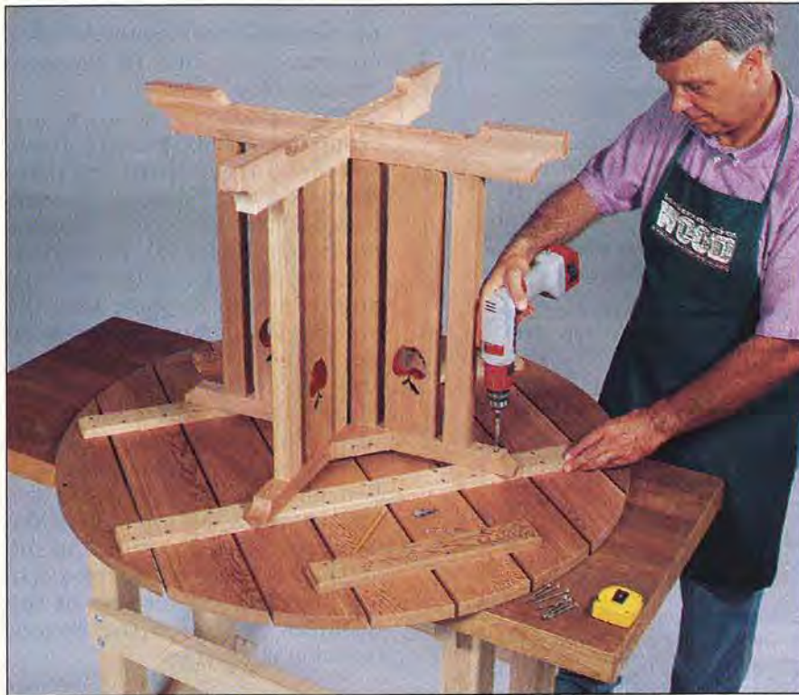
With the base assembly centered on the bottom of the tabletop, glue and screw the two assemblies together.
