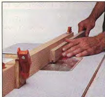
Use your table-mounted router fitted with a fence, stop, and straight bit to rout the stopped grooves.
