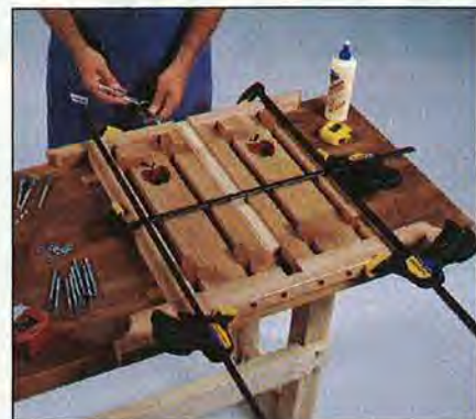
Working on a flat surface and using spacers to establish even gaps, glue, and screw each base half together.
