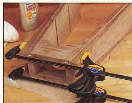
The waste edges ripped from the uprights make convenient pads for clamping the tapered top section.
