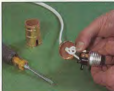
Wrap wire clockwise around terminal screw so tightening the screw draws the wire in.
