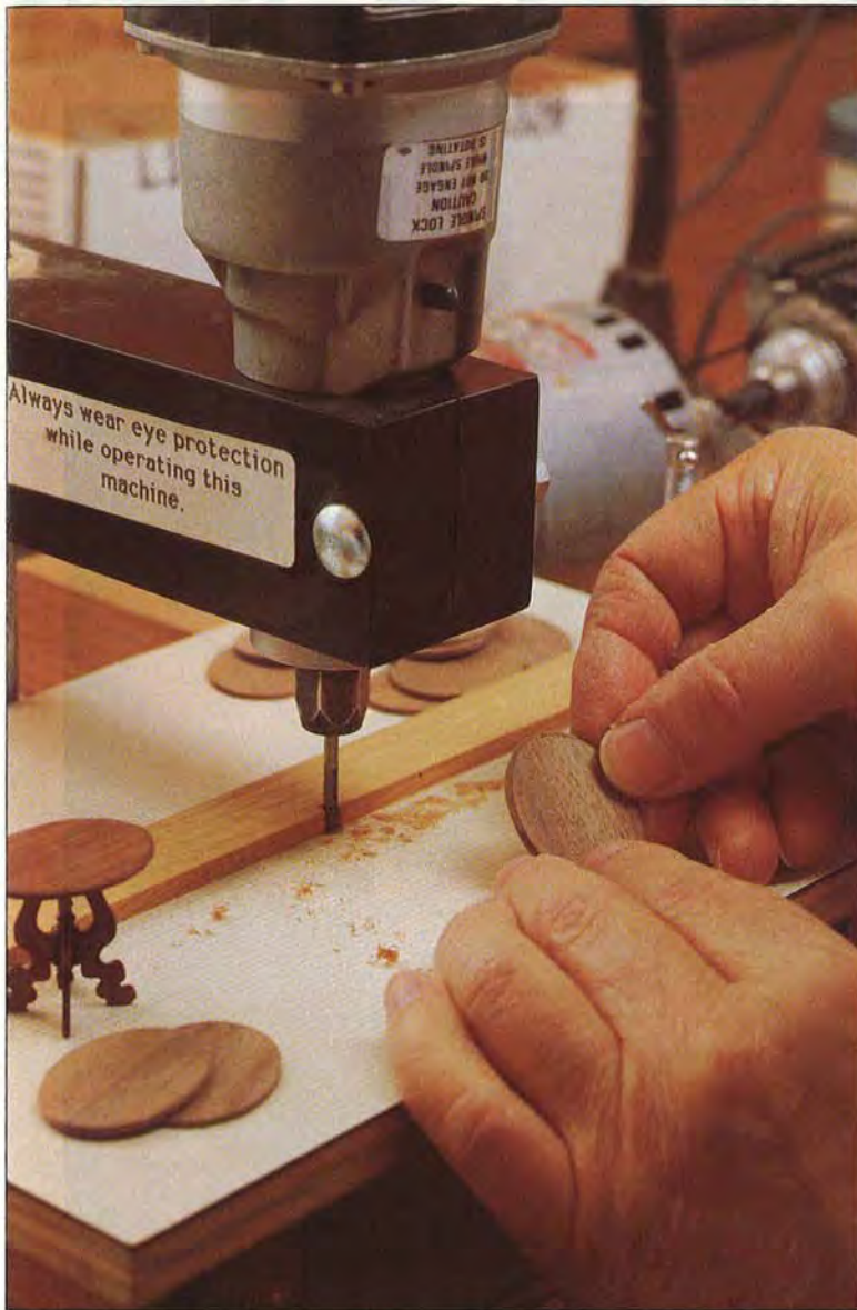
Above: An inverted mini-shaper made from a die grinder contours the edge of a Victorian side-table top. In assembly line fashion, Don will make 310 such tables for a special commission.
