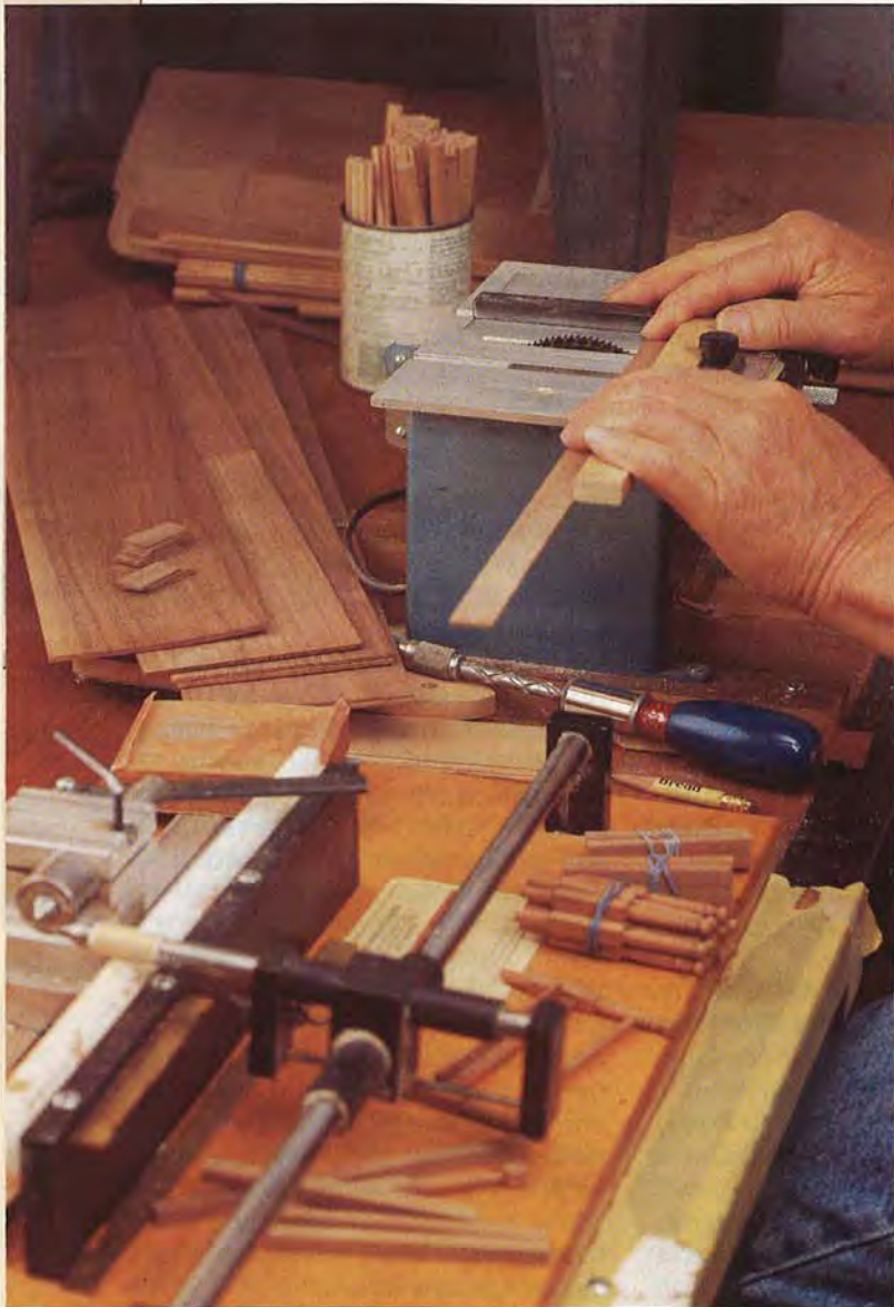
Above: At his Lilliputian tablesaw with its 4" blade, Don crosscuts walnut that he's resawn and sanded to 1/16" thickness. Besides walnut, he regularly uses maple, birch, and cherry.
