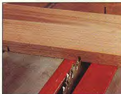
Saw the \frac{1}{4} " shelf dados straight across each upright with the blade tilted to 7^\circ . The dados angle toward the bottom.
