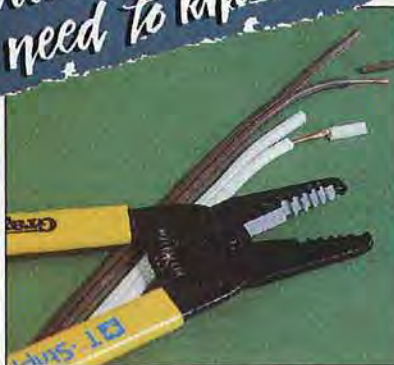
A wire stripper removes insulation from conductor ends easily.
