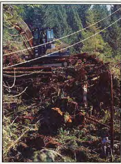
On a clear-cut of Simpson Timber Company land near Korb, California, a swing yarder brings young-growth redwood logs up the slope via a skyline of steel cable. The site will yield about 40,000 board feet per acre.
