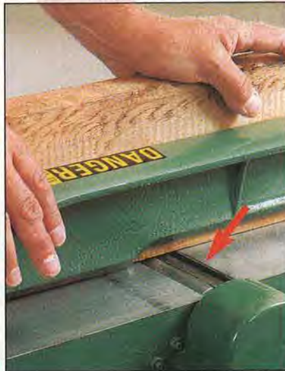
Beware of exposed cutters on some older jointers not fitted with a guard behind the fence.
