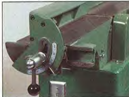
Side-mounted fences, like the one on this General jointer, control the tilt and sliding mechanism from one handle.
