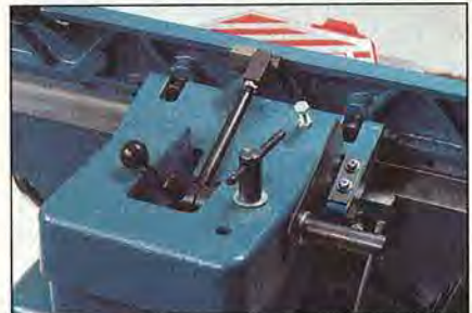
A hinged rod controls the tilt mechanism on the Sunhill jointer.
