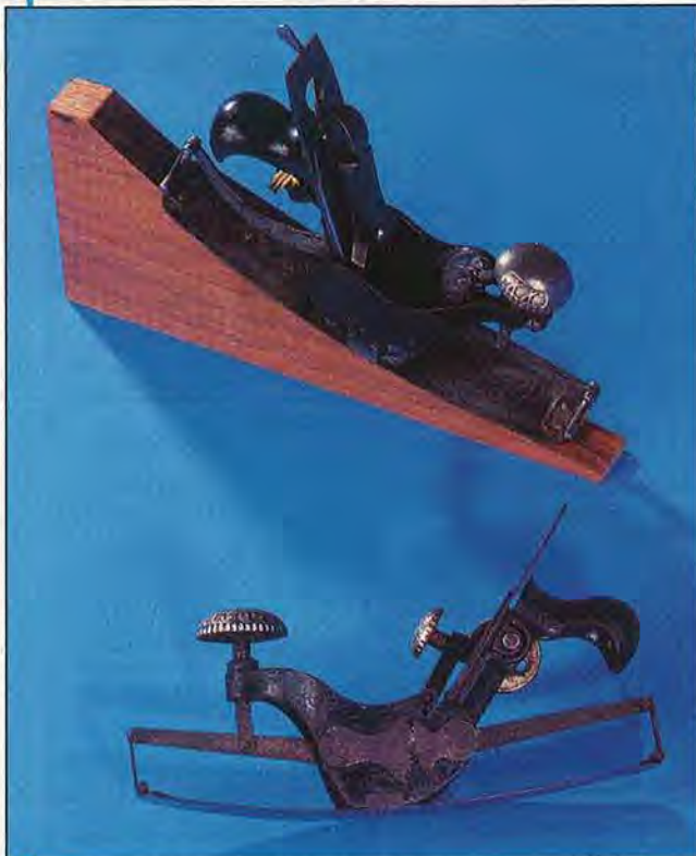
The Stanley 113 compass plane, front, was manufactured in the 1890s. The Keen Kutter K 115, on the wood, dates from the early 20th century.
