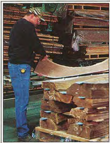
Todd Speicher and a partner load walnut veneer by flitches onto a pallet for shipping to a customer. A pallet may hold up to 20,000 square feet of sliced veneer. Filling one industrial order sometimes requires 40 of those pallets.
