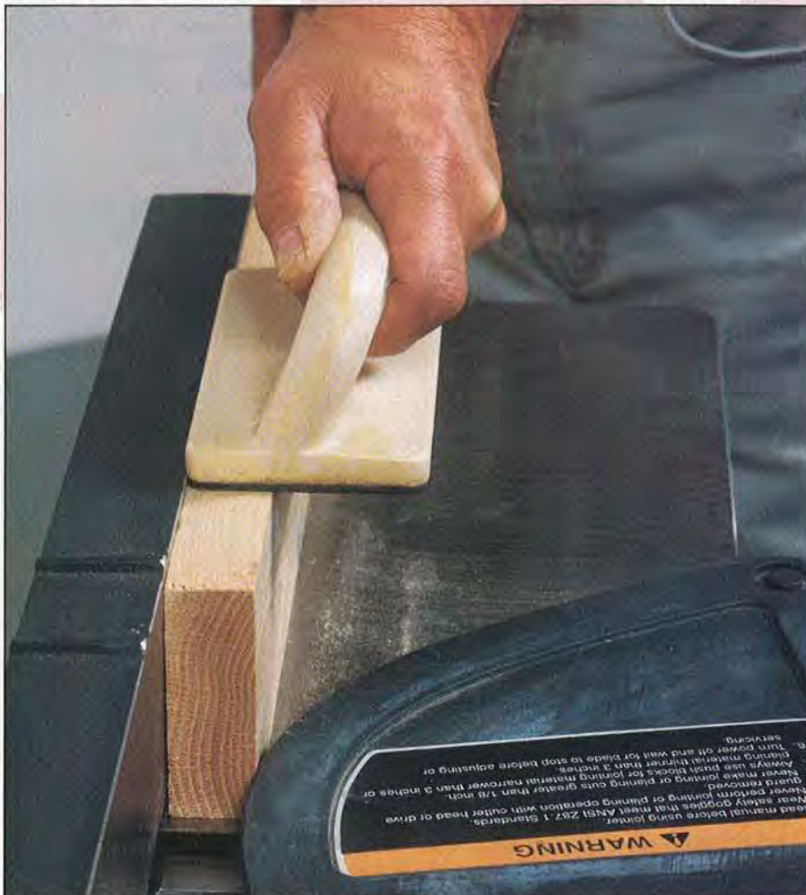
For safe jointing, use pushblocks to keep hands and fingers out of the cutters' way.
