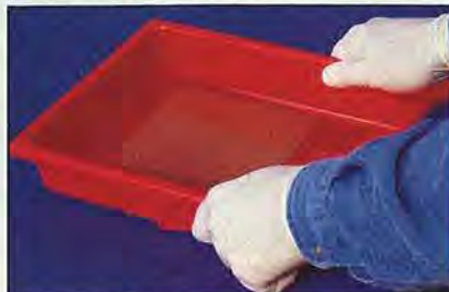
Gently rock the tray from side to side and end to end while aging copper in photographic rapid fixer.
