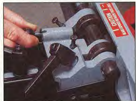
To maintain an accurate stop, the Delta fence uses a spring-loaded pin that locks into a tapered groove in the collar attached to the large rod on the fence.
