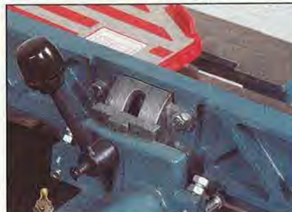
The fence on the Jet jointer tilts on a curved bracket bolted to the backside of the fence.
