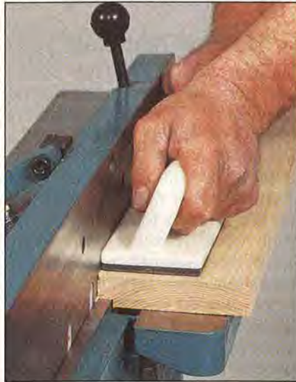
Jointers cut rabbets faster than routers, but you must remove the guard first.
