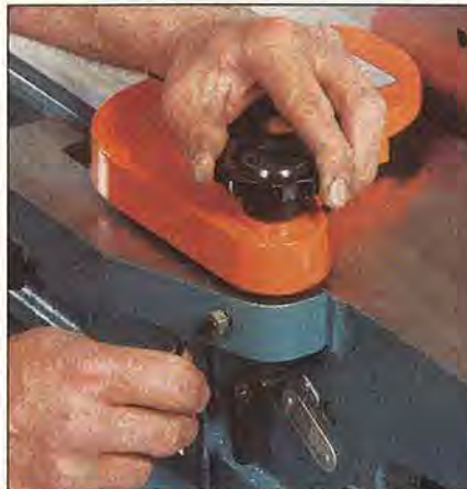
To set the guard tension on the Enlon jointers, all you have to do is turn the knob and tighten the set screw.
