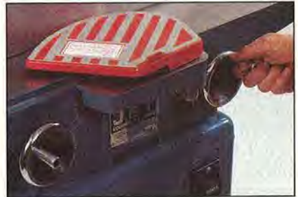
Mounting handwheels on the front of a jointer makes them much easier to grasp and turn.
