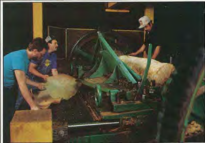
Some woods produce more figure when rotary cut, as is being done with this big-leaf maple log turning against the knife. The veneer will feature a desirable quilted figure. Because of the log's uneven shape, it first produces small, irregular sheets.
