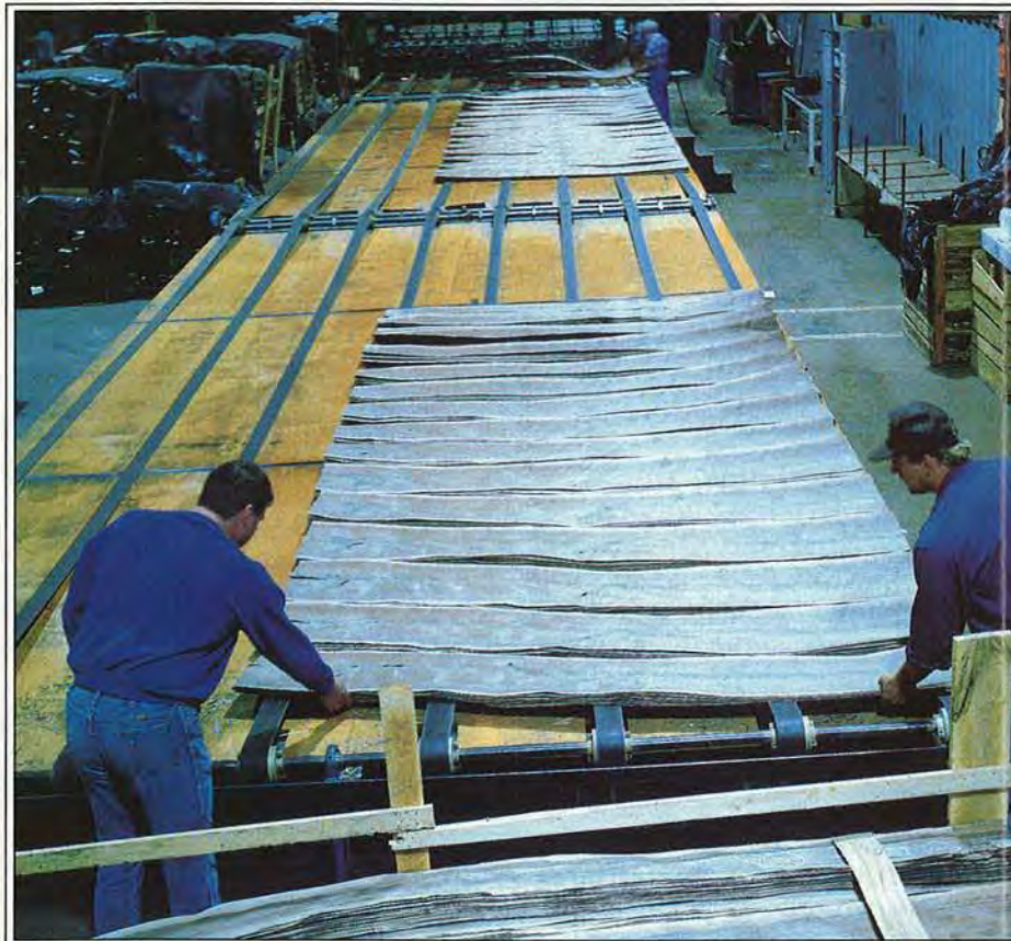
Sheets of walnut veneer, kept in order as they were sliced off the flitch, creep down the conveyor from the dryer. Pressing and banding further flattens them.
