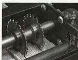
New rip saw attachment lets you gang-rip with power feed in a fraction of the time it takes for multiple hand-fed passes on an ordinary table saw.
