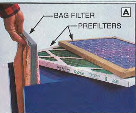
The Hartville Tool unit has one more prefilter than the other tested machines. We found it unnecessary.
