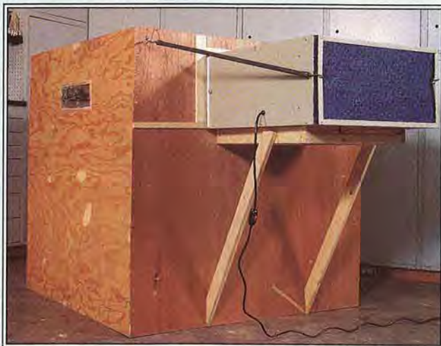
We built a plywood test chamber and used it to subject each air-filtration unit to equal amounts of dust.
