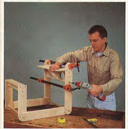
Clamp the seat and desk support assemblies between the side frames, drill pilot holes, and drive the screws.
