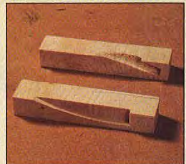
The top photo displays the difference between the short, straight pocket hole made by a conventional jig and the longer, curved hole made by the motorized Porter-Cable model.
