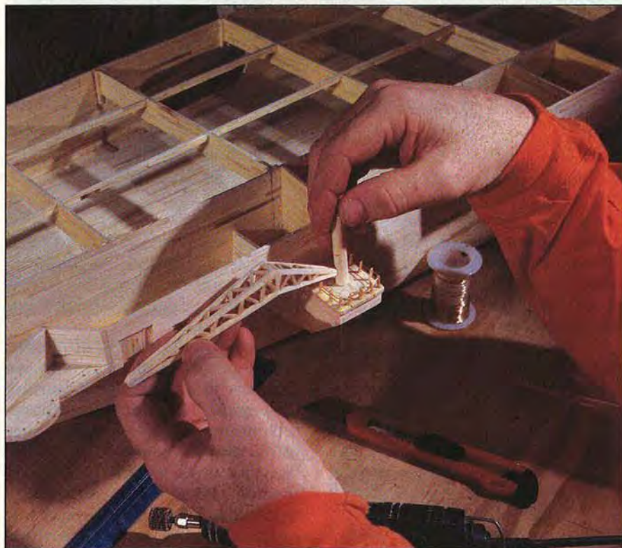
Before mounting the crane, Pat strung hair-thin copper wire through holes he drilled in stanchions made of...you guessed it, matchsticks.
