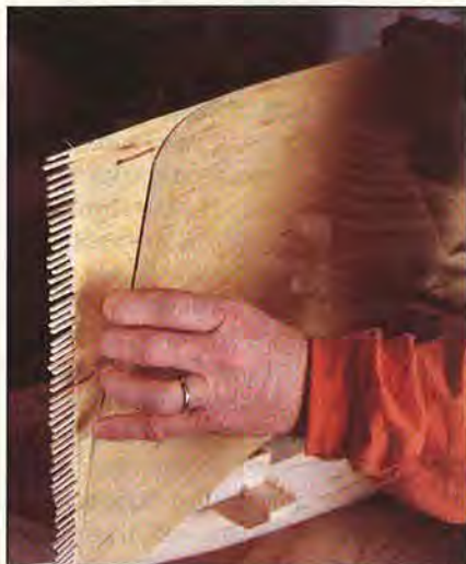
For carrier decks and other flat expanses, Pat uses sheets of glued up matchsticks. The acrylic sheet easily peels off.
