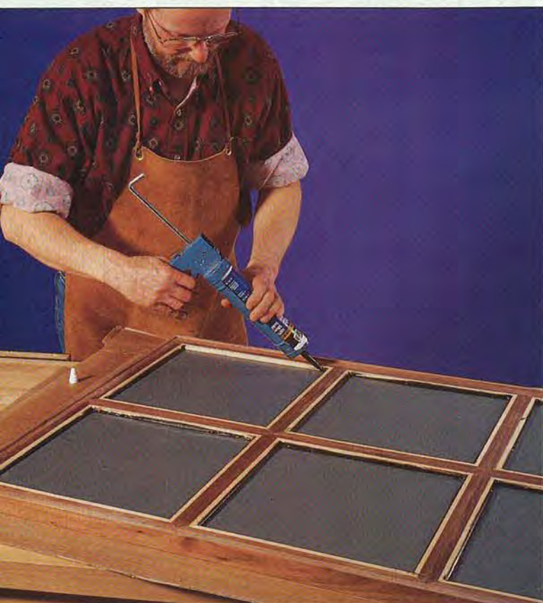
Apply a bead of silicone sealant around all edges of each mirror to hold them in place.
