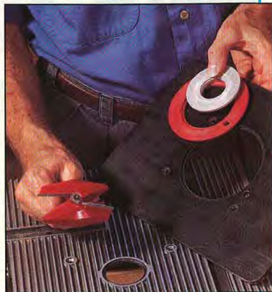
When your router bit doesn't fit in a metal table, you can run it above the tabletop. In a wooden table, use a router-table plate with inserts like those held above at right.
