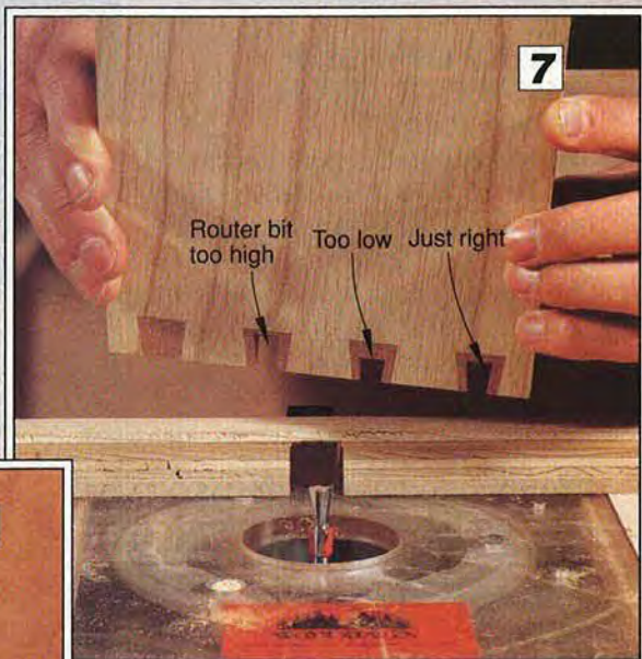
Working with scrap stock, adjust the height of the cut for the second key as shown here.
