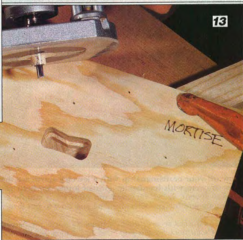
Occasionally vacuum debris from the mortise as you rout it to prevent chips from interfering with the cut.
