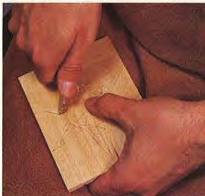
Move your thumb to the back of the blade for the second position.
