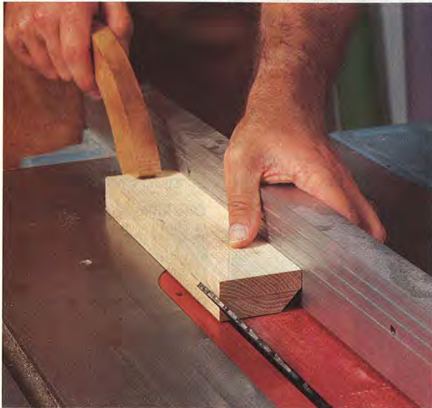
Bevel-rip the edges of the laminated-ash mallet-head blank at 45°.
