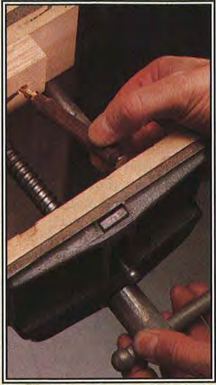
Press fittings into tubes with a vise. Wood block shown here prevents damage to applicator nib.
