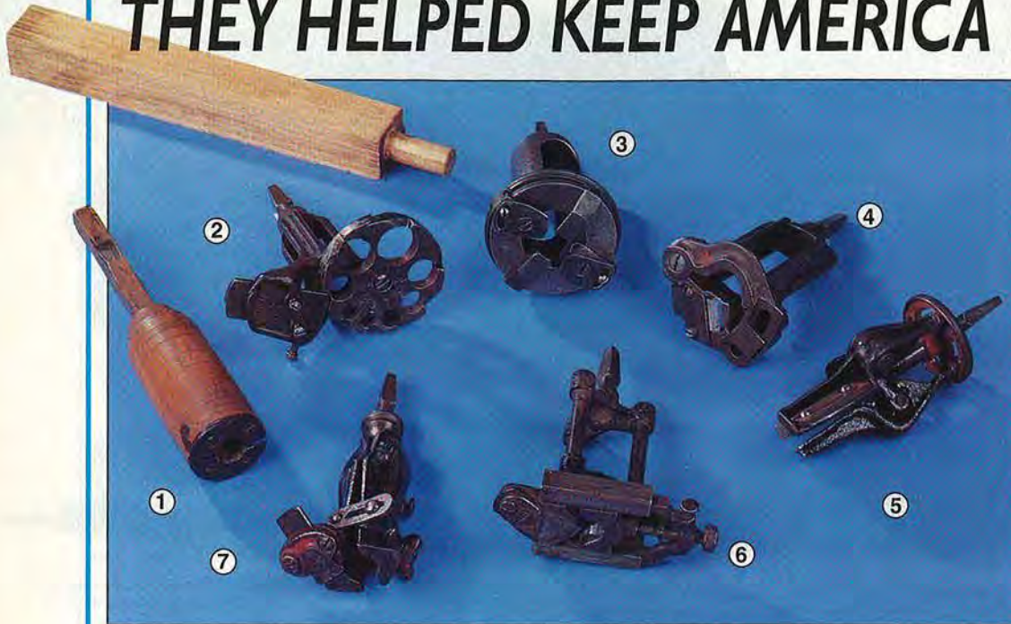
The wooden hollow auger, no. 1, cuts one tenon size. Adjustable types shown include: Bonney, 1870, no. 2; Cushman, 1870, no. 3; Wood, 1875, no. 4; Stearns, 1877, no. 5; Wood, 1900, no. 6 (Wood patented five types of hollow augers); Stearns, 1878, no. 7 (Stearns held patents for seven hollow-auger designs).
