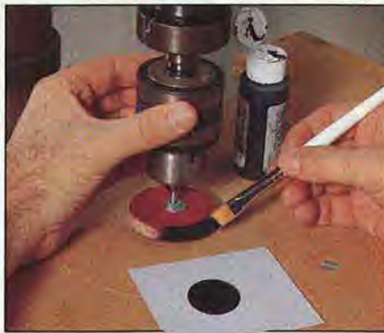
Secure a wheel on a bolt in your drill press. Turn the chuck by hand to paint the black on the wheels.
