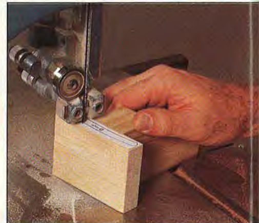
Use a scrap block to support the roof blank when cutting the roof to shape.
