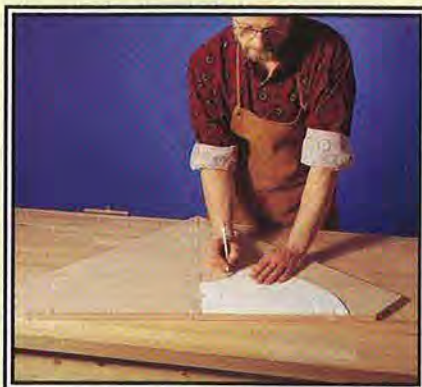
Transfer the full-sized shelf half pattern to poster board and use it to mark the front edge of the top two shelves.
