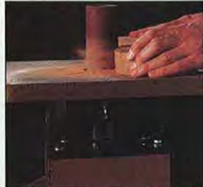
Hooked to a 3-hp shop vacuum the Powermatic 14 collects most, but not all, sanding dust.
