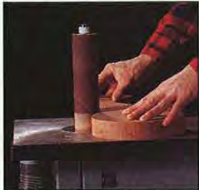
The Clayton model 146 spewed almost no sanding dust into the air during our tests.
