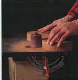
With no provision for dust collection, the Vega OS-3 produces a cloud of fine debris.
