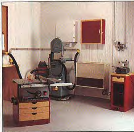
Above: The shop vacuum, from its position in the right corner of the shop, collects dust from a run of clear-plastic pipe. With a mobile base, the bandsaw can be positioned anywhere in the shop. Above the heater is the enclosed exhaust fan. The compressor hose connections are for spraying.
