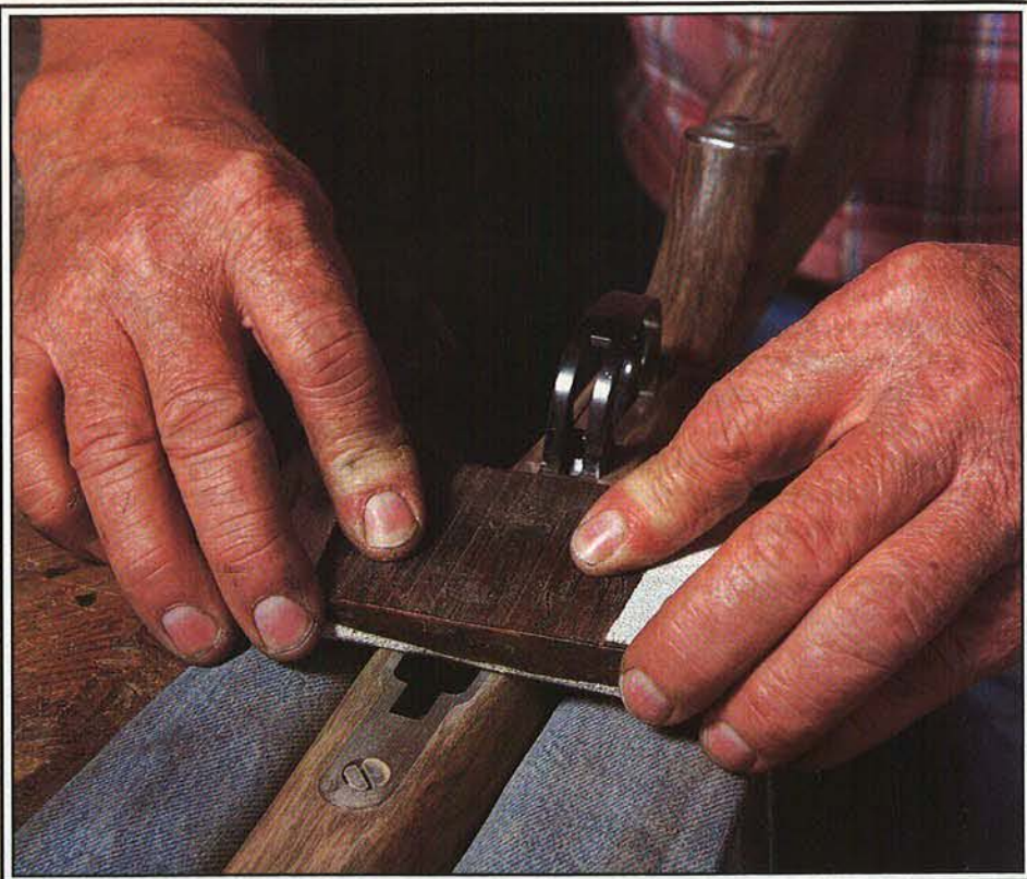
Having fit the metal into the wood, Bud brings the two flush with careful sanding.
