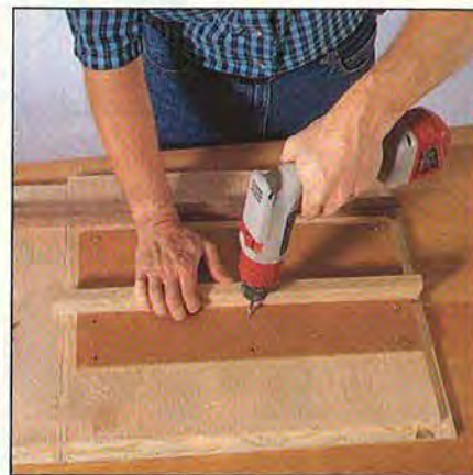
For evenly spaced tray supports, use a piece of \frac{3}{4} "-thick stock to position the pieces before screwing them in place.
