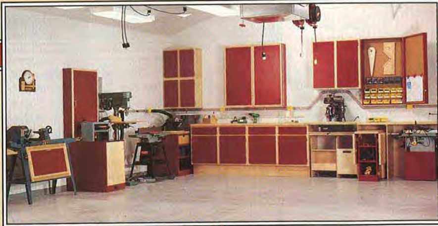
Above: The sander, jointer, drill press, and planer find homes in the far-left corner of the shop (see floor plan). The lockable cabinet stores drill bits and other accessories. The sander and planer bases were shop built.
