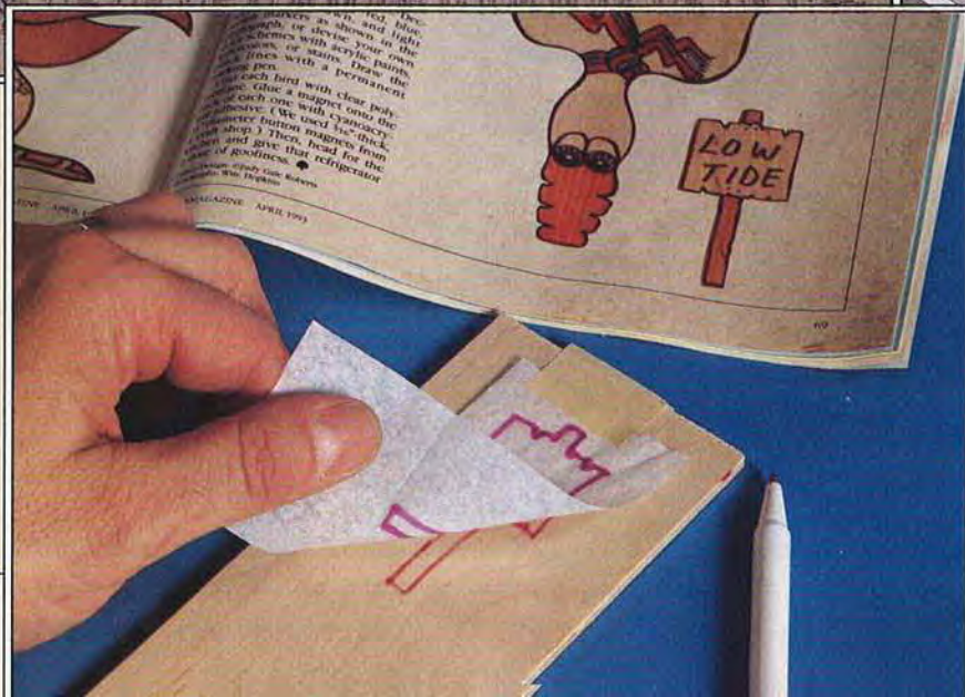
Left: This disappearing fabric marker works great on light-colored woods. The ink soaks through the tissue to mark the wood beneath. The lines fade away within a day.
