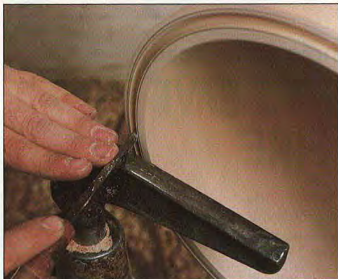
Initially turn a thick-walled bowl— \frac{1}{2} " or thicker. As you cut the groove into the rim, taper the sides to match the ring.
