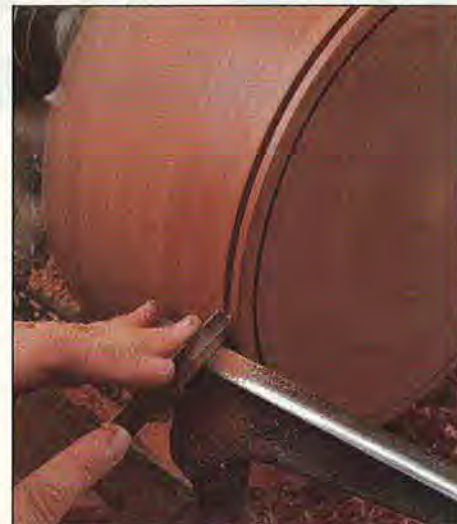
Cut into the face to set the ring's width. Then, cut from the side to establish thickness and release the ring.
