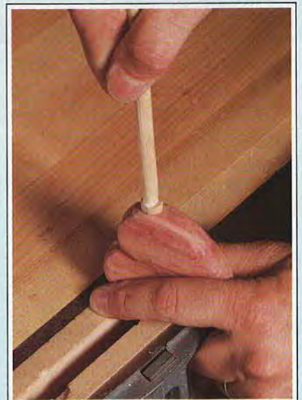
Whittle away the corners of the compressed end until it will just fit through the hole in the heart.
