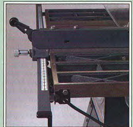
The angle-iron rails on the Sears saws required regular fine-tuning.
