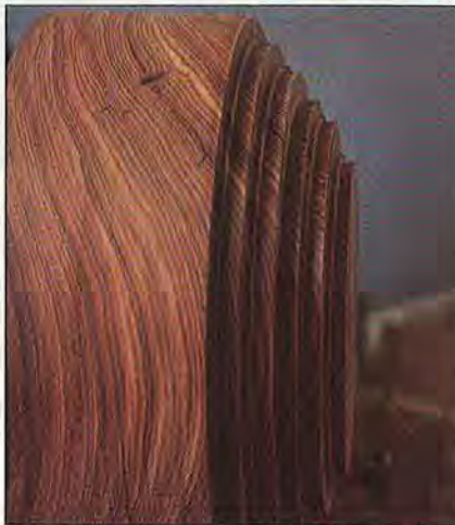
Removing rings from a blank helps rough out the shape for a bowl without piling up a lot of waste chips.
