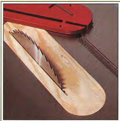
You'll need a factory throat plate at least 1/8"-thick to make your own plywood zero-clearance inserts.
