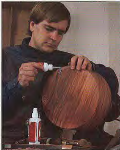
Lane Phillips glues hairline cracks with cyanoacrylate adhesive before beginning to cut rings from the blank.
