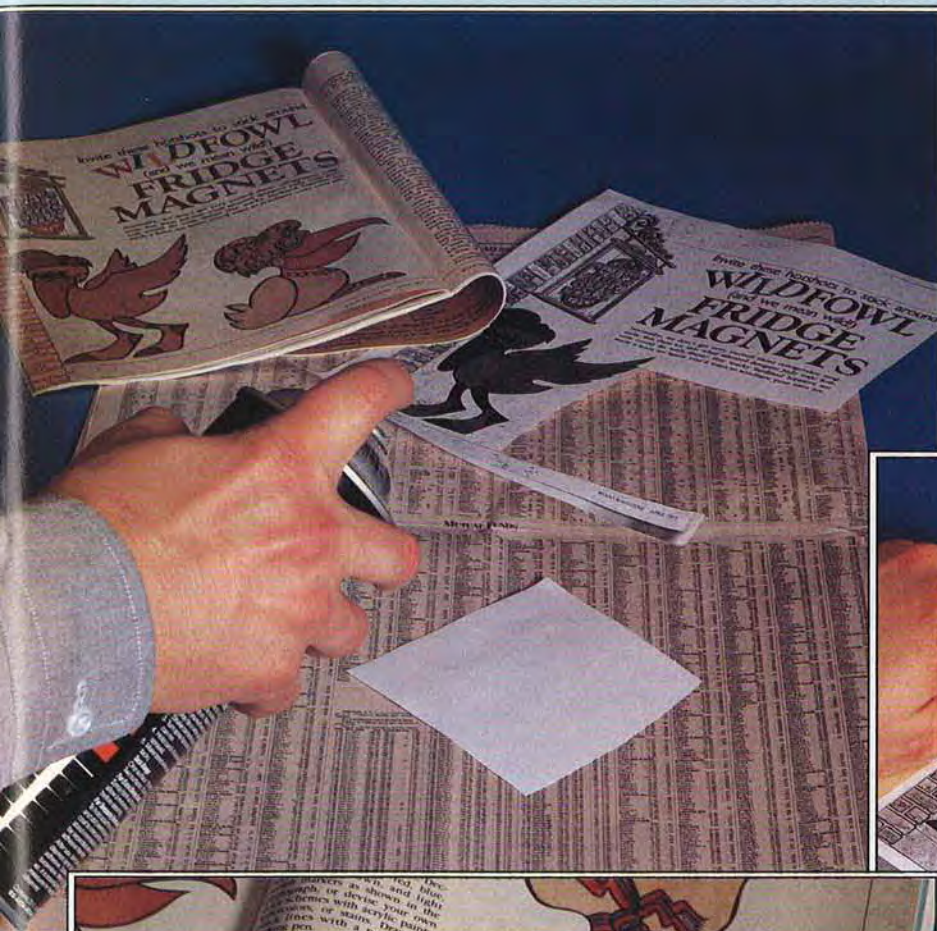
Left: Spray an even coat of adhesive on the back of the pattern. Lay the pattern on newspaper so you can spray all the way to the edges.
