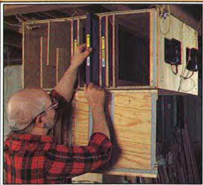
Al traps airborne dust particles with his shop-made particulate cabinet .
