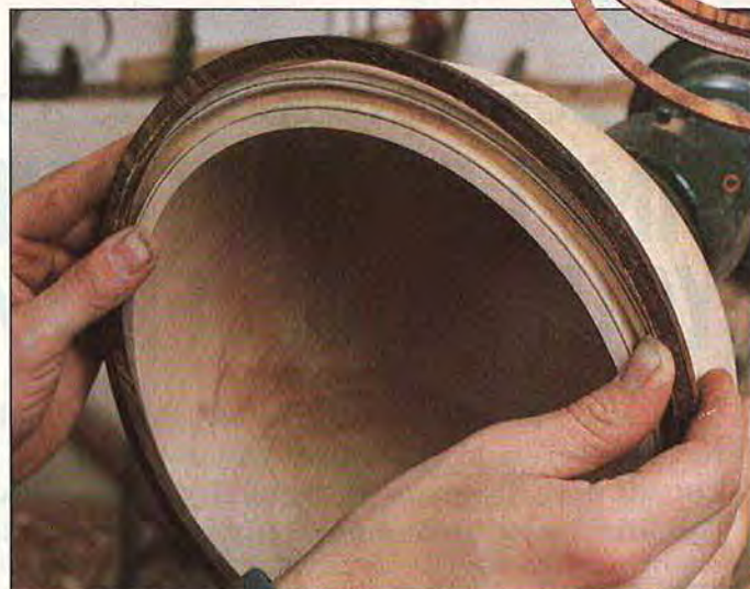
Test-fit the inlay in the groove frequently as you work. The ring must fit tightly, but need not be flush with the rim.
