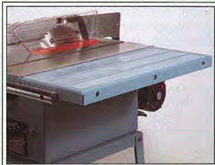
Formed-steel extensions on Delta's saws won't pinch fingertips.
