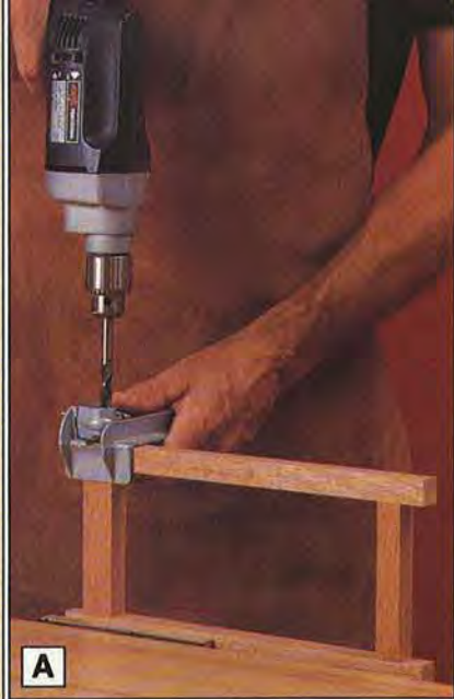
Using a doweling jig for alignment, drill a \frac{3}{8} " dowel hole at each butt joint.
