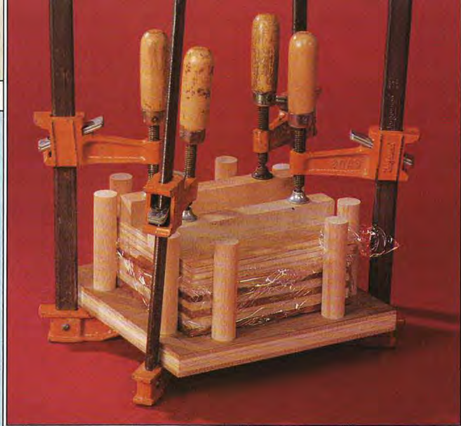
The gluing jig helps keep the edges aligned as you build the lamination. Make sure the jig posts stand perpendicular to the base. A plywood square and scrapwood bars distribute the clamp pressure to ensure a tight lamination.
