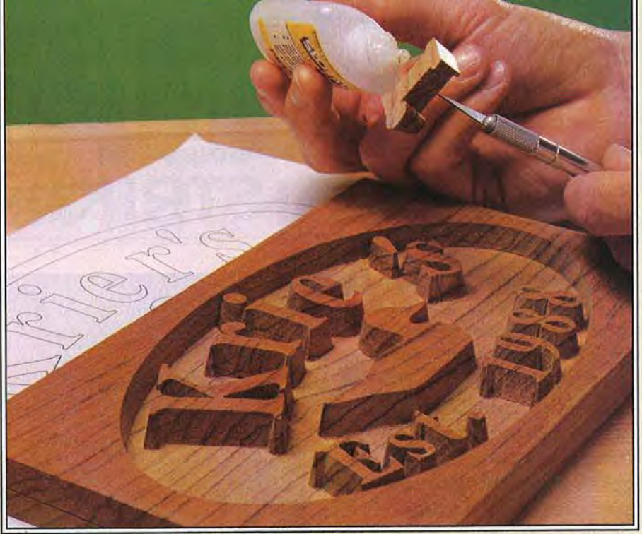
When applying adhesive, use an X-acto knife to pick your characters off the resawn surface. Orient the knife blade with the grain to avoid marring the workpiece.
