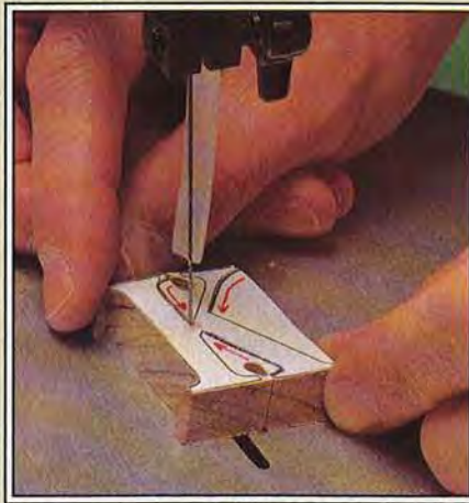
Cut just one side of tight corners (as shown by the arrows), and then tilt the table and cut the other side.
