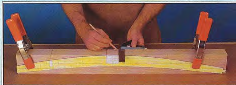
Transfer the mortise location, dowel-hole centerline, and leg outline to the rear leg blanks from the template.
