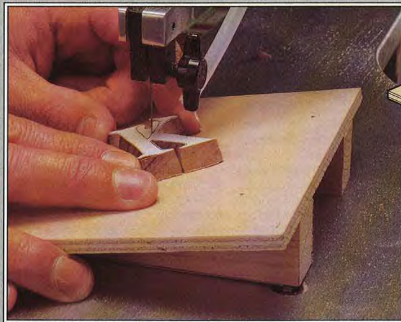
No matter what scrollsaw you use, this simple 10° auxiliary table helps you make beveled cuts in any direction.
