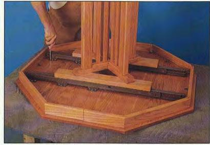
Attach the metal slides to the slide supports (I) and then secure them to the bottom of the tabletop halves.
