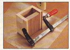
Secure the mitered joints together with masking tape when gluing the pieces. The spacer holds the pieces square.
