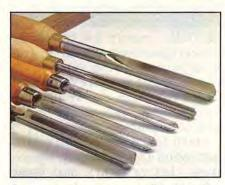
Gouges are the most versatile of turning tools. In fact, you could turn a spindle or a bowl with no other tool than a gouge. The flute depth, bevel angle, and end shape distinguish the three different types. Shown from left, the roughing gouge, used to round square stock for spindle turning, two spindle gouges, and two bowl gouges.
