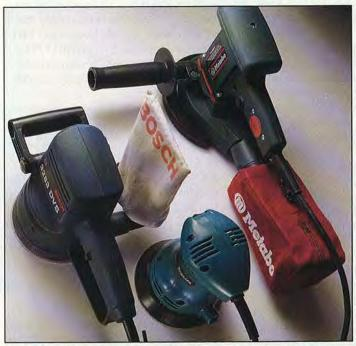
Each of these in-line sanders has a different handle style; from left: The Milwaukee 6126 at right has an auxiliary side handle Bosch 3283DVS with front handle, Makita BO5000 with palm handle, and Metabo 0125 with side handle.
