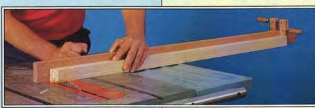
Fasten a long auxiliary wooden fence to your miter gauge, angle the blade 10° from square, and angle-cut the top end of each corner post. Use a clamp attached to the fence for a stopblock.
