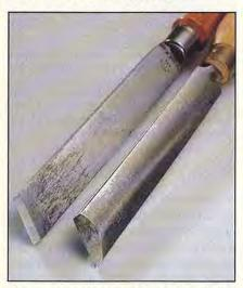
Above, compare the standard skew's flat sides and sharp corners to the oval skew's blade. Many woodturners find the oval skew easier to handle. Skews, like all turning tools, must be sharp.
