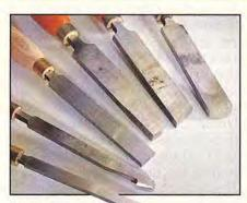
Scrapers, mostly used in faceplate turning, come in a variety of sizes, shapes and styles. Typical scrapers include, from left, roundnose, diamond side-cutting, straight, half-round, skew, and domed. Thicker, heavier scraper blades provide a smoother turned surface by reducing chattering.
