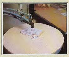
Here, the cutting platform with the tiny \%" zero-clearance blade hole gives nearblade support to delicate silhouette details. Roy cut away some of the waste area to expose the blade hole.
