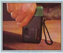
For an accurate reading with an electronic moisture meter, push the meter's probes into the wood at the center of the board, not at the edge or end.
