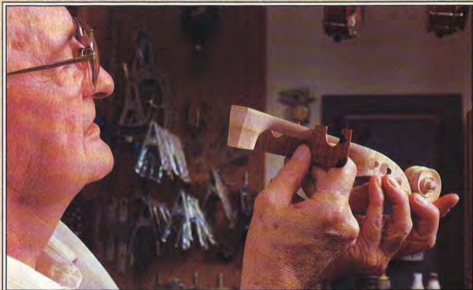
▲ Bill sights along a violin neck to check it for straightness. With the small
