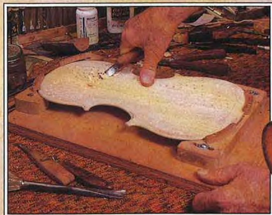
Spruce tops can be hand-carved to thickness, such as Bill is doing here, but hard maple requires machine tools.
