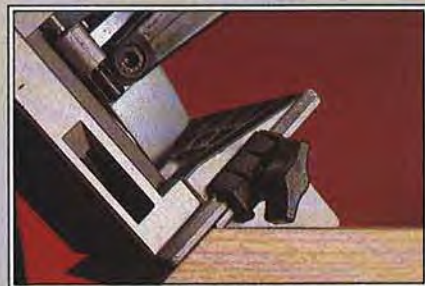
The fences and faceplates of the Skil and Freud (shown here) give you little control when joining beveled edges.
