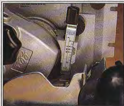
The Elu 3380 has a fully adjustable depth-of-cut scale.
