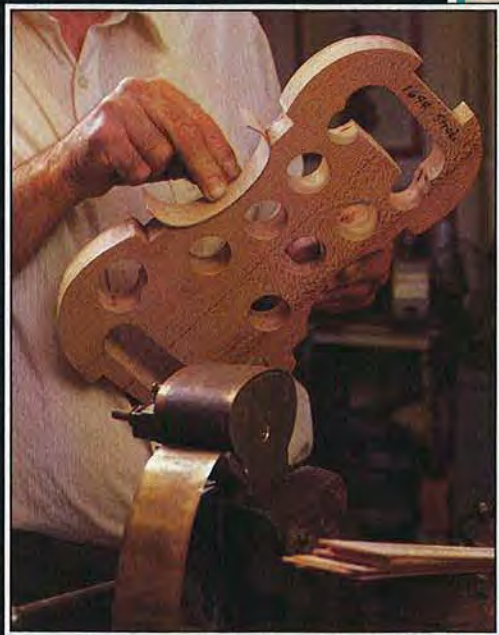
◀ Bill built the heated shaper (in the foreground) that he uses to curl the violin's sides, or ribs.
