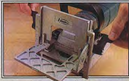
You can change the height and angle of the fence on the Virutex AB-11 in seconds by flipping two levers.
