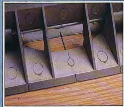
To cut a slot, first align the biscuit joiner's mark with the mark on your workpiece. Then, plunge in the blade.
