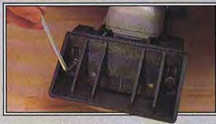
To reposition the fence on the Skil 1605:02 you have to loosen two screws with an allen wrench.
