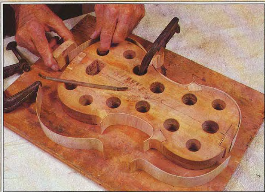
◀ Bill built the heated shaper (in the foreground) that he uses to curl the violin's sides, or ribs.
