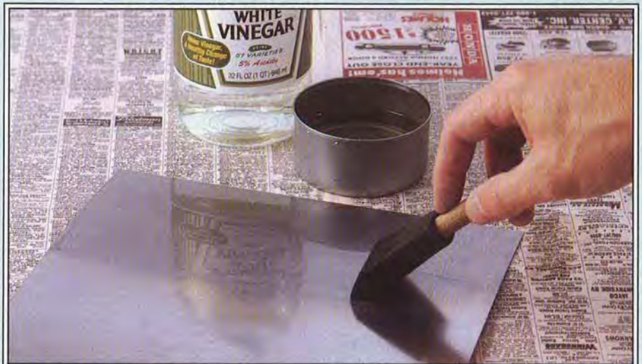
For an evenly aged panel, generously apply the vinegar in quick, overlapping strokes. Be careful not to allow vinegar to leak onto the opposite side of the panel.
