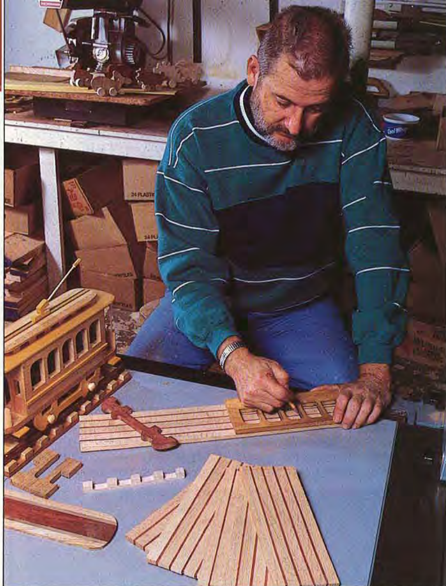
Hank uses templates to help him lay out the parts for a trolley car. With track, his trolley will bring $125.
