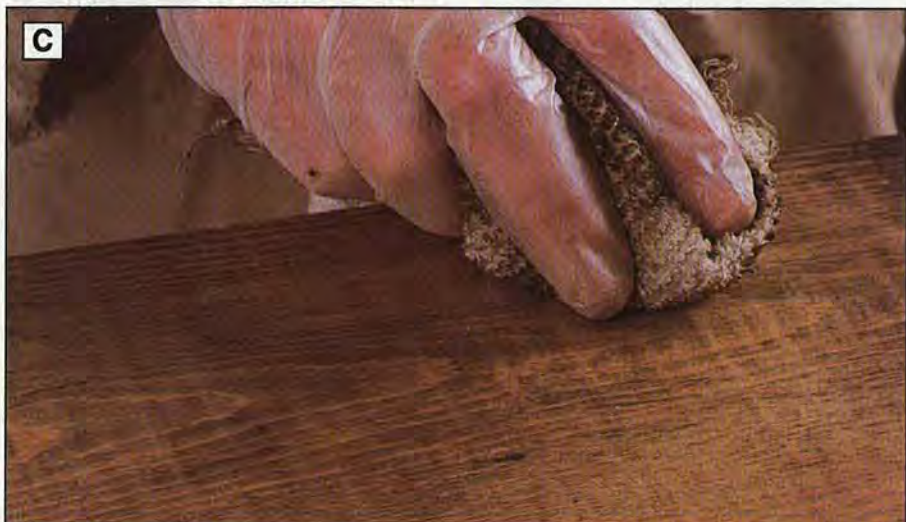
Before the stain dries, lighten any high-wear areas with paint thinner. Don't forget to wear the protective gloves.
