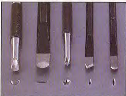
A sampling of specialty punches and the holes they make. From left: C chisel, curved chisel, star punch, willow punch, and lampmaker's chisel.
