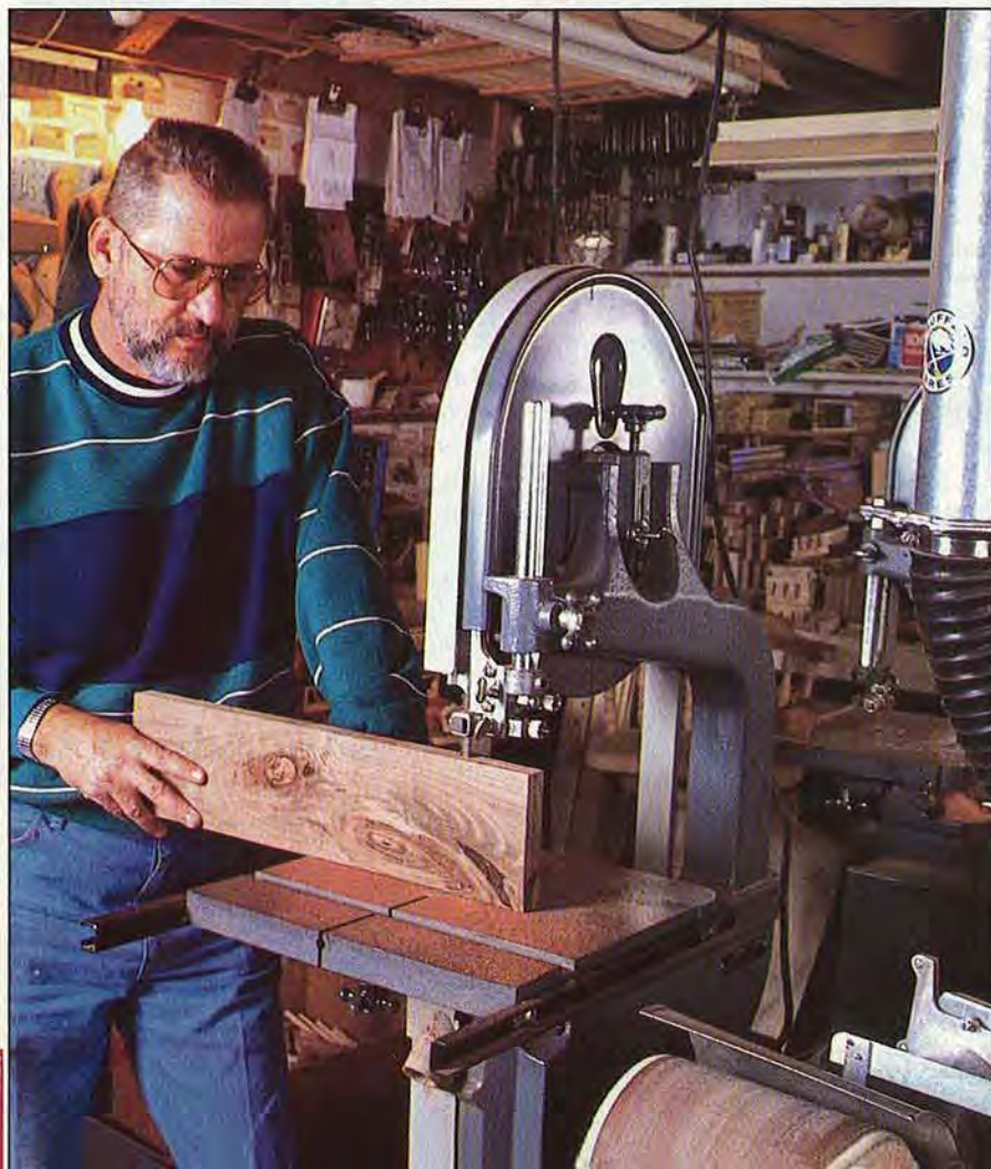
Left. Hank resaws all his wood at the bandsaw minus its fence, a technique WOOD magazine can't recommend. He believes that he gets a straighter cut.
