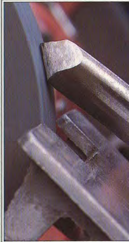
Touch the heel of the bevel to the grinder first, then ease the toe into the wheel before grinding the entire bevel. This helps you avoid burning the edge.
