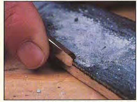
To polish the inside surface of a V-tool, pull it along the strop's edge.
