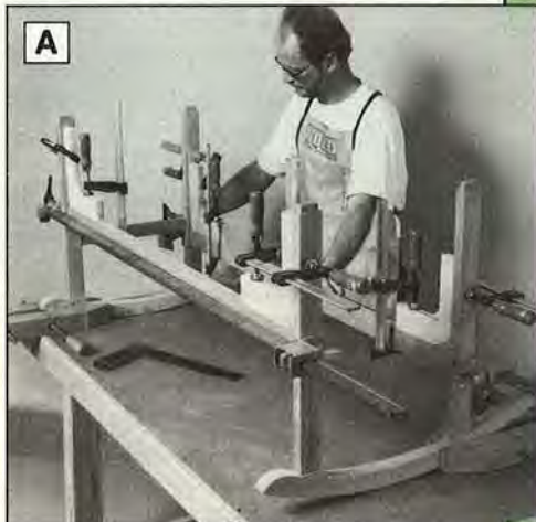
We used 90° corner braces to hold the rocker frame pieces square while the glue dried.
