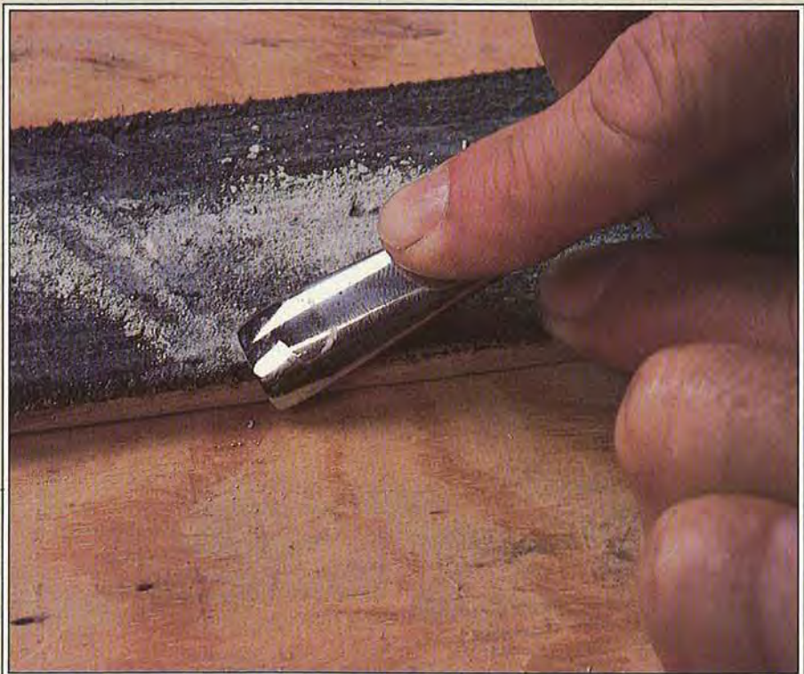
Roll the concave side of a gouge as you pull it along the strop's edge. For each stroke, roll the tool completely from one corner of the edge to the other.
