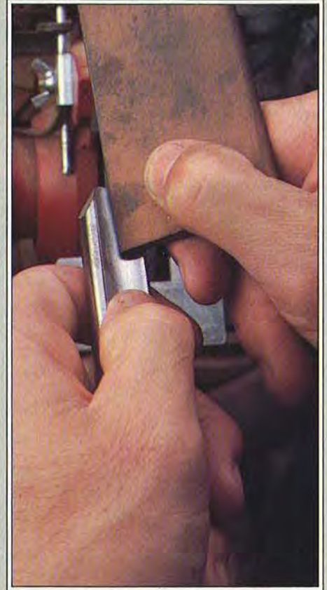
With a slipstone you can quickly remove the burr from the edge of a gouge.
