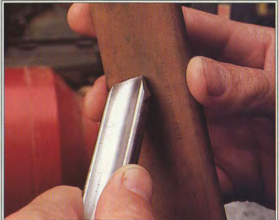
Stroke the tool's bevel several times with the flat side of a slipstone.
