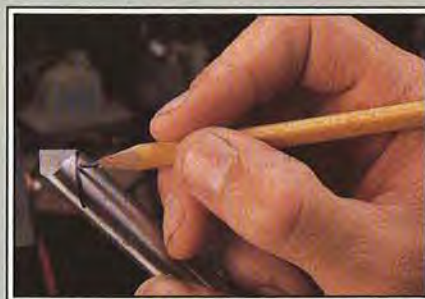
Before grinding, mark the tool's new profile with a pencil.
