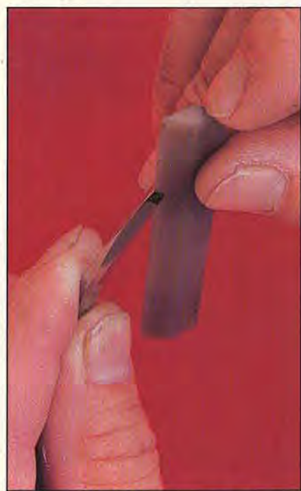
A slipstone with a fine point helps you deburr the inside edge of a V-tool.
