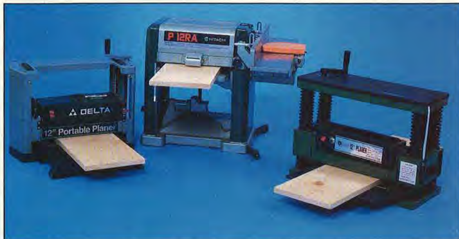
We tested these three new entries in the portable-planer market (from left): Delta 22-540, Hitachi P12R (shown as model P12RA with attachable 6" jointer), and Grizzly G1017. All three machines plane 12"-wide boards.
