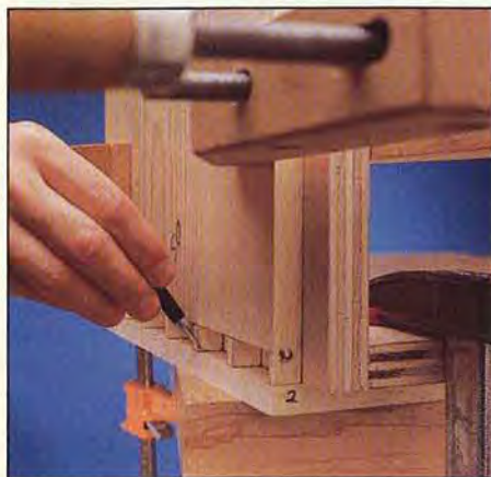
Clamp the workpieces to the bracket for accurate tail marking.
