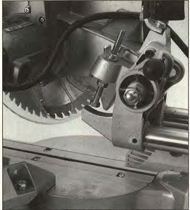
An easy-to-adjust depth stop is just one of several well-designed controls on the Hitachi C8FB.
