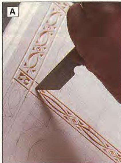
A. The stab knife leaves a triangular impression when forced straight into the wood.
