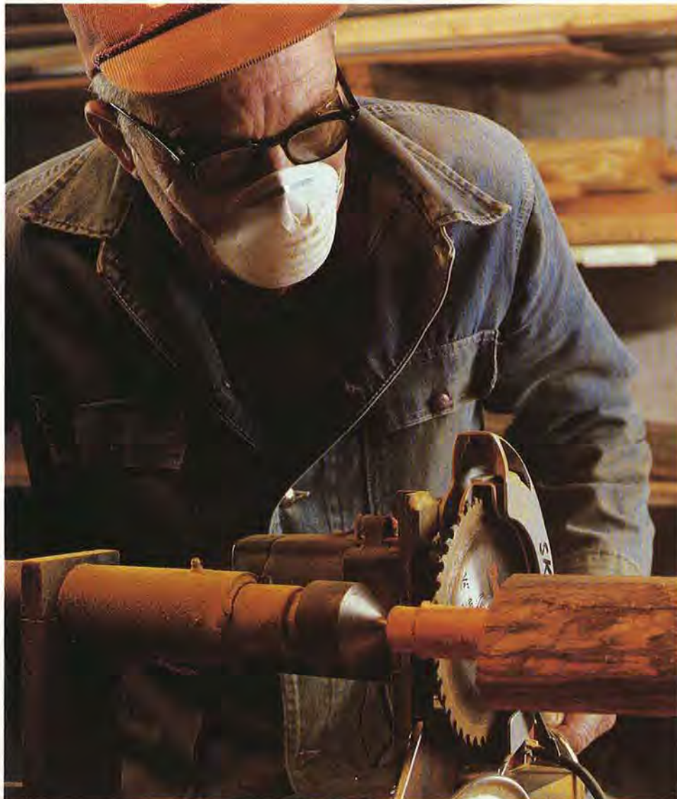
Because the hard hedge would quickly lay waste even the best carbide turning tools, Bud saws the round tenons at his lathe.
