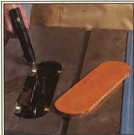
For best results, allow the hotmelt adhesive to cool for 10–15 seconds before putting the insert in place.
