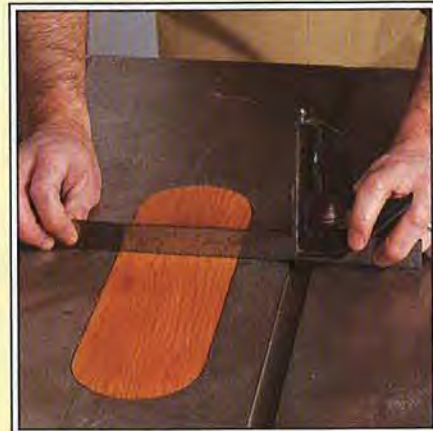
Before the hotmelt adhesive cools completely, set the insert flush with the table top using a straightedge.
