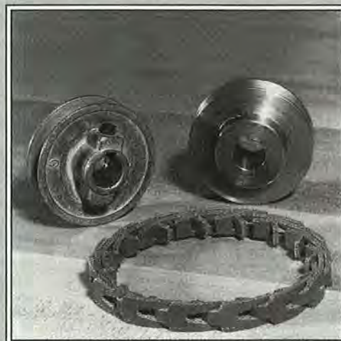
We reduced the vibration in our table-saw by replacing its cast pulleys ( left ) with turned pulleys ( right ), and adding a link belt.
