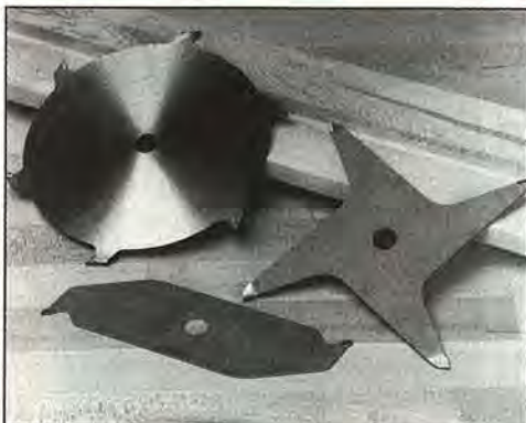
Most chippers have two carbide teeth, but Forrest and SystiMatic make four- and six-toothed chippers, respectively.
