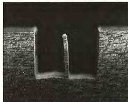
Both of the steel, hollow-ground sets we tested—the Sears 32177 and Vermont American 26747—left a tiny ridge when cutting a ¼”-wide dado (no chippers).
