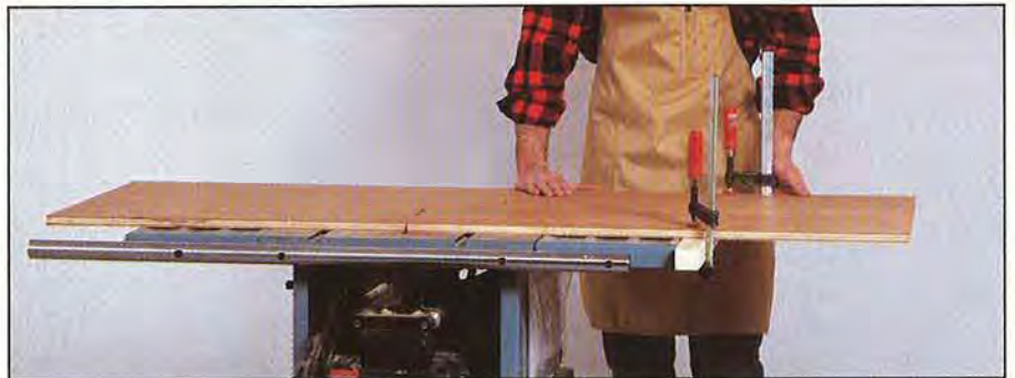
A straightedge clamped to the bottom side of your workpiece helps you crosscut long panels quickly, easily, and accurately.
