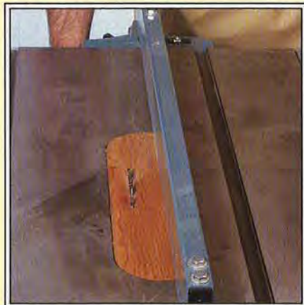
Hold down the insert with your rip fence and slowly raise the blade. Be careful not to cut into the rip fence!
