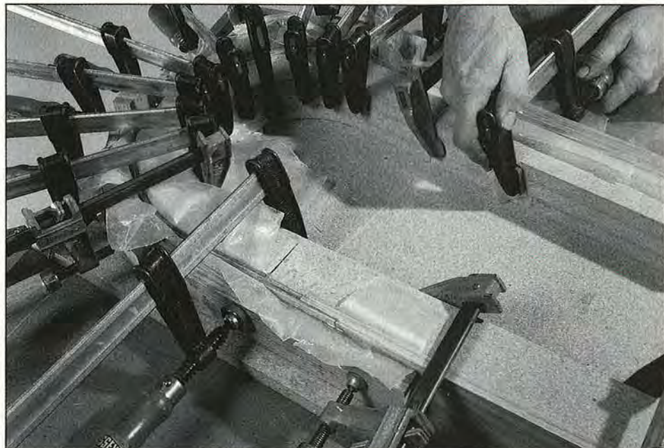
Epoxy and clamp the thin ash strips to the straight rabbeted runner and then
