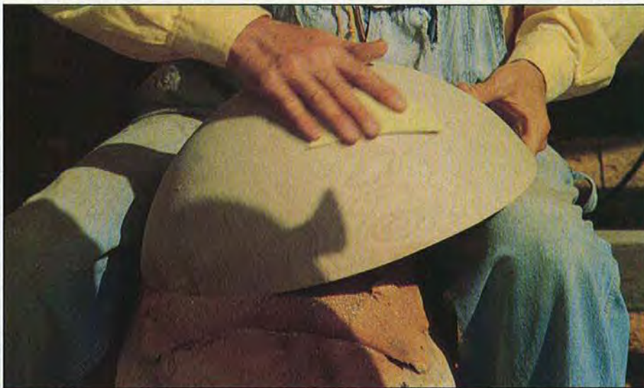
After belt-sanding, John hand-sands with 320-grit paper for super-smoothness, all the while taking off tiny high spots that his hands notice.
