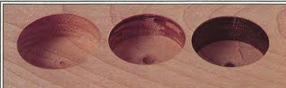
We came across the good, the bad, and the ugly of burned walls in our tests. Holes resulted from left: CONVALCO, Chinese-made, and West German-made Forstner bits.
