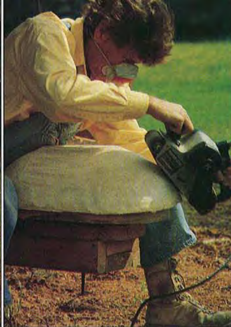
Grinding, then sanding, removes all the saw and adz marks from the bowl, as well as fine-tunes the shaping.
