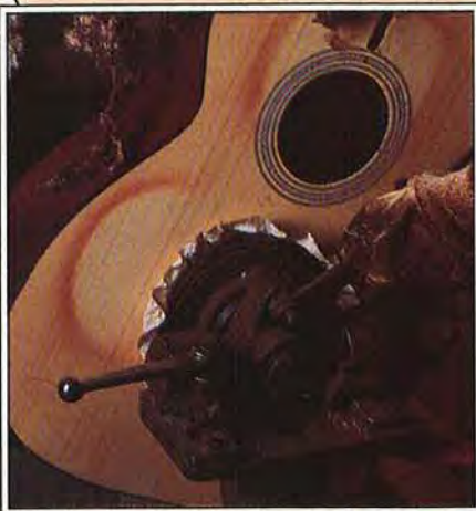
A vacuum clamp holds the guitar in position so walnut-colored filler can be rubbed into the back and sides with a soft cotton bun.
