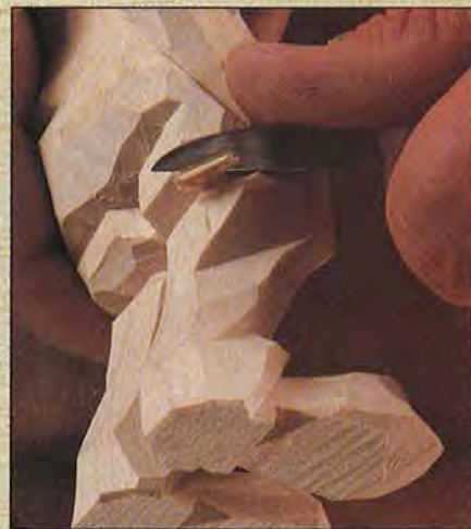
One cut down and in, another up and in make a fold in the cloth.
