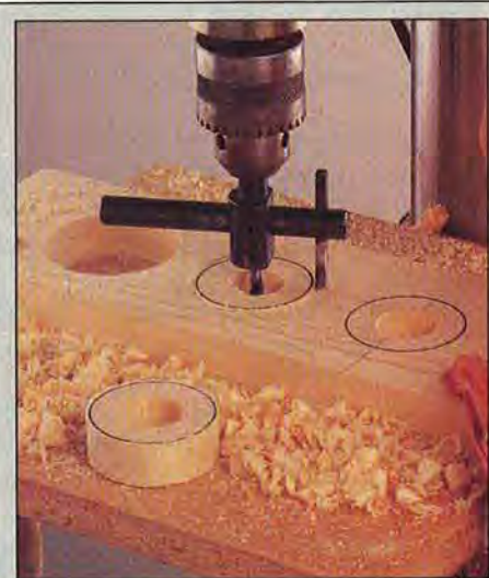
Center the circle-cutter pilot bit over the Forstner-bit depression, and cut the wheels to shape.
