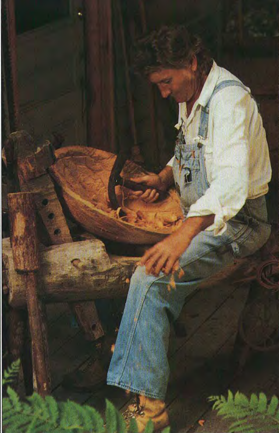
John likes to rough-shape his bowls at his cabin in the hollow. There's no telephone to interrupt him as he works the inside of the bowl with a hand adz.
