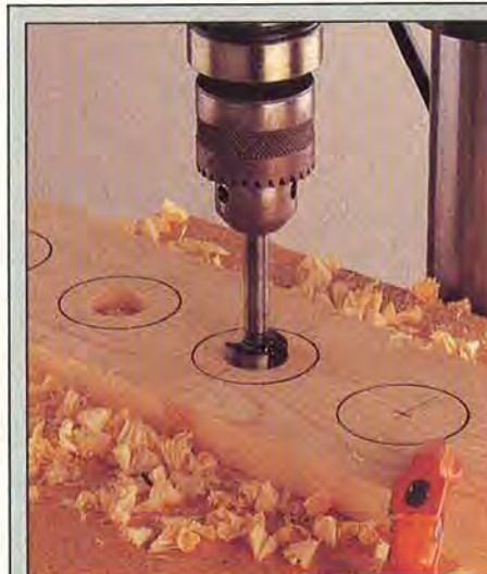
Mark the wheel centerpoint locations 3" apart on the pine, and drill holes \frac{1}{2} " deep for each wheel.
