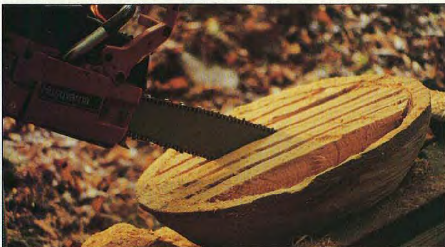
With a technique similar to cutting a mortise, the craftsman saws deep incisions, then clears them away. The bowl won't shift in the form-fitting saddle.
