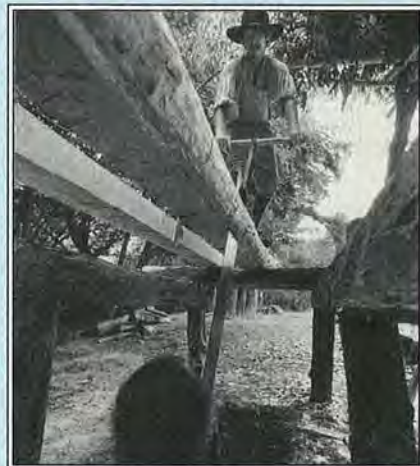
In colonial times, logs were ripped with a long, double-handled pit saw.
