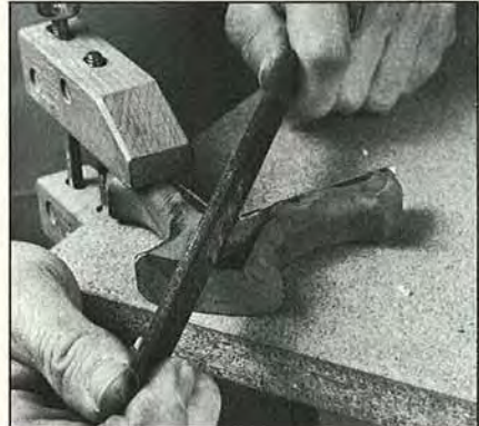
Use a bastard file to form a notch in the brass to match the groove cut in the walnut handle.
