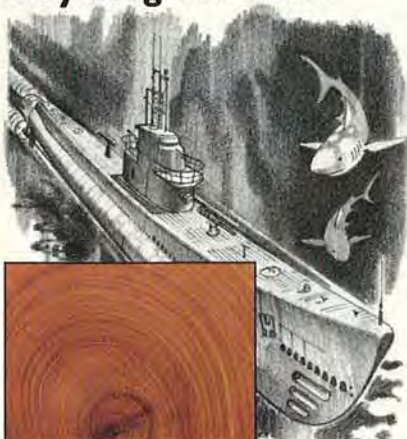
At home in water, lignum vitae helped submarines run quietly.
