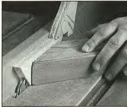
Cut a \frac{1}{4} " groove \frac{3}{4} " deep centered along the inside-curved edge of each lid piece. Use a push stick to feed the stock.
