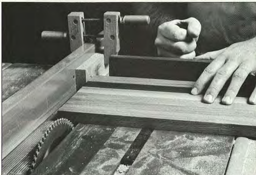
Clamp a scrap block to your rip fence for use as a stop to ensure equal-length pieces. The guard was removed for photo clarity.
