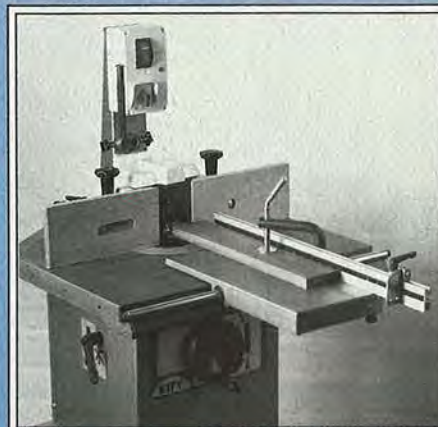
Kity's sliding table makes for safe cross-grain cuts. Jet and Sunhill also have sliding-table shapers under $2,000.
