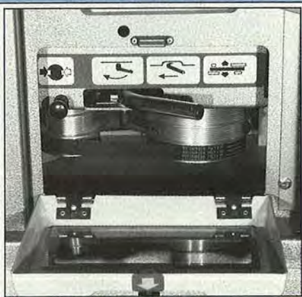
You can quickly switch between three speeds by means of a convenient handle on the Kity 623.
