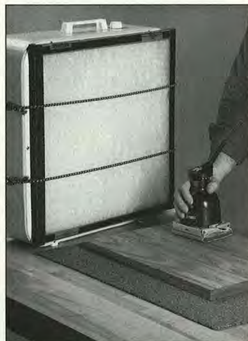
We strapped a furnace filter to a window fan with bungee cord for an inexpensive dust evacuator.
