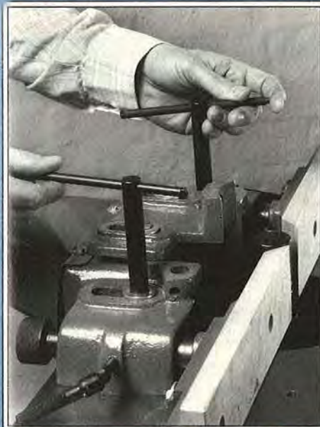
You can remove the fence on the Jet JWS-34-1 with a few turns of its convenient handles.
