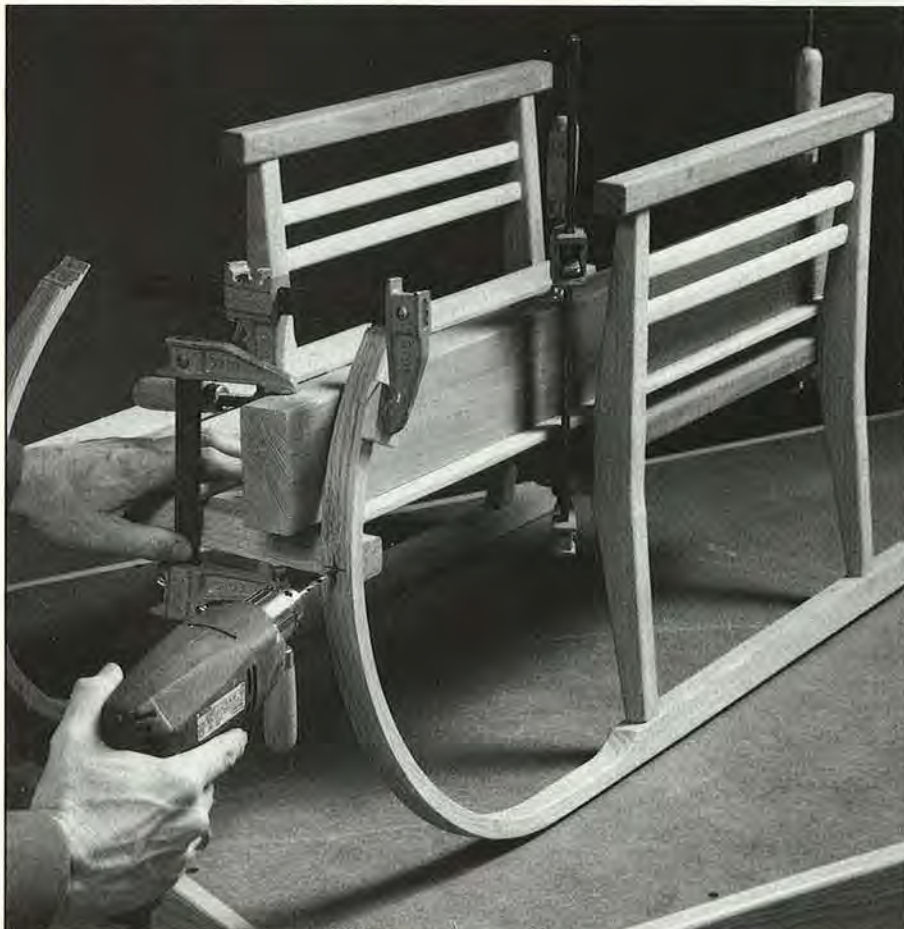
Mark the centerpoint and drill a hole for fastening the deck-board support to the laminated runner. The 2×4 helps keep the deck boards flat.
