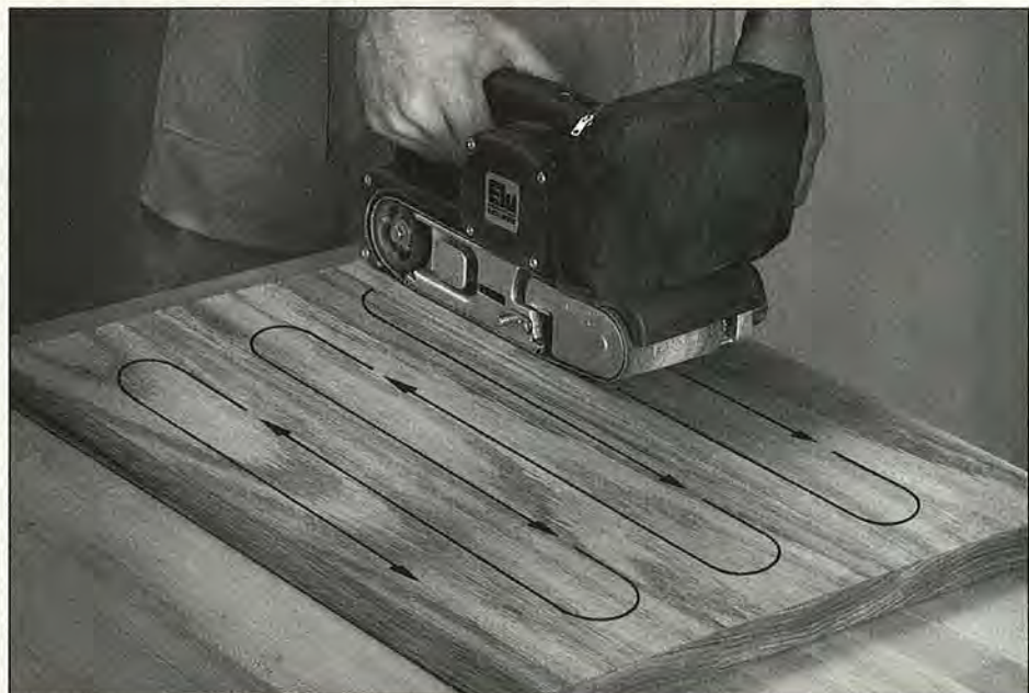
Try to minimize cross-grain movements when smoothing a surface with a belt sander. Sand the full length of the workpiece and keep the machine moving.
