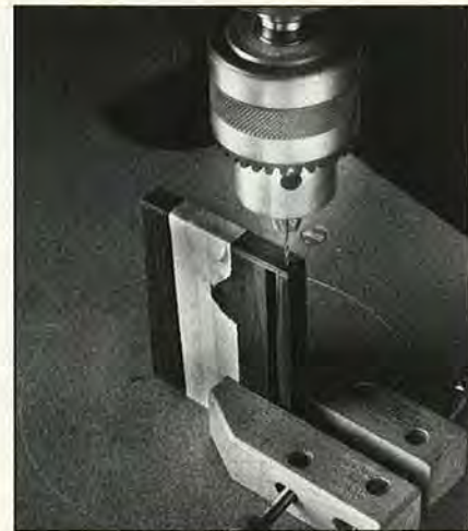
Mark the location of the hinge pins, tape the assemblies together with the edges and ends flush, and drill 1/16" holes.
