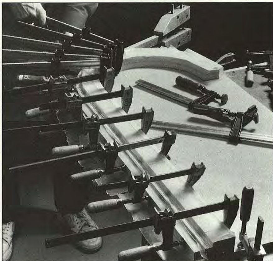
Starting at the straight end, clamp five \frac{1}{8} "-thick oak strips to the bending form to laminate the runner.
