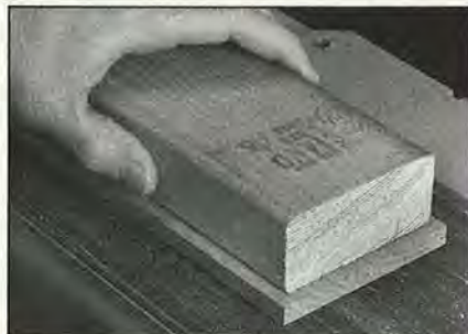
To smooth resawed stock, position it parallel to the sanding belt.
