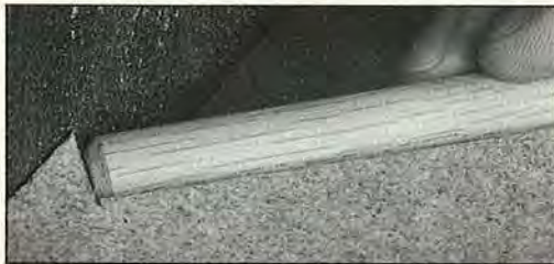
With the chamfering jig in place, spin the dowel until the chamfer is complete.
