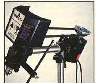
With Delta's radial press, above , you tilt the head, not the table. When working with long stock, this simplifies drilling holes at an angle.
