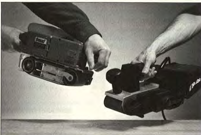
You need two hands with in-line sanders such as the Freud LC75,
