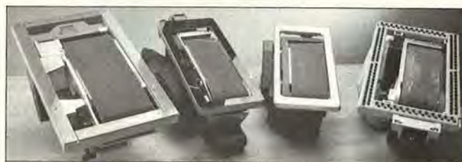
Sanding frames: From left, Hitachi and Ryobi (both plastic-on-aluminum bases), Skil (all steel), and AEG (brush bottom).
