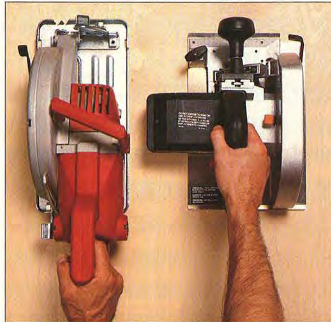
A worm-drive saw, such as Milwaukee's 8¼" model, left , extends your reach over a helical-gear saw such as AEG's 8¼".
