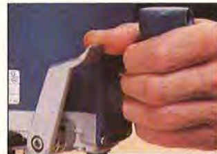
A spring-actuated lever automatically locks when you release your thumb. We found this one the easiest to use.
