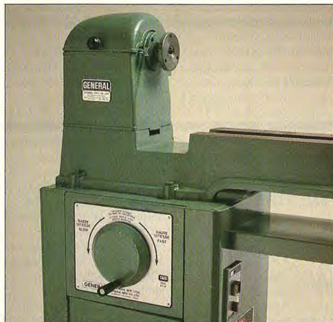
"Gap-bed" lathes such as the General shown in the photo, above , expand the diameter of faceplate projects the lathe can
