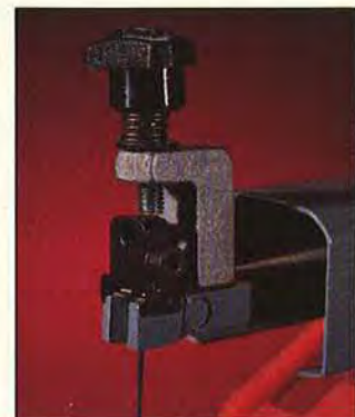
When using a clamp-type holder such as this one, make sure you leave a 1/16" gap between the locking screw and clamp to prevent breaking an excessive number of blades.
