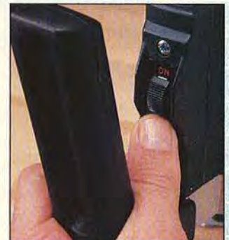
Slide switches can't be inadvertently tripped.
