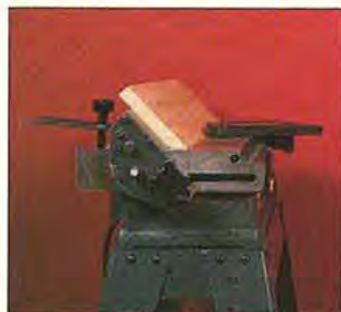
The Sears 23220 has a fence mounted on the end of its outfeed table—a drawback in our opinion.
