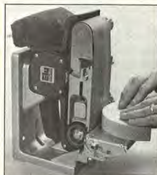
The Elu inversion stand enables you to shape small objects.
