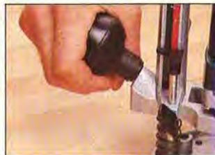
A twist knob (the right-hand handle) locks easily, but may loosen when you pick up the router.
