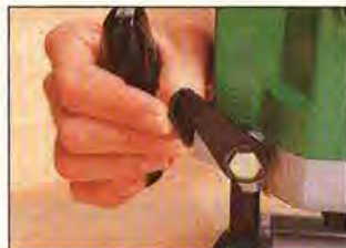
A manual locking lever requires the most effort to operate. Flip it down to lock, up to unlock. These can vibrate loose.
