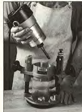
Porter-Cable's new plunge base retrofits to most 3½"-diameter motor housings.
