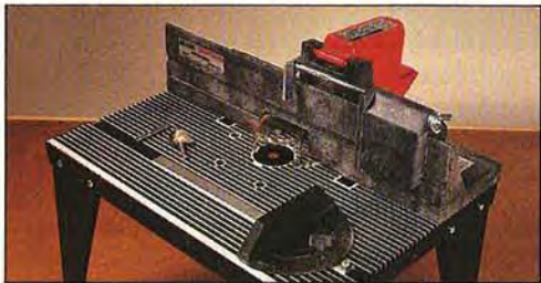
A router table provides a partial alternative to a stationary shaper, at a much lower cost.
