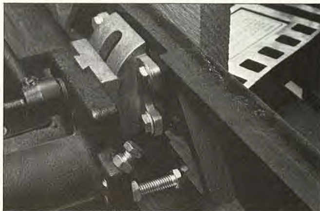
Two bolts serve as quickly adjustable 45° and 90° stops on
