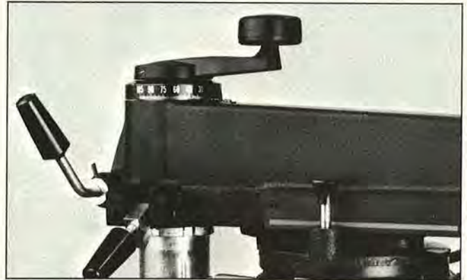
Column-mounted elevating crank and arm controls on the 12"
