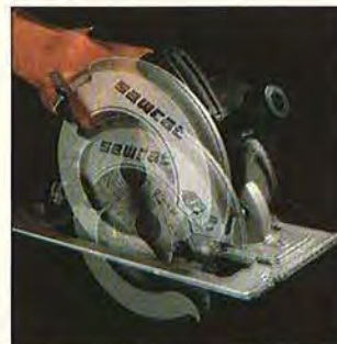
As you go from a full to light cut while using a rear-pivot portable circular saw, your hand position changes little. This proves to be a handling plus.
