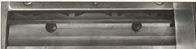
Grizzly, top, has three blade-lock bolts, no height-adjustment.
