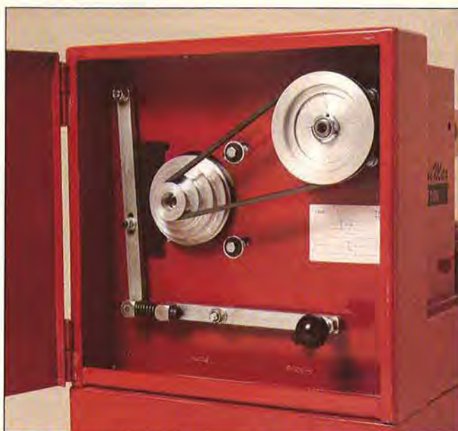
Mechanical speed-reduction systems increase horsepower at
