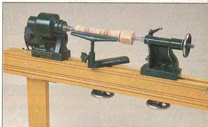
Conover's head and tailstocks mount on wood beams of any length.
