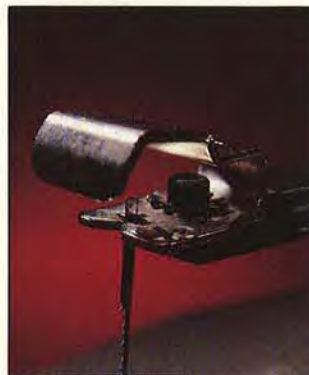
The AMT model 4601 has a pin-type blade holder, but you can install a pivoting blade clamping device that holds standard blades and comes with every unit.
