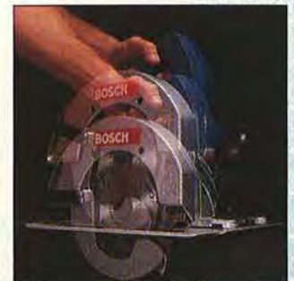
With a drop-foot saw, you can cut at various blade depths without changing your balance. The reason: The vertical alignment of your hand stays the same.
