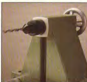
The tailstock's adjustable spindle should move in and out 2 or more inches for use with a drill chuck, as shown here.
