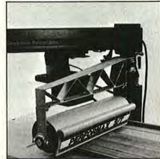
Performax's S/T drum sander attaches to a radial arm or to a stand the company offers.
