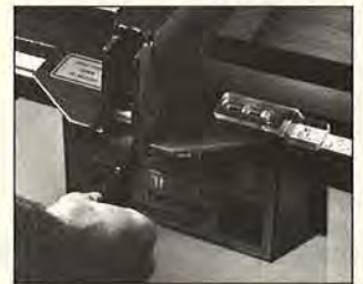
The fence on the Foley-Belsaw 4900900 is lighter duty than a Biesemeyer or Vega, but works just as accurately.
