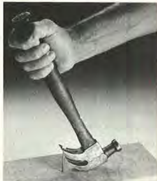
Voight's double-claw hammer was one of 400 hammers patented in the U.S. between 1840 and 1910.
