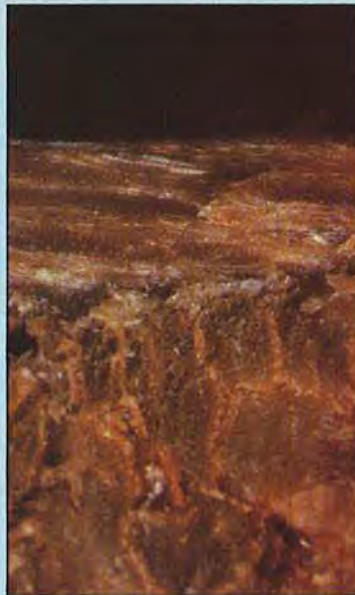
Taken at 8X magnification, the photo left shows Asian plywood's thin-as-a-coat-of-paint walnut face veneer. The dark substrate below the face veneer fools the eye by making the top layer appear thicker. In contrast, American-made plywood, right , has solid face veneer from \frac{1}{28} " to \frac{1}{32} " thick.
