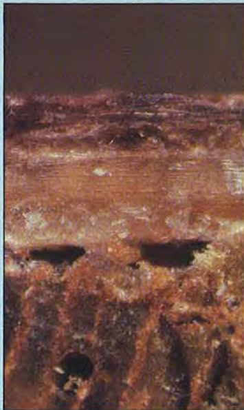
Taken at 8X magnification, the photo left shows Asian plywood's thin-as-a-coat-of-paint walnut face veneer. The dark substrate below the face veneer fools the eye by making the top layer appear thicker. In contrast, American-made plywood, right , has solid face veneer from \frac{1}{28} " to \frac{1}{32} " thick.
