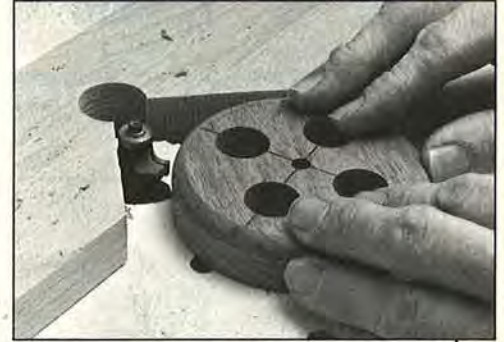
For safety, use a router with a V-shaped notch when routing the wheels.
